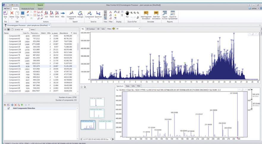
Mass Frontier software extracts the multiple components that can occur underneath chromatographic peaks. Each blue triangle is a detected component.
