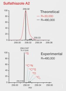
Full-scan mass spectrum of sulfathiazole, measured using the Orbitrap Exploris 480 mass spectrometer at a resolution (R) setting of 480,000 (FWHM) at *m/z* 200, demonstrates outstanding resolving power.
