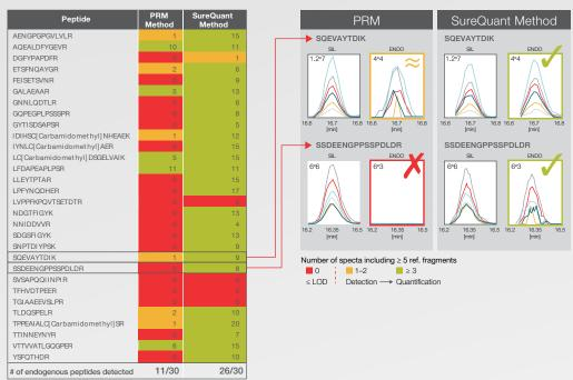
Compared to PRM methods, the SureQuant method increases resolution by a factor of four, and fill time by a factor of six, without compromising cycle time. The result is higher sensitivity and more reliable detection of targets, as shown here for peptides from the protein targets GSK3 $\alpha$  and AKTS1 from the AKT/mTOR pathway—a key cancer biology pathway.
