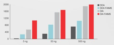
Combining the Orbitrap Exploris 480 mass spectrometer with the FAIMS Pro interface and a DIA strategy enables sensitive analysis for short gradients, high throughput (>200 samples per day), and identification of 2500 peptides per minute of gradient time. Overall, proteome coverage is increased by over 35% compared with data-dependent acquisition (DDA).
