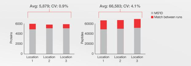
To asses instrument reproducibility, three operators at three different locations analyzed 1 µg of Thermo Scientific™ Pierce™ HeLa Protein Digest Standard (n=5). Left figure indicates the number of proteins identified at 1% false discovery rate (FDR) and the right figure shows the number of identified peptides for each of the three locations.
