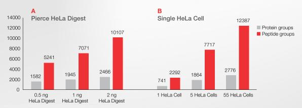
The Orbitrap Exploris 480 mass spectrometer with the FAIMS Pro interface provides sensitivity from low-ng to single-cell levels. (A) Instrument performance at low nanogram levels (0.5-2 ng Pierce HeLa Digest Protein Standard), (B) Instrument performance at single-cell levels (1, 5, and 55 HeLa cell).
