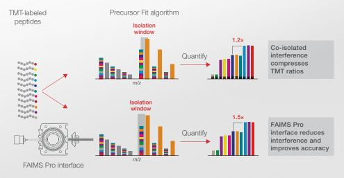
Thermo Scientific technology adds quantitative precision, accuracy, and throughput. The Precursor Fit algorithm increases precursor specificity in the isolation window, reducing co-isolated interferences.
