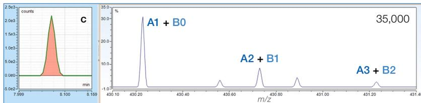
With a lower resolution setting of 35,000 (at  $m/z$  200) all three isotope peaks of the deamidated form (B0-B2) are overlapping with the isotopes of the wild type form (A1-A3).
