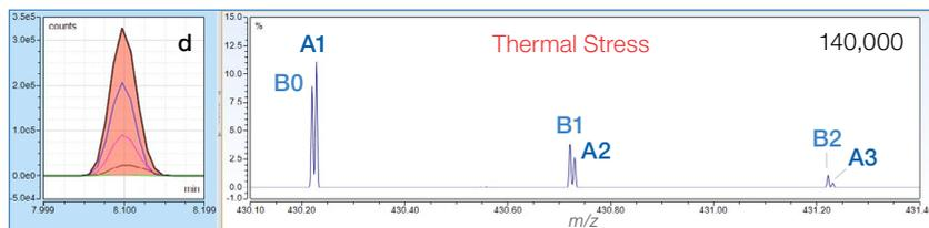
A resolution setting of 140,000 or higher (at  $m/z$  200) is needed to detect significant abundance increase of the deamidated form (B0-B2) in the thermally stressed sample.
