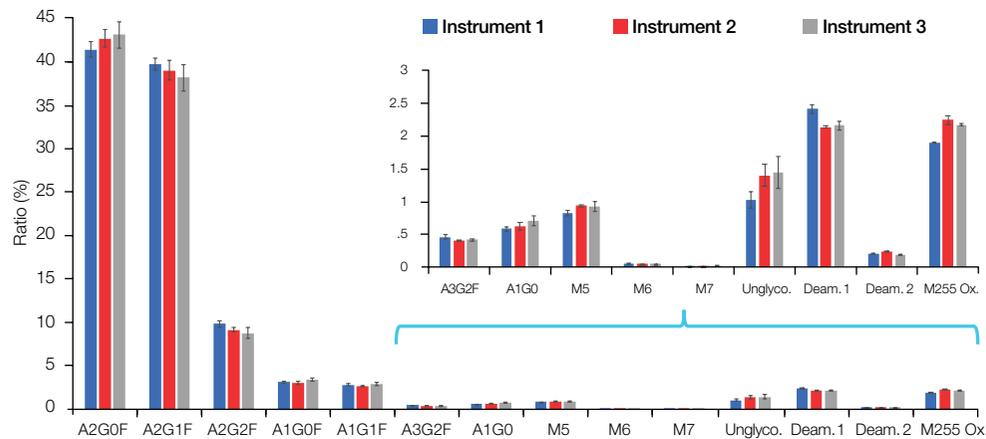
Consistent results for common CQAs on three different HR MAM instruments.
