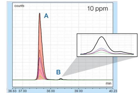
Extraction with 5 ppm mass tolerance—correct peak (peak B) was integrated in the absence of the wild type form (peak A).
