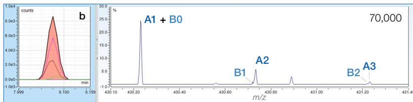
At a resolution setting of 70,000 (at  $m/z$  200) the monoisotopic peak of the deamidated form (B0) is completely overlapping with the C13 peak of the wild type form (A1), resulting in the absence of this isotope in peak integration.
