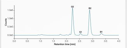
FLD chromatogram of the four aflatoxins: G2, G1, B2 and B1 at a concentration of  $0.9 \mu g/kg$  for G2 and B2 and 2.9  $\mu g/kg$  for G1 and B1.
