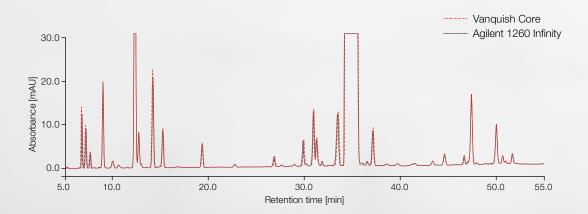
With the Vanquish Core HPLC system, the instrument gradient delay volume can be seamlessly adjusted in order to match legacy HPLC instruments. In this example the gradient delay volume was increased by a simple software command (Idle Volume=200  $\mu$ L) in the instrument method to best match the Agilent<sup>®</sup> 1260 Infinity LC system.
