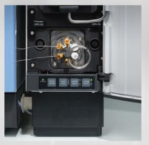
Method Transfer kit for Vanquish Core HPLC system. In combination with the Vanquish Split Samplers metering device, the gradient delay volume can be adjusted on a microliter scale over a wide range. Audit trail tracking of the settings and full qualification ensure regulatory compliance.
