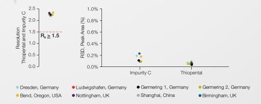
Above graph: Test sites of a Vanquish Core round robin test using eight different instruments with individual samples, users, and columns. Each analysis passed the specified SST criteria highlighting the reliability of the instrument and the ease of use for each user resulting in successful SST.
