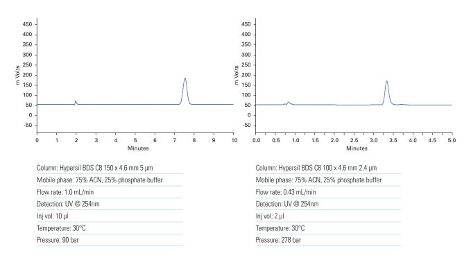
Figure 9: Columns packed with 2.4 µm particles give faster, more efficient chromatography than columns packed with 5 µm particles
