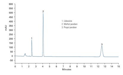
Column: Hypersil BDS C18 150 x 4.6 mm 5  $\mu$ m Mobile phase: 30% MeCN 70% 50 mM KH<sub>2</sub>PO<sub>4</sub> pH 3.5 Flow rate: 1.0 mL/min Detection: UV @ 254nm Inj vol: 20  $\mu$ l Temperature: 30°C Pressure: 92 bar
