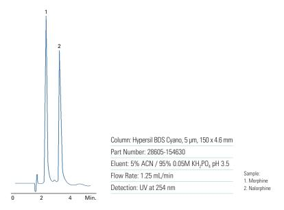
Figure 8: Polar compounds (morphine and nalorphine) are retained and separated using a Hypersil BDS Cyano column
