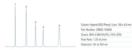
Figure 7: Analysis of procainamides using a Hypersil BDS Phenyl column
