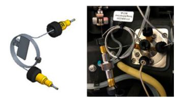
Figure 3. Schematic of the strong solvent loop on the left and installed on the instrument on the right
