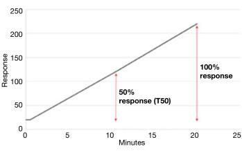
Figure 1. Experimental gradient delay volume calculation
