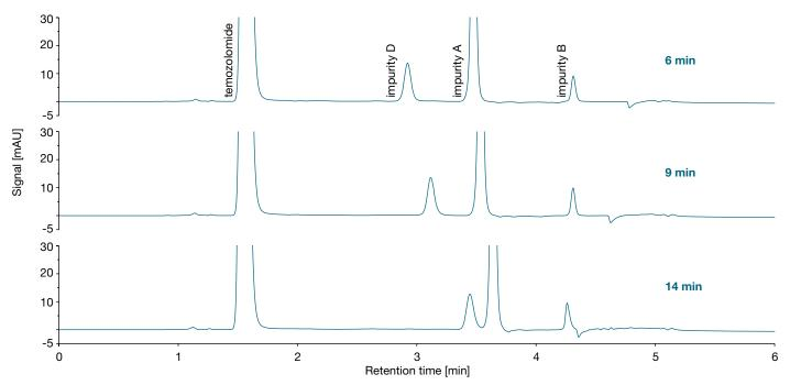
Figure 3. Selectivity changes of the HILIC method dependent on equilibration time (6, 9, and 14 min), shown for sample IV
