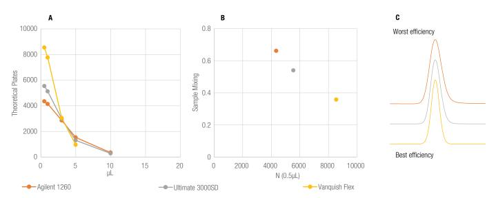
Figure 20. (A) Dependency of increasing injection volumes on system efficiency, (B) relationship between instrument sample mixing behavior and system efficiency with (C) respective peak shapes
