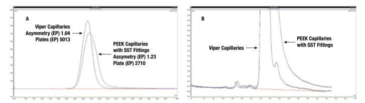
Figure 19. Comparison of Viper capillaries with ferrule-based fitting systems. (A) Asymmetry and plate counts of a single peak and (B) resolution of API and nearly eluting impurity
