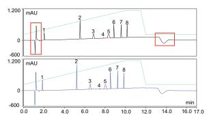
Figure 1. Gradient separation of heart disease treatment drugs performed on an Agilent 1100 system (black) and an UltiMate 3000 system (blue), both with default flow connections. The red rectangles indicate baseline artifacts caused by the injection and the final gradient step.
