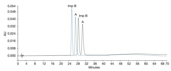
Figure 1. System suitability (Atorvastatin (A) and impurity B (Imp B)) standard solutions on an Agilent 1260 system (blue) and a Vanquish Flex UHPLC system (black)
