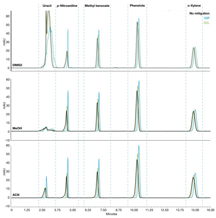
Figure 8. Overlay of chromatograms using the 4.6 mm ID column and 20 µL injection volume without any mitigation, with CIP and with SSL for all three sample solvents (ACN, MeOH, and DMSO)
