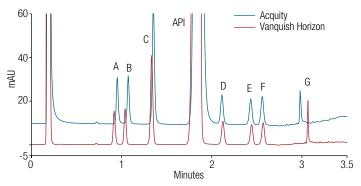
Figure 4. Chromatograms of down-scaled UHPLC method with Acquity and Vanquish Horizon systems; peak assignment according to impurity designation in EP monograph
