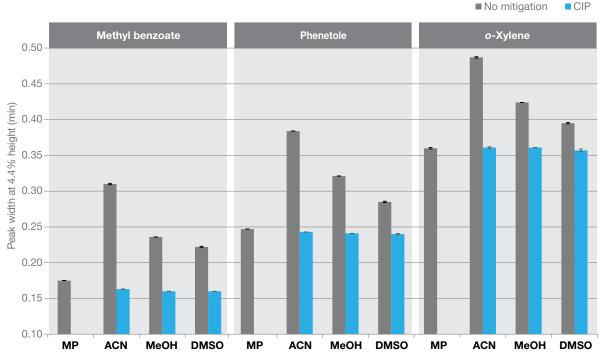
Figure 5. Peak width at 4.4% with 3 mm ID column and 10 µL injection volume with no mitigation and CIP for all sample solvents. Standard deviation is shown with the vertical error bars (N=3).
