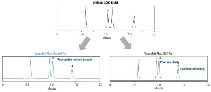
Figure 15. Influence of thermostatting mode on the transfer of a method
