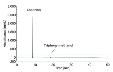
Figure 4. Injections of system suitability solution for impurity method for losartan potassium on a Vanquish Core (black) and an UltiMate 3000 (blue) HPLC system Table 12. System suitability requirements for losartan potassium analysis
