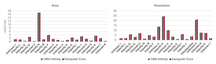
Figure 2. Chromatographic results with the 1260 Infinity and Vanquish Core HPLC systems under conditions outlined in the EP monograph (Figure 1)
