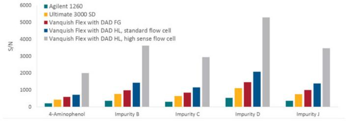
Figure 6. Signal-to-noise ratios (S/N) obtained with Agilent 1260 Infinity system, Ultimate 3000 SD system after method transfer optimization (750  $\mu$ L static mixer and gradient prestart), Vanquish Flex system after method transfer optimization (100  $\mu$ L sample loop and idle volume 68  $\mu$ L) with DAD FG, DAD HL with 10 mm flow cell, and DAD HL with 60 mm high sense flow cell. Noise calculated from the current chromatogram 4.1–4.6 min.
