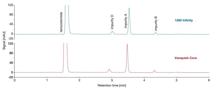
Figure 4. Transfer from 1260 Infinity system to Vanquish Core system
