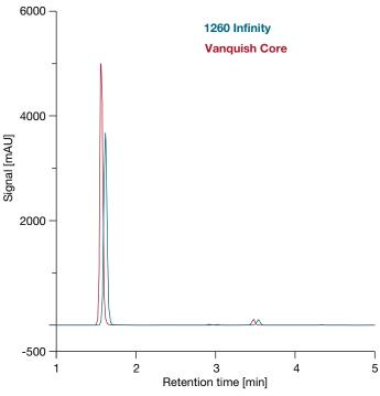
Figure 6. Unzoomed comparison of chromatograms obtained by 1260 Infinity and Vanquish Core instruments. While the temozolomide peak exceeds the linear range of both detectors, the dynamic response of the Vanquish Core VWD was distinctly higher than that of the 1260 Infinity VWD.
