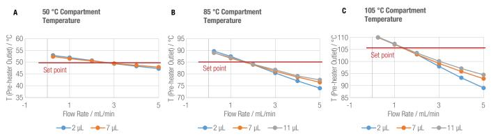
Figure 10. Passive eluent pre-heating effects on flow rate and pre-heater volume grouped by set compartment temperature
