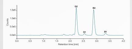
FLD chromatogram of the four aflatoxins: G2, G1, B2 and B1 at a concentration of 0.9  $\mu$ g/kg for G2 and B2 and 2.9  $\mu$ g/kg for G1 and B1.
