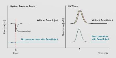
Significant reduction of pressure drop after sample injection using SmartInject Technology resulting in improved retention time reproducibility (6 replicates) and enhanced column lifetime.
