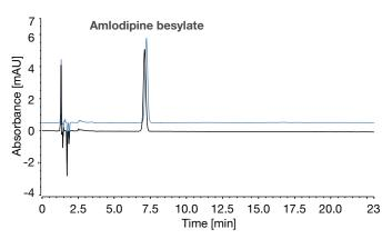
Figure 2. Injection of standard solution for related substances of amlodipine besylate on a Vanquish Core (black) and an UltiMate 3000 (blue) HPLC system
