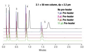
Figure 11. Standard isocratic column test on a column that produces small peak volumes show the effect of the pre-heater on peak shape and retention. Stationary phase: Thermo Scientific<sup>™</sup> Acclaim<sup>™</sup> RSLC 120 C18, eluent: water/acetonitrile 60/40 v/v, flow rate: 1.0 mL/min, column temperature: 70 °C. Peak assignment: 1: Uracil, 2: Nitroaniline, 3: Methylbenzoate, 4: Phenetole, 5: o-Xylene.
