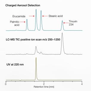
Unlike mass spectrometry (A) and UV (B), the CAD can measure all analytes in a sample. Mass spectrometry (MS) requires the analyte to form gas phase ions while response by a UV detector depends upon the nature of the chromophore.
