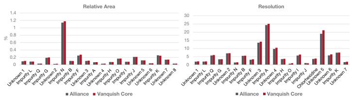
Figure 2. Chromatographic results with Alliance and Vanquish Core HPLC systems under conditions outlined in the EP monograph (Figure 1)
