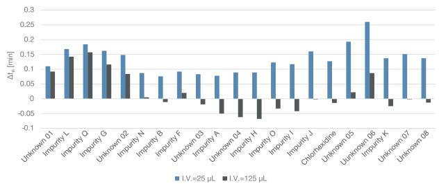
Figure 5. Retention time deviations of the Nexera-i system compared to the Vanquish Core HPLC system with an idle volume (I.V.) of 25  $\mu$ L (default) and of 125  $\mu$ L
