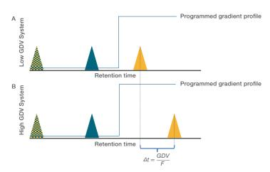
Figure 7. Impact of GDV on elution times of non-retained (blue) and strongly retained (orange) peaks during a step gradient elution (A) for a system with low GDV and (B) for a system with GDV. The retention time of the blue peak is not influenced by the GDV while the orange peak is directly shifted by the delay of the gradient (with GDV= gradient delay volume [mL], F=flow [mL/min] and  $\Delta t$ =retention time shift [min]).
