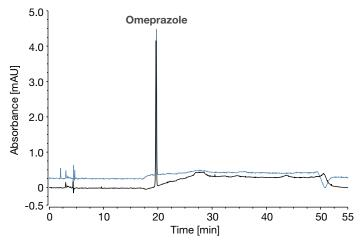
Figure 14. Injections of standard solution for the impurity method of omeprazole on a Vanquish Core (black) and an UltiMate 3000 (blue) HPLC system
