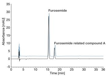
Figure 10. Injections of system suitability solution for furosemide assay on a Vanquish Core (black) and an UltiMate 3000 (blue) HPLC system
