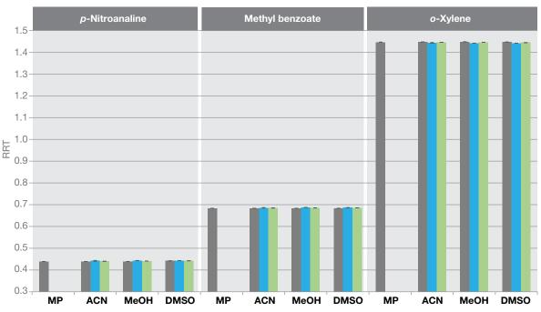
Figure 11. Retention time relative to phenetole (RRT) with the 4.6 mm ID column and 20 µL injection volume with no mitigation, CIP and SSL for all sample solvents. Standard deviation is shown with the vertical error bars (N=3).
