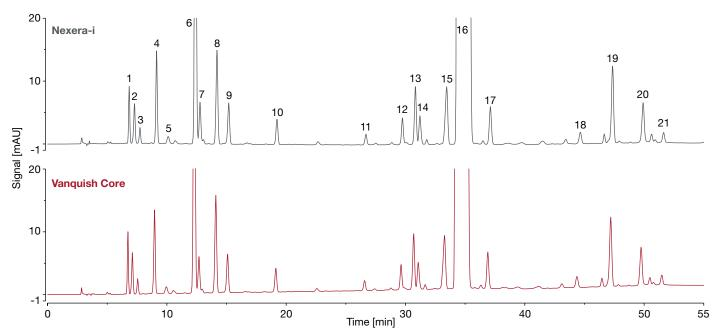
Figure 1. Transfer from Nexera-i system to Vanquish Core HPLC system according to the EP monograph for chlorhexidine gluconate; peak assignment according to impurity designation in EP monograph and standard leaflet<sup>5, 9</sup>
