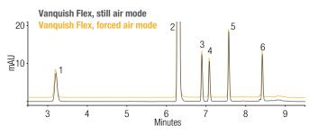
Figure 4. Negligible effect of column thermostatting mode for Vanquish Flex system in still and forced air mode. For peak assignment see Table 2.
