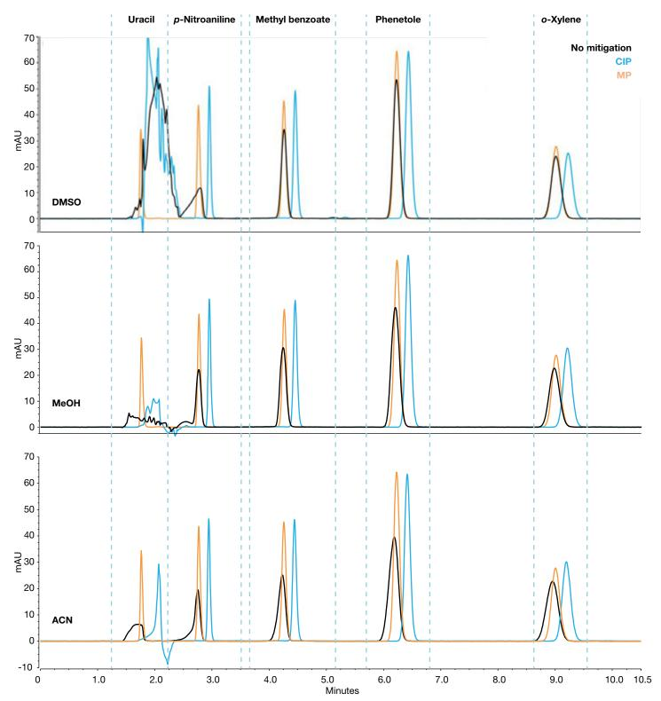
Figure 4. Overlay of chromatograms using the 3 mm ID column and 10  $\mu$ L injection without any mitigation ("no mitigation" and sample dissolved in mobile phase (MP)) and with CIP for ACN, MeOH, and DMSO. The sample in MP is shown as a reference.
