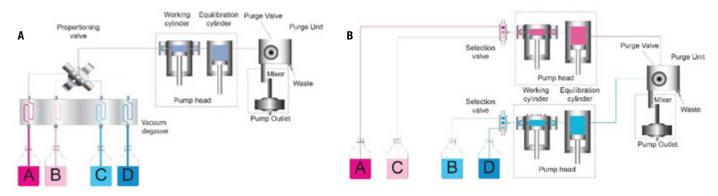
Figure 4. Schematic setup of a low-pressure gradient pump (A) and a high-pressure gradient pump (B). Note how the different solvent convergence points have effects on the gradient delay volume, which is defined as the volume between the convergent point of the solvents and the column head.
