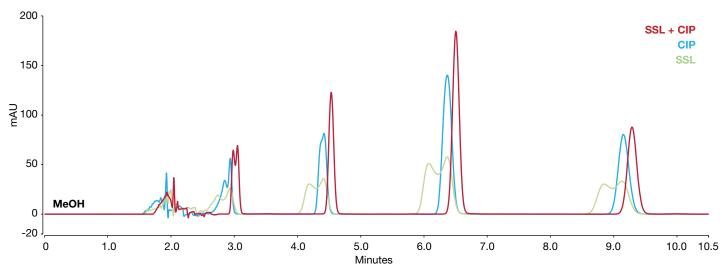
Figure 12. Overlay of chromatograms with SSL, CIP, and SSL+CIP using MeOH as a strong solvent for column 3 mm I.D and 30 µL injection
