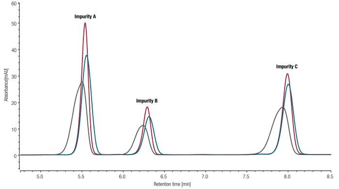
**Figure 3.** Overlaid chromatograms of normal injection (gray), custom injection A (blue), and custom injection B (red) of the impurities A–C. Sample: 1 mg/mL mebendazole SST in DMF; separation on a Hypersil GOLD column with 100 x 4.6 mm and 3 µm particle size; injection volume: 10 µL. For full details on the chromatographic method refer to Table 1; for full details on the custom injection programs refer to Table 2 and Table 3.
