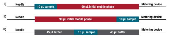
**Figure 2. Schematic drawing of the sample loop on the three different injection methods.** I = normal injection, II = custom injection A, III = custom injection B; sample = 1 mg/mL mebendazole SST standard in DMF; initial mobile phase = 20:80 acetonitrile:7.5 g/L ammonium acetate in water; buffer = 7.5 g/L ammonium acetate in water (refer to Tables 1–3 for more details)
