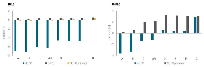
Figure 8. Summary of  $t_R$  deviations obtained with the Vanquish Horizon system at different column thermostatting settings with respect to the Acquity system set to 40 °C
