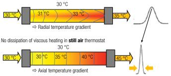
Figure 14. Schematic to show the differences in frictional heat dissipation for forced (top) and still air (bottom). For forced air, a radial temperature gradient occurs while for still air an axial temperature gradient occurs. The given temperatures are not real experimental data but simply serve to illustrate the effects.
