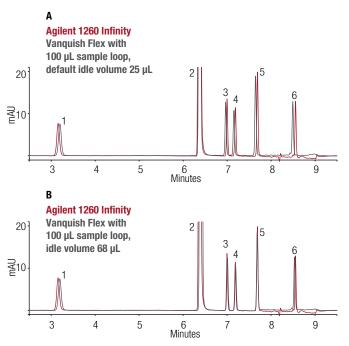
Figure 3. Method transfer from the Agilent 1260 Infinity system to the Vanquish Flex system. A) Comparison of Agilent 1260 Infinity system and Vanquish Flex system with 100  $\mu$ L sample loop; B) final transfer: comparison of Agilent 1260 Infinity system and Vanquish Flex system with 100  $\mu$ L sample loop and adapted idle volume to 68  $\mu$ L. For peak assignment see Table 2.
