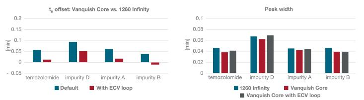
Figure 8. Effect of added ECV on the method transfer from the 1260 Infinity to the Vanquish Core system regarding t<sub>R</sub> offset and peak widths (at half height)
