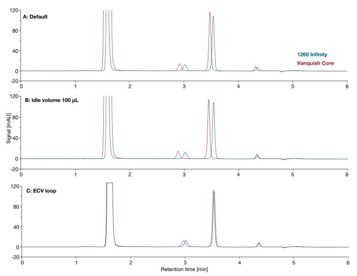
Figure 7. Overlay of chromatograms obtained by the 1260 Infinity instrument and the Vanquish Core instrument A) in default state (idle volume 25  $\mu$ L); B) with idle volume set to 100  $\mu$ L; C) with added ECV by 46  $\mu$ L loop installed between injector and column. While the GDV adjustment could not compensate the t<sub>p</sub> offset due to the partial column equilibration, the volume loop resulted in a closer match of ECVs.
