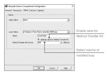
Figure 5. Instrument configuration screen of Chromeleon 7.3 CDS allowing the configuration of the method transfer kit and defining the loop volume thereof.  $200 \ \mu$ L is the volume of the loop provided with the method transfer kit, other volumes for customized loops can also be entered.
