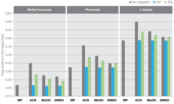
Figure 9. Peak width at 4.4% with the 4.6 mm ID column and 20  $\mu$ L injection volume with no mitigation, CIP and SSL for all sample solvents. Standard deviation is shown with the vertical error bars (N=3).
