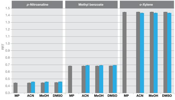
Figure 7. Retention time relative to phenetole (RRT) with 3 mm ID column and 10 µL injection volume with no mitigation and CIP for all sample solvents. Standard deviation is shown with the vertical error bars (N=3).
