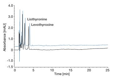
Figure 6. Injections of standard solution for the organic impurities procedure 1 of levothyroxine on a Vanquish Core (black) and an UltiMate 3000 (blue) HPLC system
