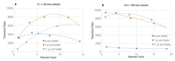
Figure 13. Plot of plate number against retention factor for both column type and experiment with no pre-heater, 1  $\mu$ L pre-heater, and 11  $\mu$ L pre-heater
