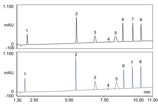
Figure 2. Gradient separation of heart disease treatment drugs performed on an Agilent 1100 system (black) and an UltiMate 3000 system (blue) with 800 µL mixer. The retention times obtained with both instruments match very well.
