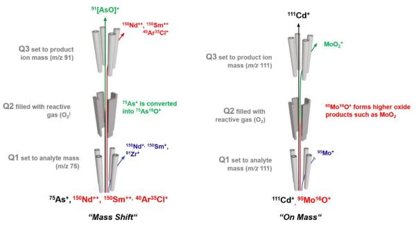
Figure 1. Possible reaction pathways in triple quadrupole ICP-MS
