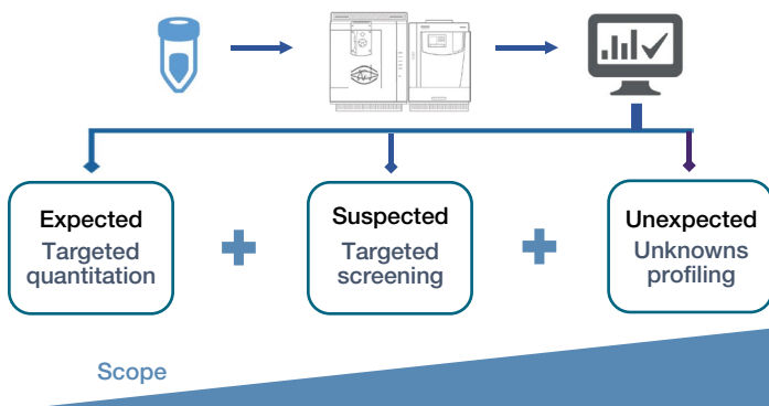
Figure 1. Analytical approaches to increase scope of analysis through full scan high-resolution, accurate-mass data
