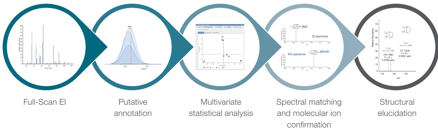
**Figure 1. Metabolomics workflow using the Orbitrap Exploris GC 240 MS and Compound Discoverer software, taking high quality data through to confident metabolite identification and confirmation**
