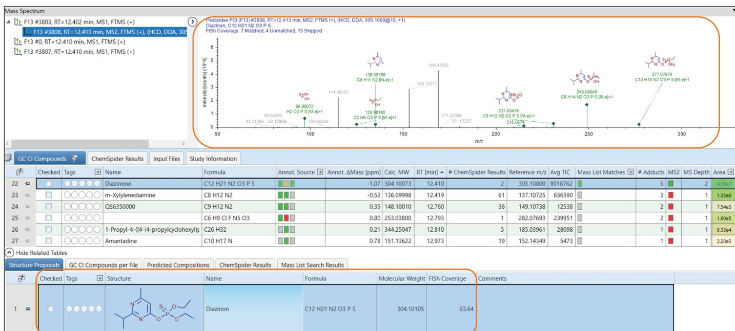
**Figure 8. GC CI results.** FISh Scoring for MS<sup>2</sup> scan. Identification through online database matching is performed and fragments assigned and annotated to mass spectrum.
