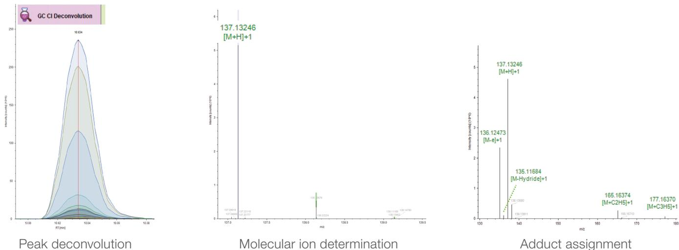
**Figure 5. Chemical ionization node functionality with the aim of identifying molecular ion adducts to support unknown identification or compound confirmation from spectral match result.** Peak deconvolution is followed by automatic assignment of molecular ion adducts (center and right).
