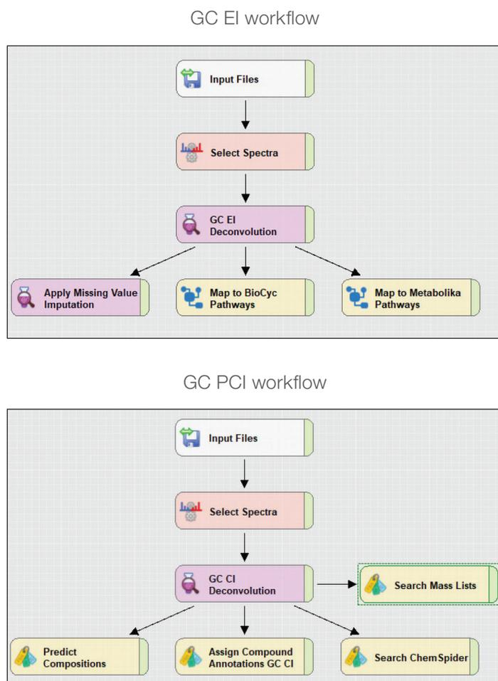
**Figure 2A. GC workflows in Compound Discoverer software, covering both EI and PCI HRAM data**
