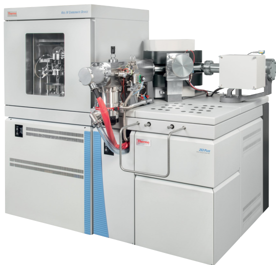
Figure 1. Kiel IV Carbonate Device (left) coupled to a 253 Plus 10 kV IRMS (right).
