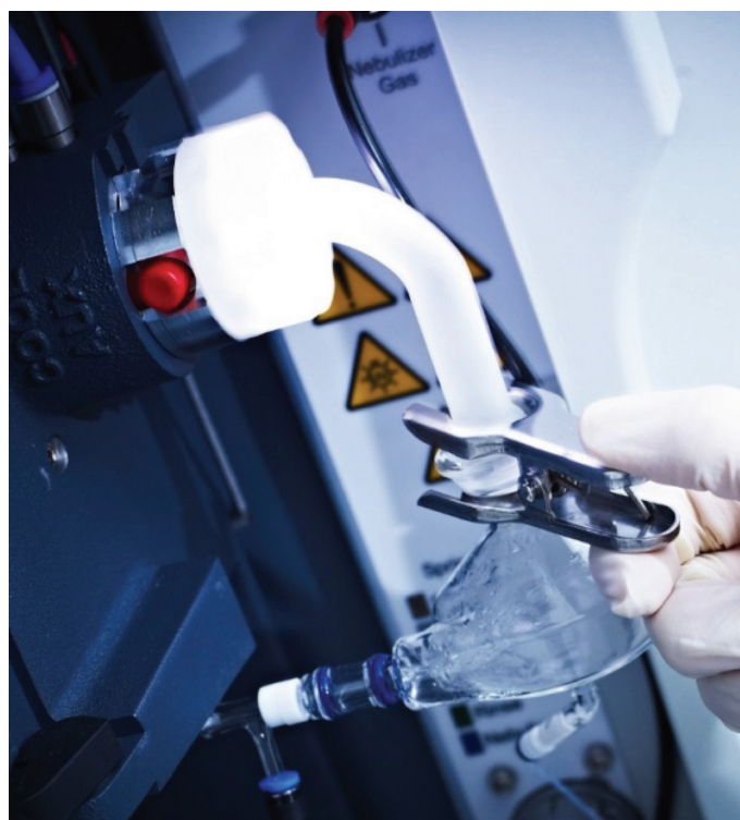
Figure 1. Standard sample introduction kits for the Thermo™ Scientific™ iCAP™ 7000 Plus Series ICP-OES Duo, designed for the analysis of aqueous solutions containing up to 3% TDS.
