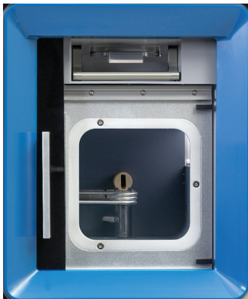
Figure 2. The iCAP PRO Series ICP-OES Radial torch box
