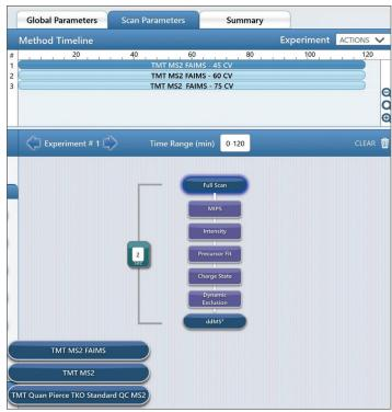
Figure 3. Within the ICSW method editor, application nodes for small-molecule or peptide analysis display pre-built, optimized method templates that are customizable through drag-and-drop method creation. Shown here is the pre-built method template for TMT multiplexing with the Thermo Scientific™ FAIMS Pro™ interface using three compensation voltages (CV), (-45, -60, and -75).
