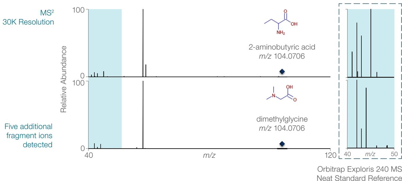
Figure 5. Extended low  $m/z$  range enables confident identification of isomers. Additional fragment ions are detected, and thus structural information, generated from this  $m/z$  range extension. In the case of 2-aminobutyric acid and dimethylglycine, there are 5 additional fragment ions detected that allow the confident differentiation of these 2 isomers.
