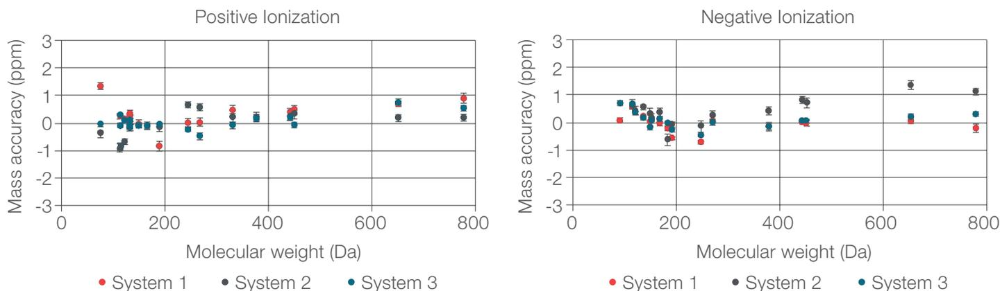
**Figure 2. The Orbitrap Exploris 240 MS delivers unsurpassed mass accuracy for all small molecules.** A mixture of 25 neat standards ranging in molecular weight from 75 Da to 777 Da, was analyzed repeatedly across 5 days. All standards were measured with excellent mass accuracy, often <1 ppm for the entirety of the experiment. The EASY-IC source was enabled during these measurements.
