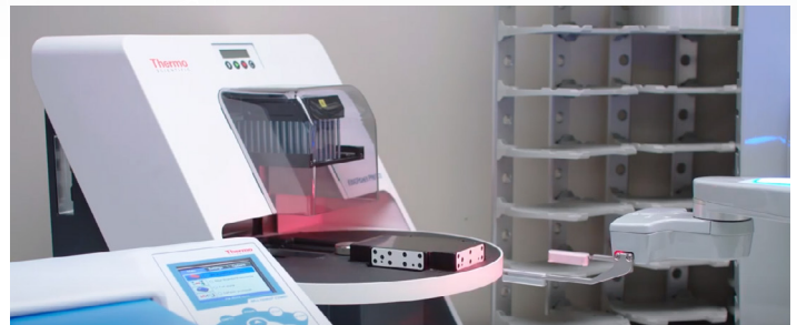
Figure 4. The Spinnaker robot performing vision teaching using the smart jig.
