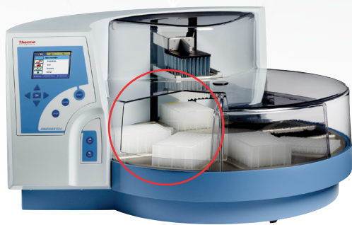
Figure 2. The Thermo Scientific™ KingFisher™ Flex System shows the appropriate clearance space for the gripper fingers of the robotic mover to access the plate inside the instrument.
