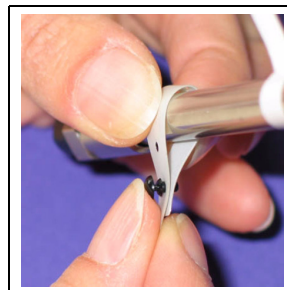
Figure 9-43. Attaching the Column ID System to the Column
