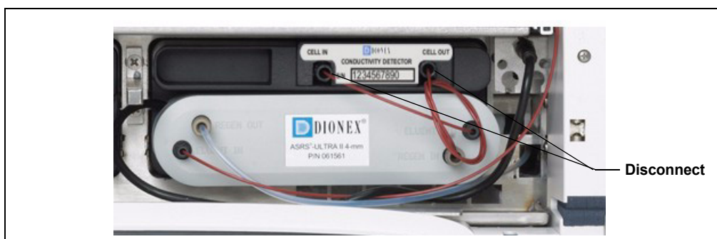
Figure 9-31. Disconnecting the Conductivity Detector Liquid Lines
