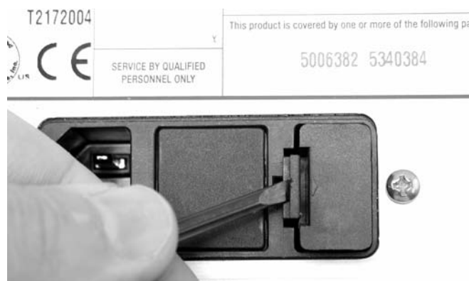
Figure 74. Using a screwdriver to pry off the fuse holder
