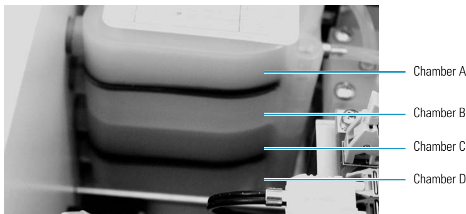
Figure 3. Vacuum degasser chambers behind the front panel
