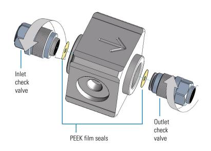
Figure 74. Installing the PEEK film seals and discontinued check valves
