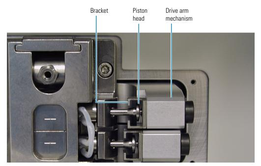
4. Insert the two piston retaining clips between the piston heads and the brackets of the drive mechanism arms.
