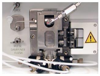
White, insulated, electrical wires connect the actuating coils at the ends of the proportioning valves to the pump as shown below. Take care not to pinch these wires when you remove the liquid displacement assembly (LDA) from the front panel of the pump to perform maintenance.
