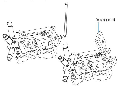
2. Remove the inner components of the LDA body. These components include the outlet module, the upper displacement chamber, and the lower displacement chamber with check valves.
