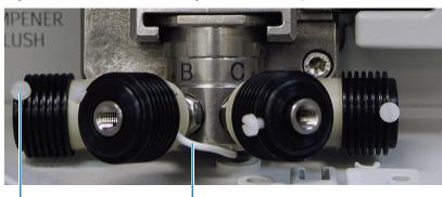
Figure 40. View of the actuating coils with their nylon screws
