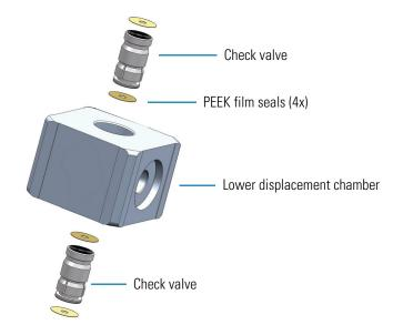
3. Because the fit between the check valve and the displacement chamber bores is loose, place the LDA body on a flat service as you insert the lower displacement chamber and check valve assembly.
