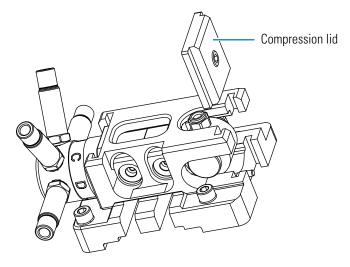
5. Using a 4 mm L-hex wrench, tighten the compression lid as shown in Figure 78.
