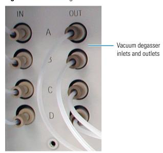
Figure 16. Vacuum degas connections
