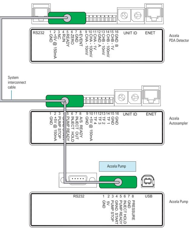
Figure 9. Schematic of the connections for the system interconnect cable
