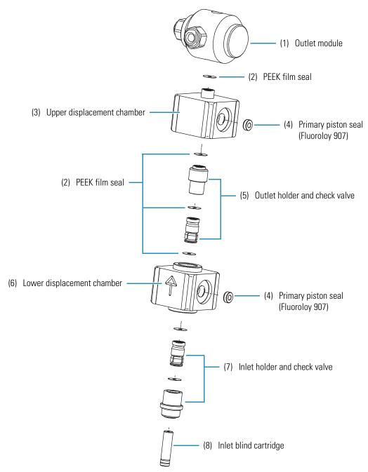
Figure 70. Liquid displacement assembly (current version, parts 1 to 8)
