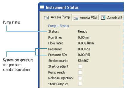
Figure 33. Pump Status area of the Accela Pump page (ChromQuest)
