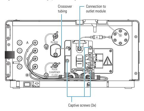
Figure 39. View of the high-pressure tubing connections
