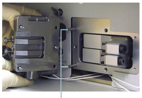
Figure 63. View of the alignment pins for the LDA body
