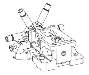
2. Slide the pistons as far as possible into the displacement chambers (see Figure 60).
