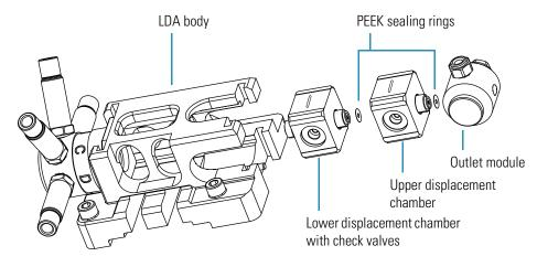
Figure 56. Installing the stacked components of the LDA
