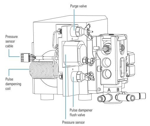
The pulse dampening assembly consists of a low volume T-connector that the mobile phase passes through. Attached to the side leg of the T-connector is a 2 mL loop of stainless steel tubing.
