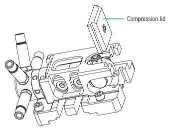
5. Using a 4 mm L-hex wrench, tighten the compression lid as shown in Figure 58.
