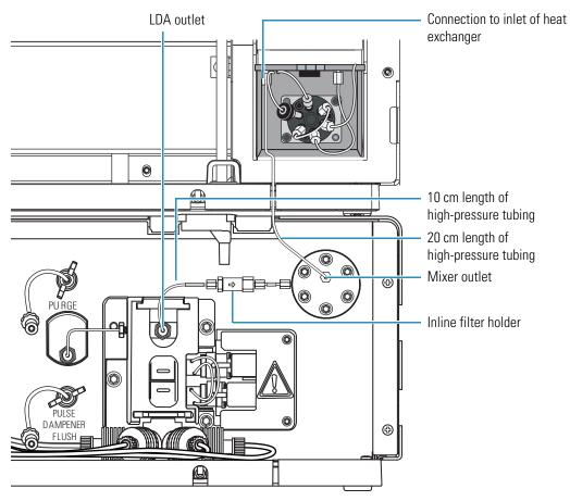
Figure 18. Connection between the pump and the autosampler
