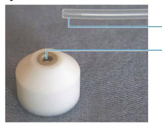
Figure 67. Solvent reservoir filter and solvent line
