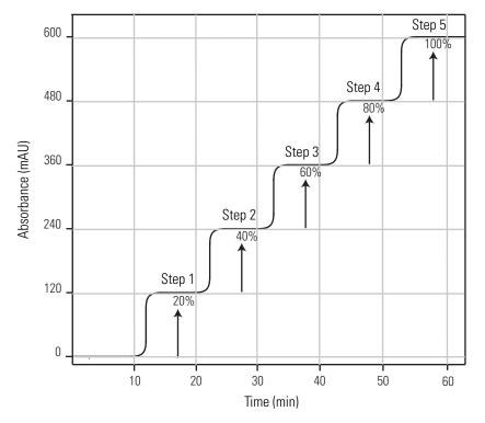
Figure 34. Step gradient profile for testing compositional accuracy
