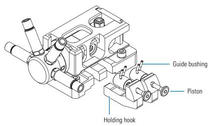
**Figure 47.** Removing the holding hooks, bushings, and pistons from the LDA body
