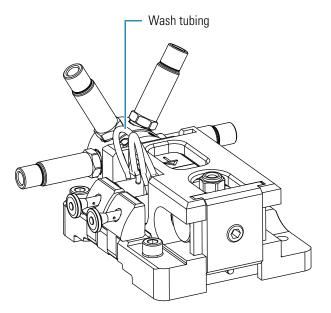
Figure 62. View of the LDA with the wash tubing installed on the guide bushings
