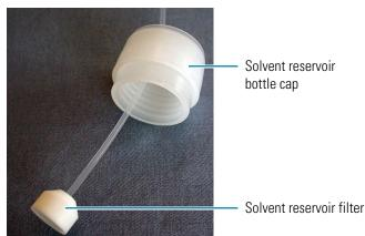
Figure 10. Solvent reservoir cap assembly
