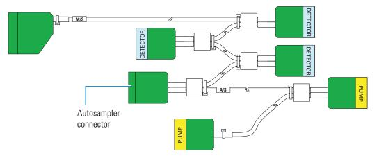
Figure 8. System interconnect cable with seven combicon connectors
