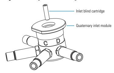
2. Slide the top rim of the quaternary inlet module into the bracket on the bottom of the LDA body (see Figure 54).
