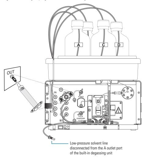
Figure 29. Using a syringe to draw solvent through a solvent reservoir line
