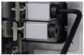
9. Remove the two piston spring clamps as shown Figure 43.
