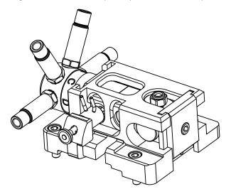
3. Using a 4 mm L-hex wrench, tighten the fastening screws (see Figure 61).
