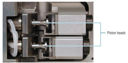
Figure 44. View of the piston heads pushed to the left
