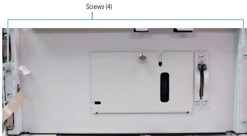
10. Slide the chassis out of the housing until the metal lamp compartment cover is accessible from the right side of the instrument.
