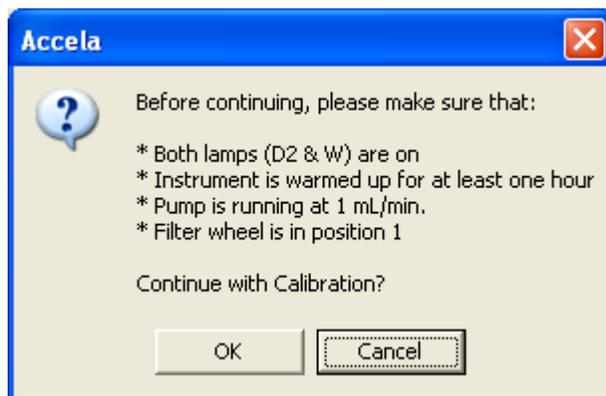
5. Make sure that the lamps are warmed up, that the pump is running at 1 mL/min, and that the filter wheel is in position 1 (see Figure 20 on page 25), and then click **OK**.
