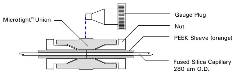
FIGURE 2-5 High Pressure Connection using a Microtight union.
