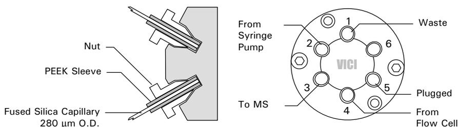
FIGURE 2-6 Connecting the Micro Valve
