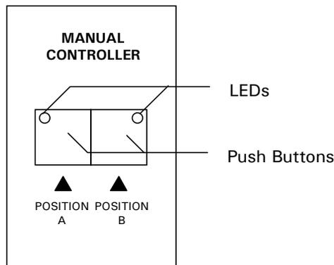
FIGURE 3-1 The Manual Controller
