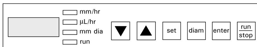
FIGURE 3-4 The Keypad of the Syringe Pump
