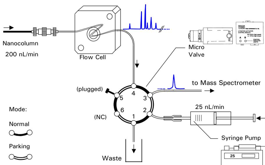
FIGURE 1-1. Schematic Diagram of the Peak Parking Setup
