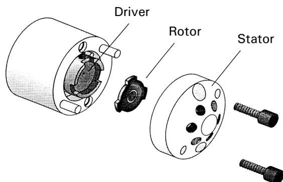
FIGURE 4-1. Exploded View of the Valco Model C2 Valve
