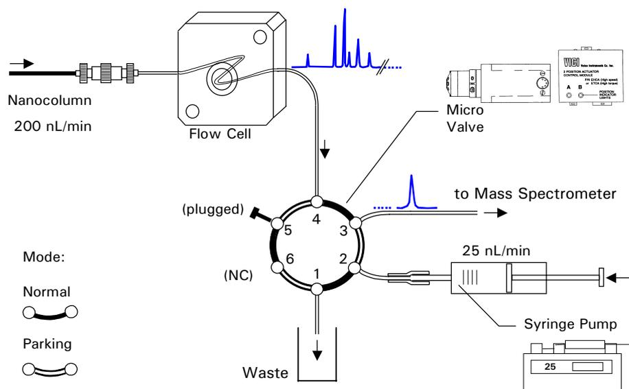
FIGURE 2-2 Fluidic Diagram with Peak Parking Kit
