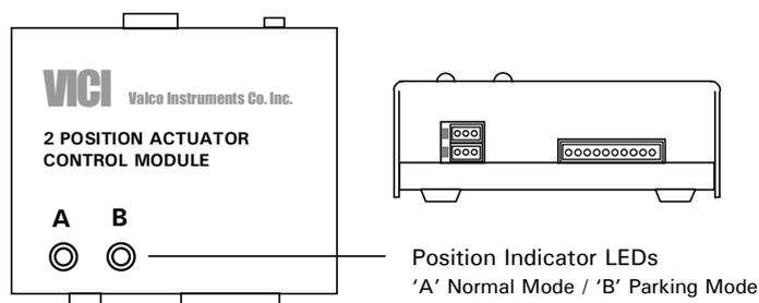
FIGURE 3-2 The Control Module
