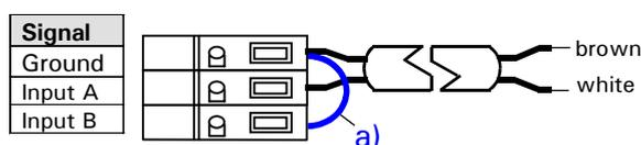
FIGURE 2-1 The MS Connector with the two Inputs – Default Configuration
