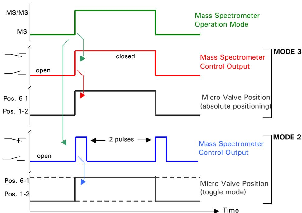
FIGURE 2-2 Input Mode 2 vs. Mode 3
