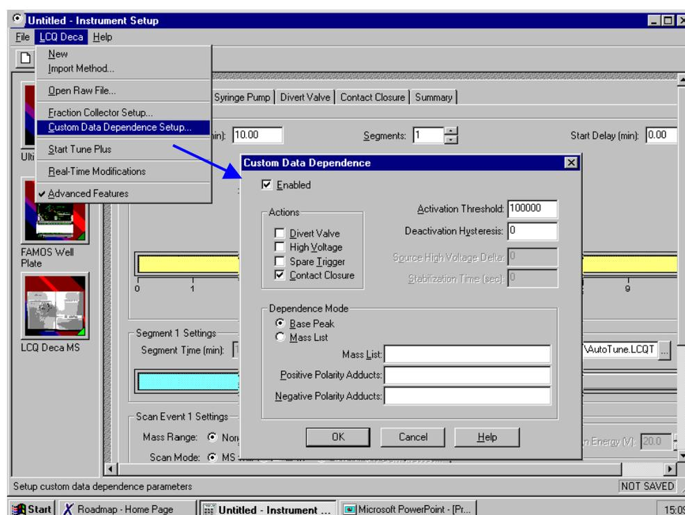
FIGURE 2-8 Xcalibur™ Instrument Method Setup for Generating the Control Signal
