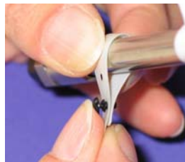
Figure 3-21. Attaching the Column ID System to the Column
