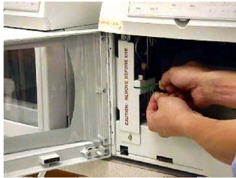
Figure 2-14. Shipping bracket hooked into frame and attached to sample arm and chassis with screws
