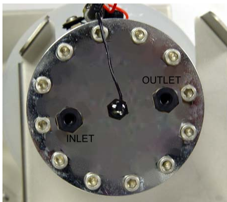
Figure 3-74. EGC Inlet and Outlet Fittings with Plugs
