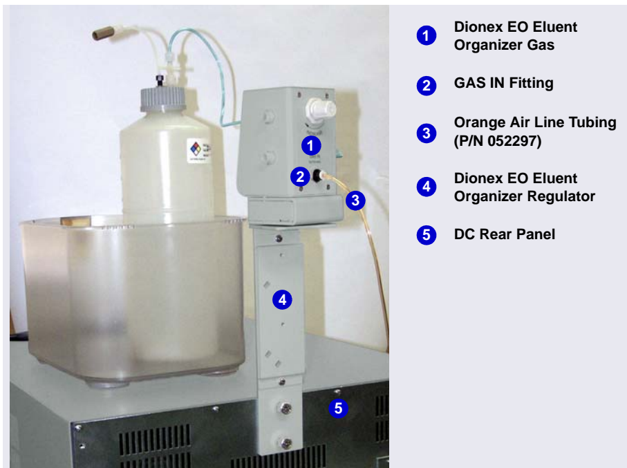
Figure A-2. Dionex EO Eluent Organizer Gas Regulator Connections
