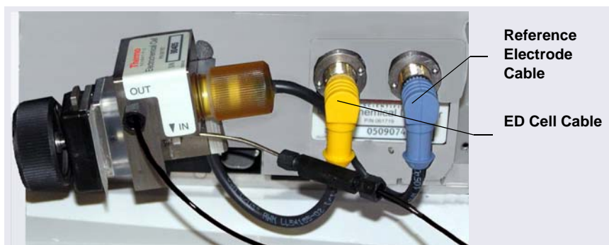
Figure B-14. ED Cell Installed on ED
