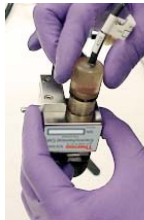
Figure B-12. Installing the pH-Ag/AgCl Reference Electrode In the Reference Electrode Well
