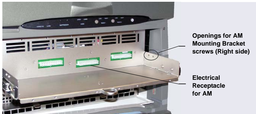
Figure B-24. DC with Top Component Tray Pulled Forward
