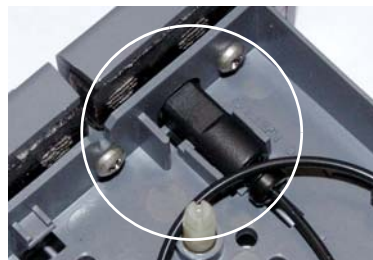
Figure 3-62. Column Outlet Fitting Installed in Column Cartridge
