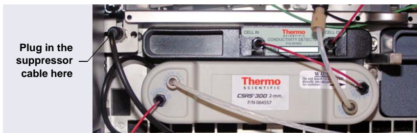
Figure 3-16. Installing the Suppressor (Left-Side Installation)
