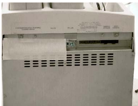
Figure 2-8. 5 cm (2 in) wide masking tape securing tubing within recess at rear of AS
