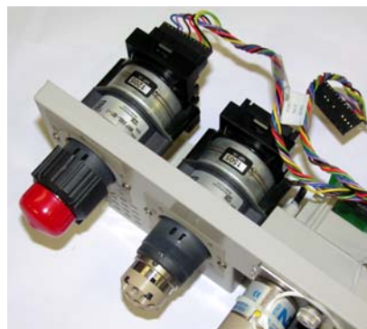
Figure B-21. High-Pressure Valve Installation
