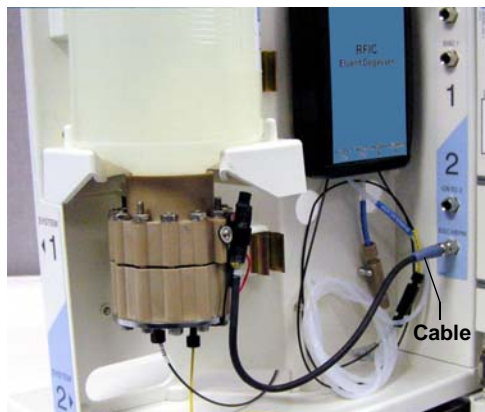
Figure 3-76. Connecting the EGC Electrical Cable
