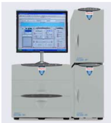
Figure 3-32. Monitor Mounted on Top of the DC
