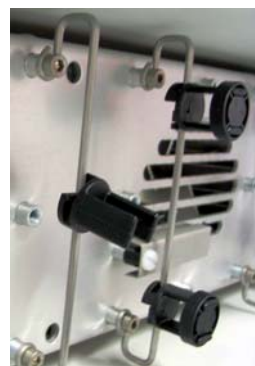
Figure 3-20. Column Clips Installed
