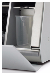
Figure 28. Waste container compartment
