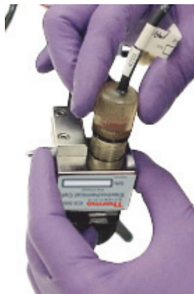
Figure 30. Installation of the pH-Ag/AgCl reference electrode in the reference electrode well
