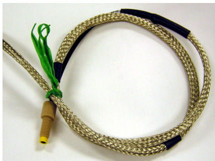
Figure 14. Dionex Integrion main waste line
