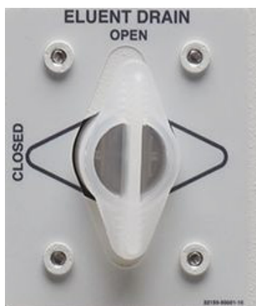
Figure 16. Eluent drain valve settings
