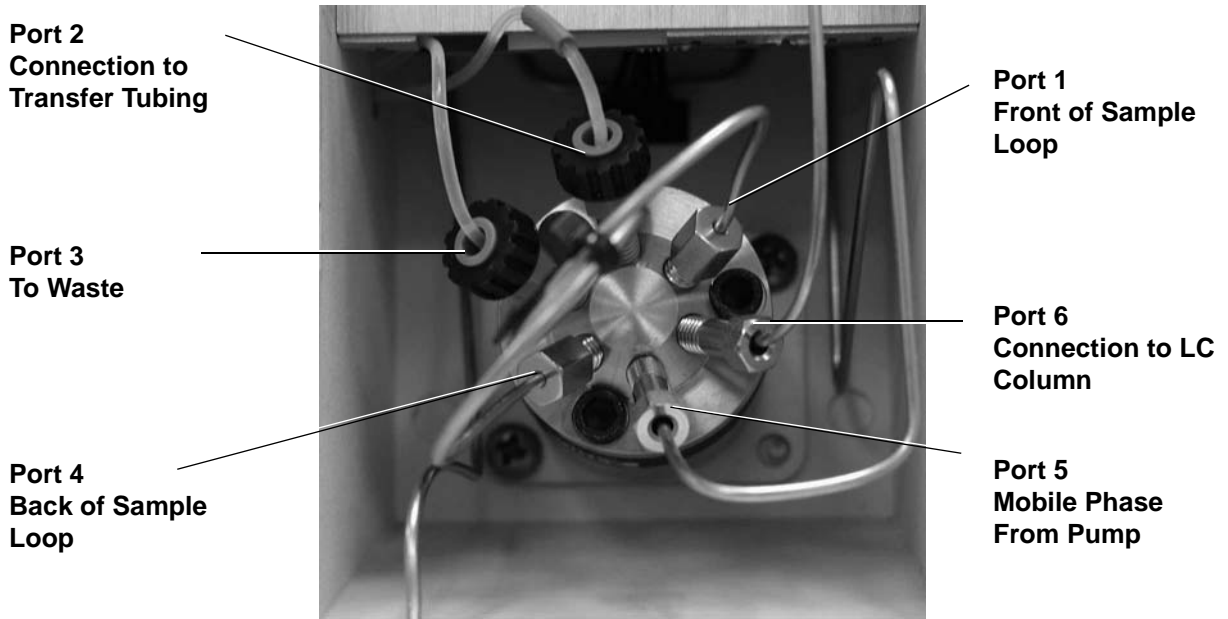
Figure 4-9. Six-Port Rheodyne Injection Valve (7739)
