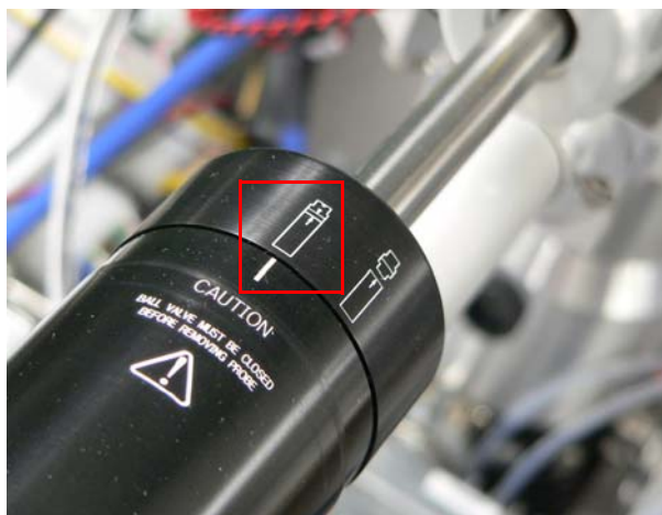
Figure 3-20. Ion volume tool handle in the locked position
