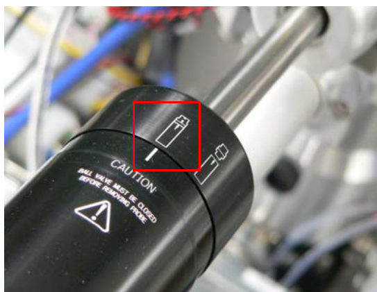
Figure 3-24. Ion volume tool handle in the locked position
