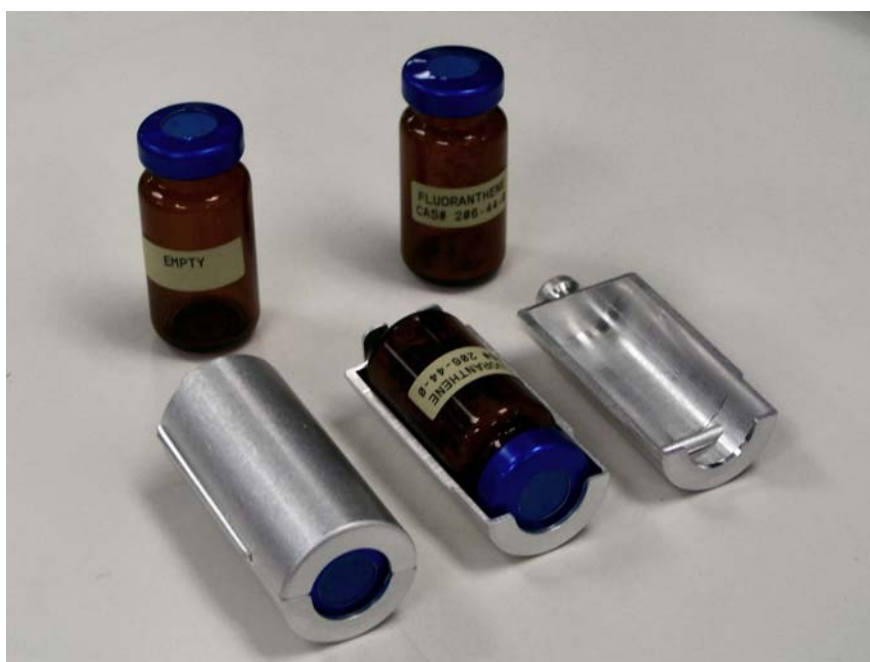
Figure 3-44. Reagent vials with holders
