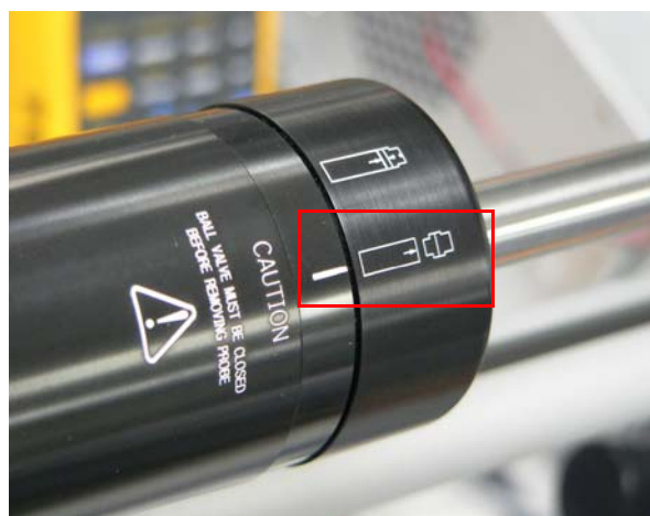
Figure 3-14. Ion volume tool handle in the unlock position
