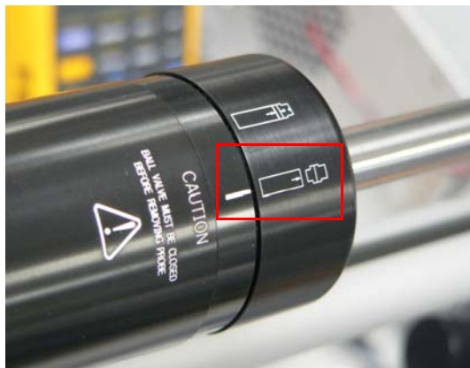
Figure 3-23. Ion volume tool handle in the unlock position
