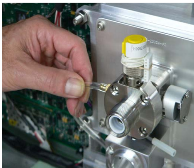
Figure 3-28. Removing the foreline hose from its connection
