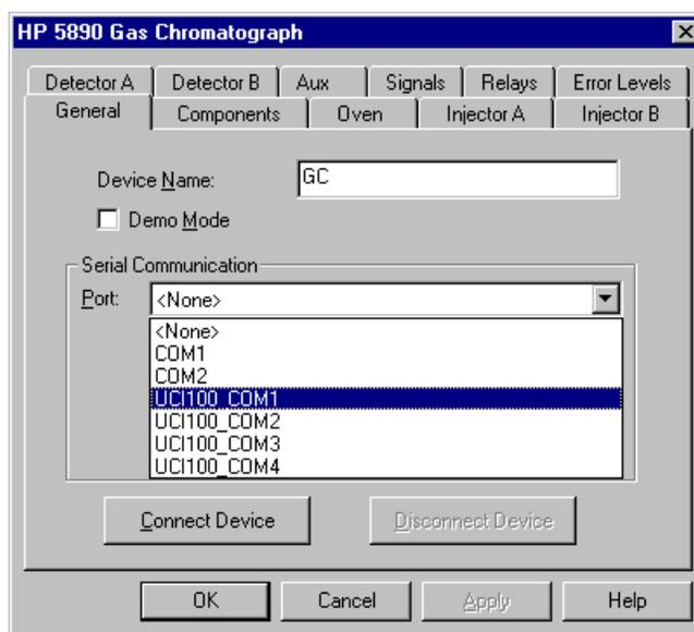
On the *Components* tab, select the installed devices.
