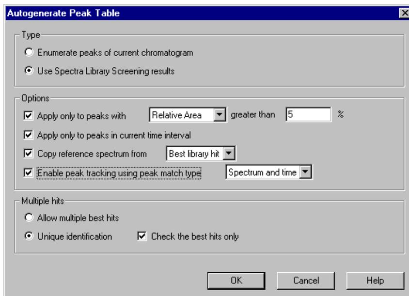
In this case, library screening is performed based on the parameters entered in the QNT file. All peaks for which at least one reference spectrum was found, are included in the peak table with the name of the best hit.
