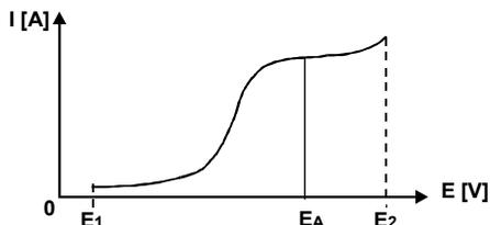
In all three cases, current/voltage curves (here represented by a **half scan**) are recorded. The working electrode potential ( $= E_A$ ) here corresponds to the optimum analytical potential of a substance. Determining this potential is required for accurate analysis in the  $\triangleright$  *DC Mode* and the  $\triangleright$  *PULSE Mode*.
