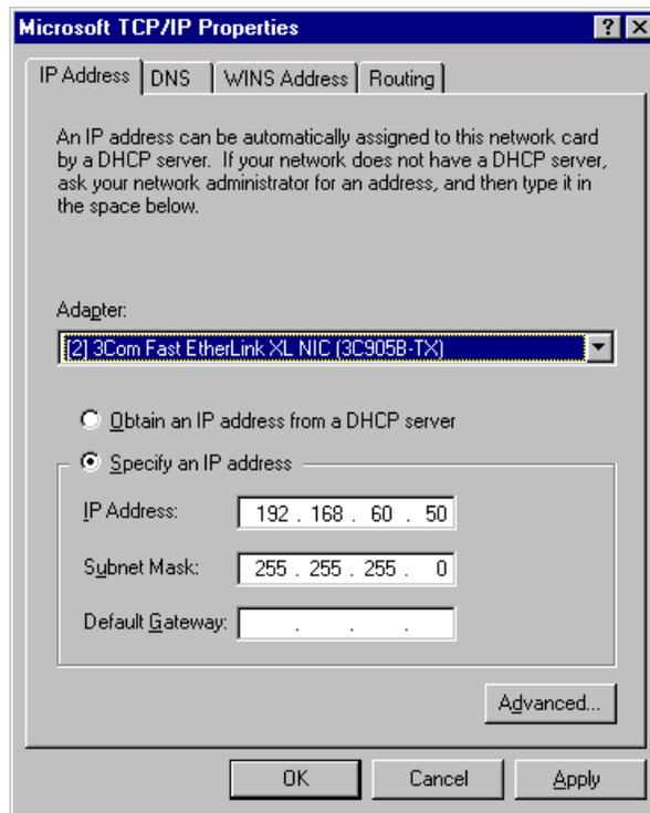
When selecting the IP address of the network adapter of the server PC ensure as well that, with the above subnet mask (255.255.255.0), only its last digit differs from the IP address of the UCI-100. Otherwise, the UCI-100 cannot be addressed.
