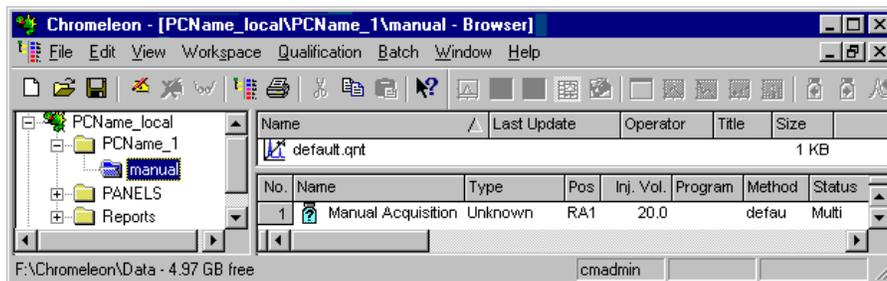
The local datasource has the name <PCNAME\_local>. It contains the subdirectory **PCNAME\_1** in which the **➤Sequence "manual"** is located. The sequence consists of a single default sample and enables the manual data acquisition. To access default templates directly in the Dionex Chromatography Management System, subdirectories of the DATA directory are mapped (PANELS, REPORT...).
