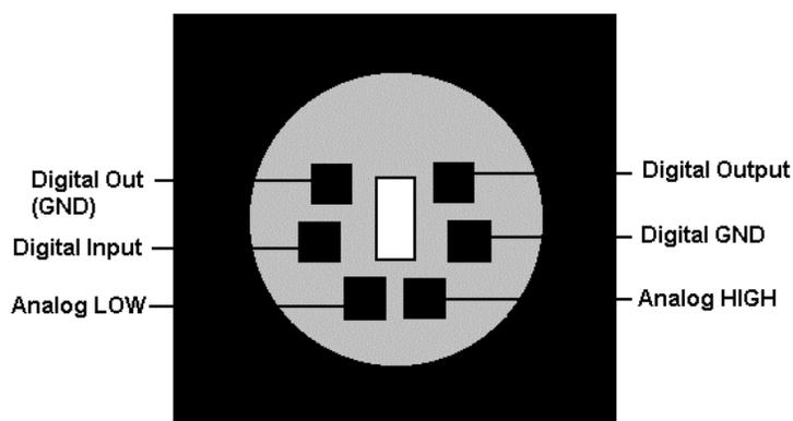
The range of the 6-pin analog input is as follows:
