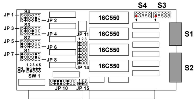
Each physical interface corresponds to a logical interface that is configured via different address combinations (I/O-address). Each logical interface can be assigned to one of a maximum of eight available interrupts.
