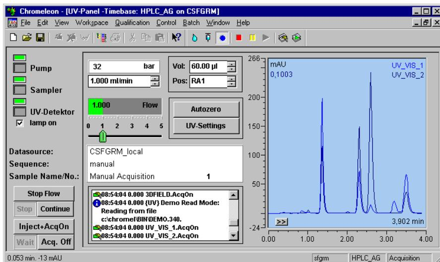
The above screen shows a control panel that allows controlling the basic functions of a pump, an autosampler, and a two-channel UV detector. On the right, you can see the detector signal.
