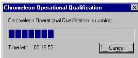
6. While the OQ is running, the Dionex Chromatography Management System is locked. This lock can be removed only by pressing **Cancel** in the active window **Chromeleon (or PeakNet) Operational Qualification**.
