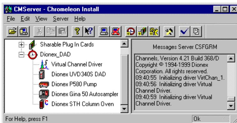
By default, the Dionex Chromatography Management System generates 16 virtual channels. All individual channels have the same sampling step. If you require different sampling steps, install another instance of the virtual channel driver.
