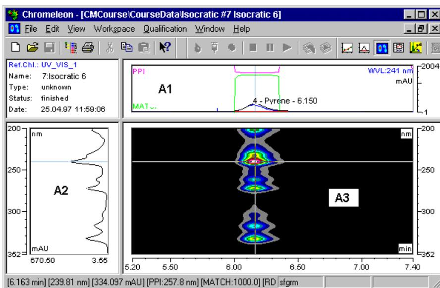
The display of the window sections A1 and A2 can be enabled or disabled via the **Show Chromatogram** or **Show Spectra** options. Optionally, an additional numeric report (PPA report) can be displayed (**Show Report**). The line of the currently selected peak is highlighted by a different color.
