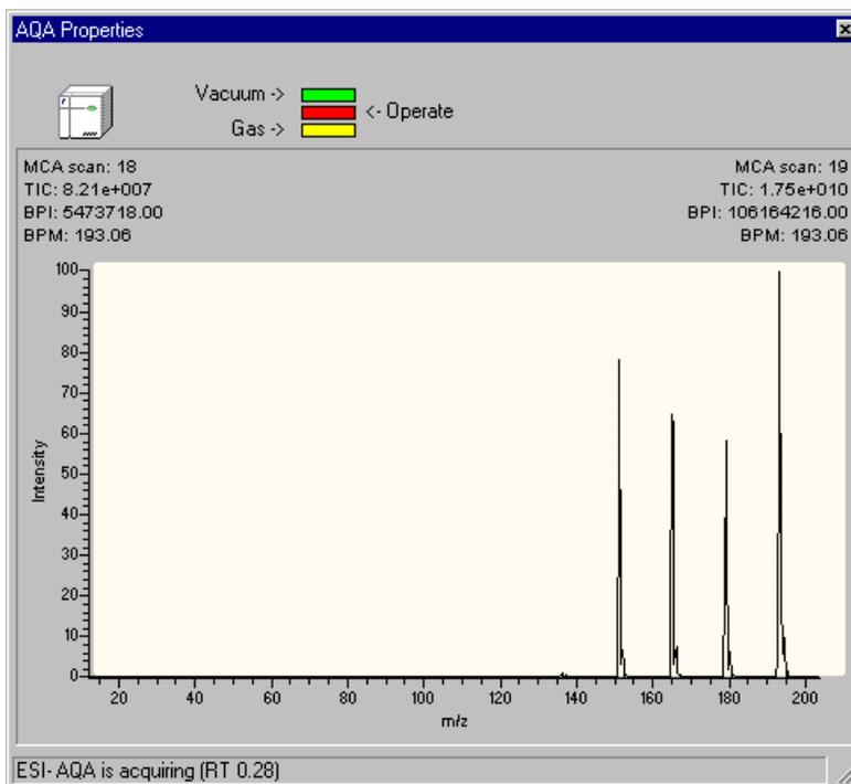
The status bar indicates the time that passed since the data acquisition was started. At the top left and right, the results of the last two scans are given.
