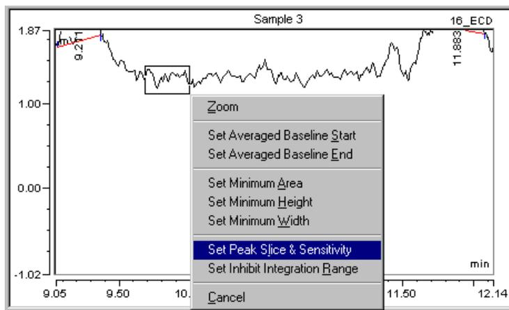
The width of the selected area is entered into the QNT method as peak slice and the height is entered as sensitivity at the time of the left edge of the area. Enter 0.000 as time onto the **Detection** tab or move the parameters in the chromatogram with the **Detection Parameter Tool** so that this peak recognition algorithm applies to the entire chromatogram.
