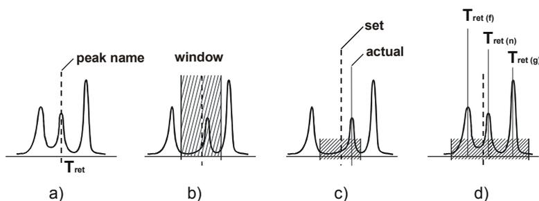
The retention time value previously entered in the peak table is corrected accordingly!
