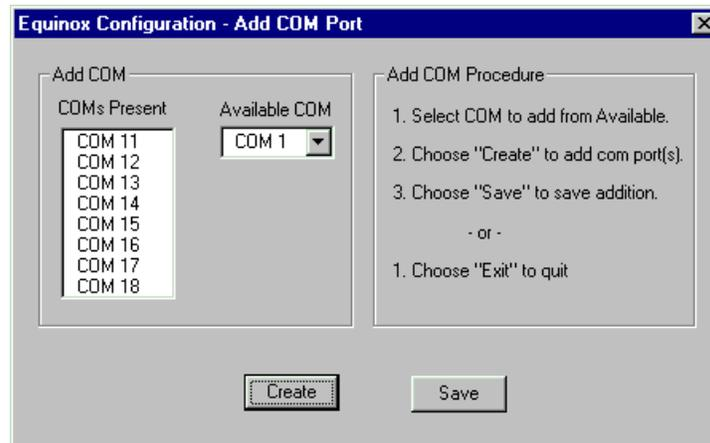
Via **Available COM**, choose a COM number and then press **Create**. Perform this four times for the 4-fold board, and eight times for the 8-fold board. NOTE: Start with COM 11. You will thus prevent overwriting an existing COM port assignment (e.g. COM1 = mouse port)!
