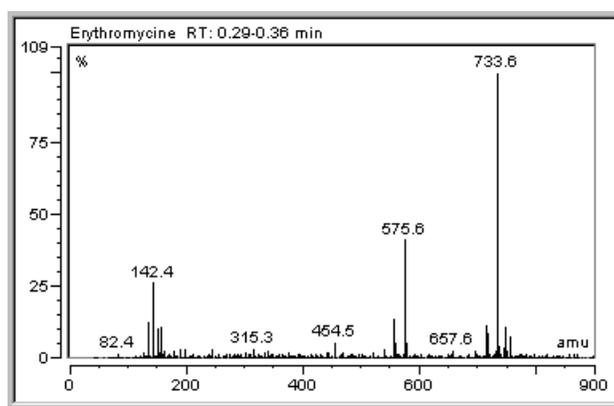
The base peak in the above example is the mass peak at 733.6 amu. The time when the mass spectrum was recorded is indicated as well. The mass spectra in the example were aggregated to the displayed total mass spectrum between 0.29 and 0.35 min.
