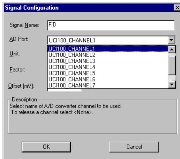
Assign a channel to the signal and name the signal in the **Signal Name** field according to the selected detector type.
