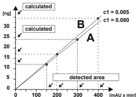
If the calibration points are not located exactly on one line, the data system calculates an optimized, approximate c1 value for each substance from the **➤ Calibration Function**.
