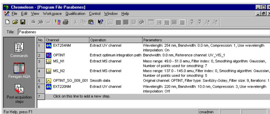
In step 1 and step 6, two UV channels are extracted at 254 and 220 nm, respectively. The EXT254NM channel does not use compression; data that were acquired at 254 nm are used only. For the EXT220NM, a range von 10 nm was selected, i.e., the wavelengths from 215 to 225 nm were used. In addition, compression is used during channel extraction. Compression = 3 means that every third datapoint is saved only.
