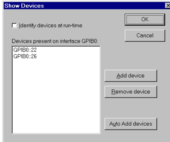
Ensure that the **Identify devices at run-time** checkbox is **disabled** and use the **Add Device** button to manually add the GPIB address you will be using for your module(s). For information on the default GPIB address of each module see the corresponding Agilent manuals.
