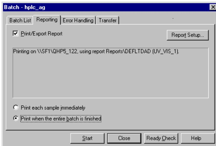
The **Print/Export Report** option opens the above dialog box (that is displayed in the Browser section) once again. Proceed as described above. The window on the tab indicates the printer, report definition file (RDF), and channel to be used for the printout. In addition, you can specify whether to print each sample separately and directly after the data acquisition or all samples when the batch is finished.
