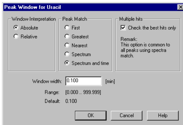
The algorithm for peak identification via a spectra comparison can be described as follows: If **(Peak Match) Spectrum** or **Spectrum and time** is selected as peak match criterion in the **Window** column of the peak table, peak tracking uses the reference spectra in the corresponding column (in the case of **Spectrum and time** limited to the specified time window). Peak tracking generates a list of spectra sorted by the match factor (the peak hit list is not shown here).
