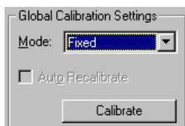
In **Fixed** mode, manual calibration is possible only, i.e., after adding standards on the **Calibration** sheet (see below) press the **Calibrate** button on the **General** sheet to include the newly entered standards in the calibration.
