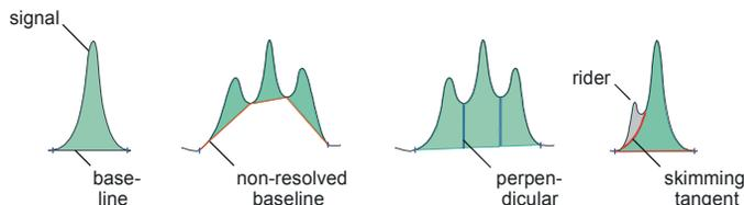
Rider peaks have a separate area that is limited by a skimming tangent and the signal curve.
