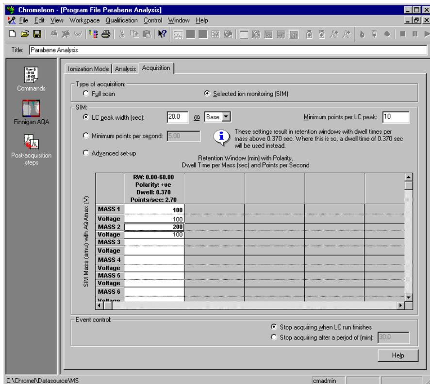
The SIM1 channel records the chromatogram at a mass of 100, the SIM2 channel records the same chromatogram at a mass of 200.
