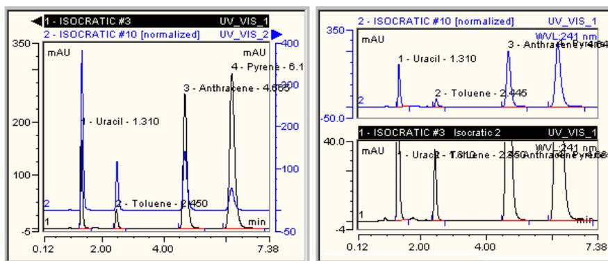
The **Overlay** view allows adding an additional signal axis (on the right) for the overlaid chromatogram that was added last via the **Overlay with right signal axis** command. This command, too, is available on the **Comparison** tab of the **Chromatogram Decoration** dialog box. Thus, you can select a different signal range for the chromatogram that was added last. The **Stack** view allows individual scaling of the signal axis for each single chromatogram.
