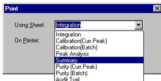
In the dialog box, select the worksheet to be printed. The sheet will always be printed with the results that are currently displayed on the screen provided they are included in the defined view. For example, the current mass spectrum will be printed only if a mass spectrum is part of the selected worksheet.
