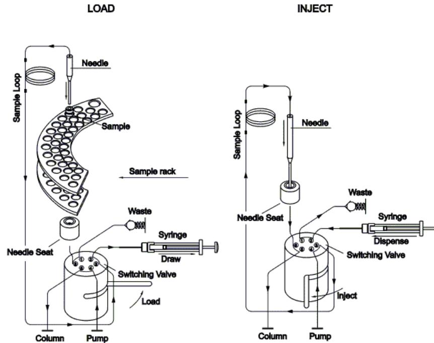
The Dionex Autosamplers Gina 50, Gina 160, ASI-100/ASI-100T, and AS50 function on this basis. Apart from the standard model, a coolable version (Gina 50T) and a model with integrated derivatization or method program (Gina 160) are available. (With the ASI-100/ASI-100T samplers, derivatization and method programming is possible with the standard version.)
