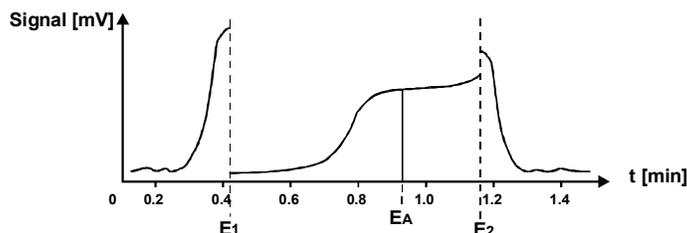
Unlike the pump, the chromatogram run time is not stopped. The retention times of the subsequent peaks will be shifted accordingly. However, the signal height of the peaks will be lower as part of the substance is "used up" during the **Scan** mode.
