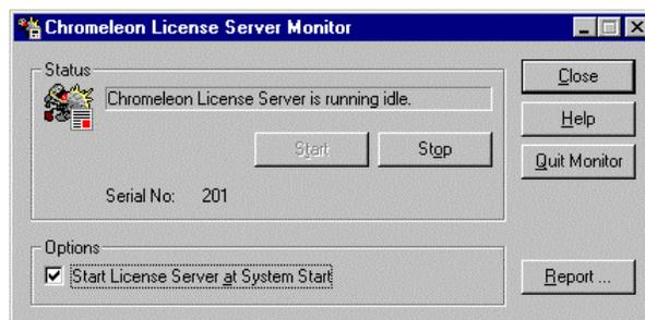
A configuration file for the License Server is supplied together with the distribution. However, this file needs to be adapted to local requirements. Replace the computer names PC\_XX in the [Servers] section of the file **CmLicSrv.ini** by the names actually used in your network (e.g. ALPHA, BRAVO...). This is to assign serial number/Key Code pairs to the servers of the Dionex Chromatography Management System:
