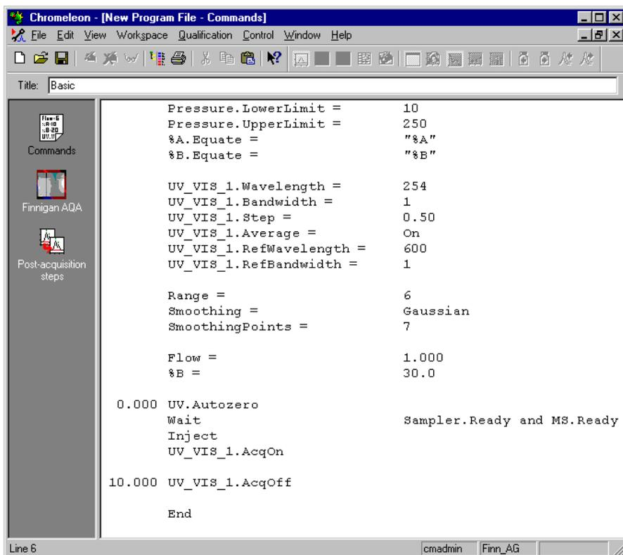
The Wizard-generated PGM file provides no  $\Rightarrow$ AcqOn/Off (*Data Acquisition On/Off*) commands for the aQa channels. The channels that are needed for mass trace acquisition depend on the contents of the MS method.
