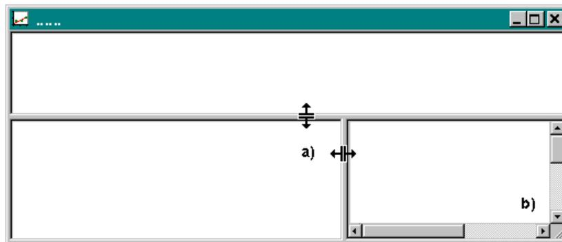
The contents of the window section depends on the type of the represented data. Table or text editors can also be integrated as a window section in a method window. Window sections with a graphical representation show the coordinates of the mouse cursor in the status bar.
