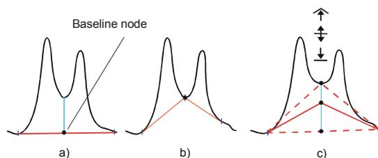
If the baseline should be drawn from peak end to peak end, activate the  $\Rightarrow$  *Valley to Valley* detection parameter. The baseline node is automatically moved towards the signal curve until it rests on the curve in the minimum between two peaks (b).
