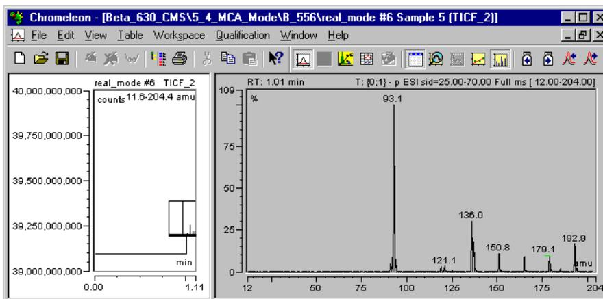
The "chromatogram" in the left pane contains one datapoint only that is at the highest retention time. To illustrate the summing up of the entire acquisition period, it shows one line in the height of the entire counts of all summed up mass spectra. In addition, only one single (entire) mass spectrum is displayed in the right window section.
