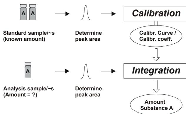
How many peaks are detected and whether at least part of these peaks can be identified, depends on the
