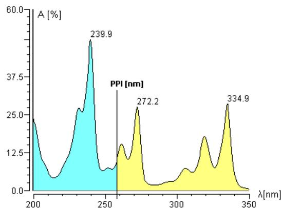
A pure single peak should supply the same PPI value from peak start to peak end for each spectrum recorded in this range. The following conditions must be fulfilled:
