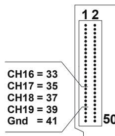
**⚠ Caution:** Always use the analog ground (Pin 41), **not** the digital ground (pin 44)!
