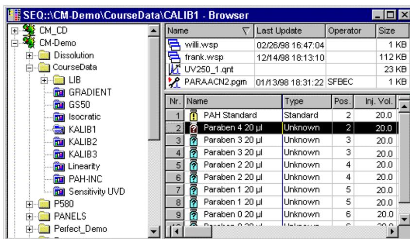
Subdirectories, sequences, and chromatographic methods can be moved via **Drag & Drop** within a datasource, but also between datasources of different types. This copy process can also change the underlying database! If you want to actually move a sample, note that the original sample must be deleted in the Browser after the copy process.
