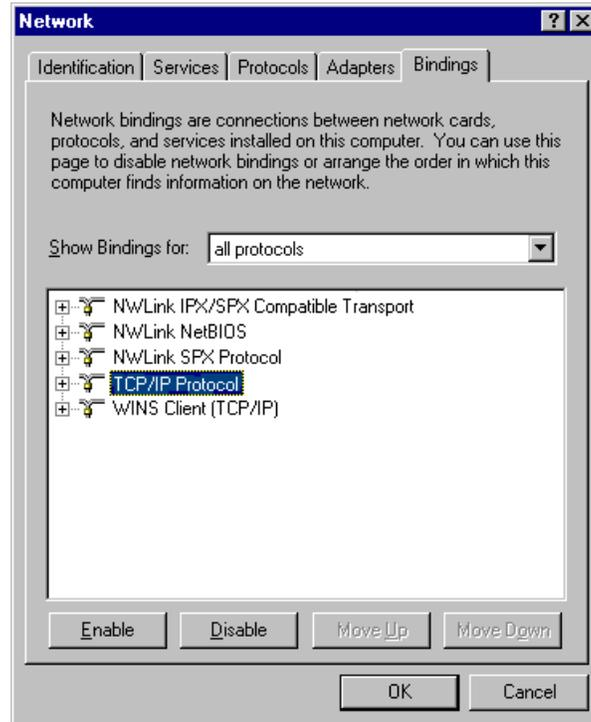
Then, select **all adapters** under **Show Bindings for** and deactivate all protocols for the peer-to-peer connection except the TCP/IP protocol:
