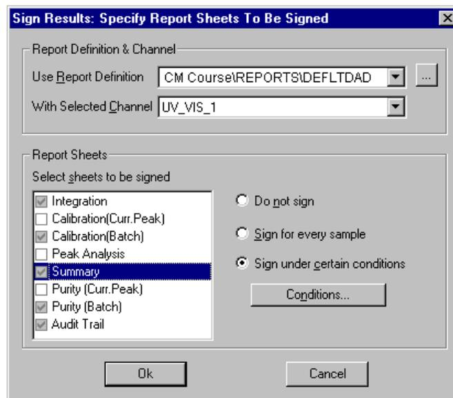
Select the **Report Definition** file (RDF) to be used for displaying the sequence as well as the channel for which to show the results. In the lower window part, you can define the pages of the RDF file to be signed.
