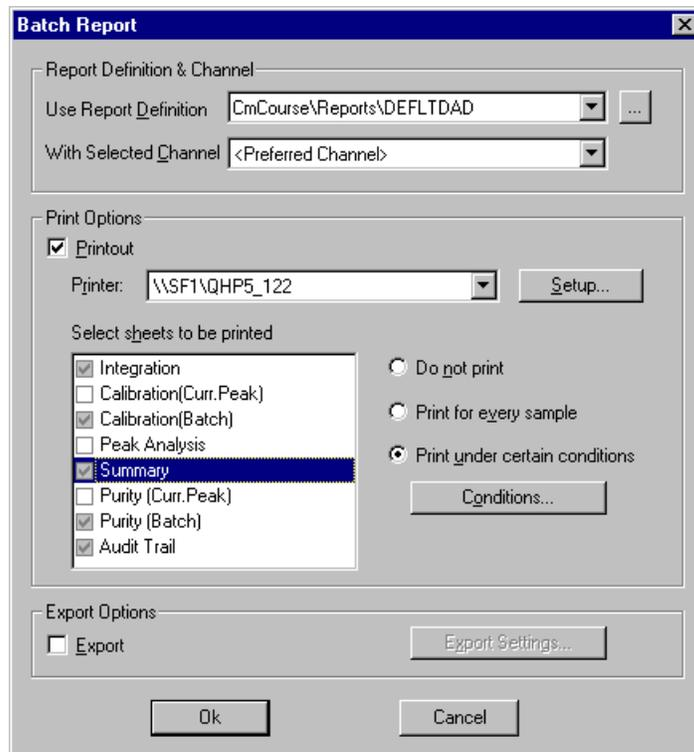
The **Select sheets to be printed** field shows the worksheets that were defined in the printer layout of the report template. Specify which pages shall be printed. Define under which conditions they shall be printed via the **Conditions...** button. Pressing **OK** then prints the entire sequence or the selected samples of a query. Select all samples of a query by clicking the **No.** field at the top left of the sample list to print the entire query.
