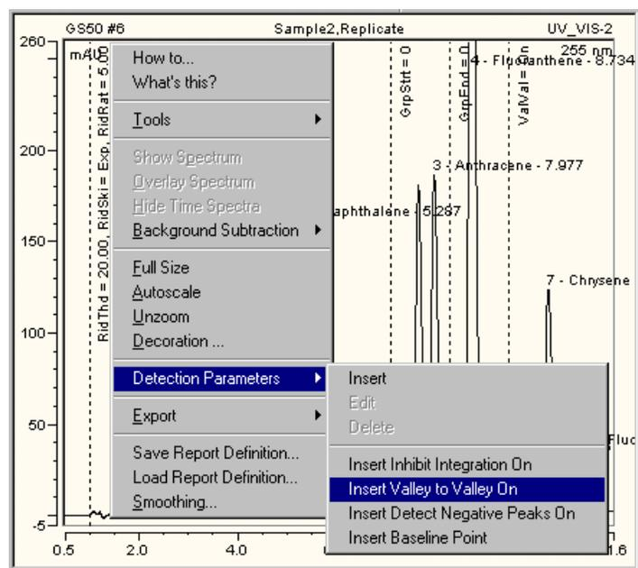
In the chromatogram, a dotted vertical line at which the abbreviation for the parameter and its respective value are given indicates the parameters. In the illustration, see e.g. the values for the Rider Threshold (in short: RidThd), Rider Skimming (RidSki) and Maximum Rider Ratio (RidRat) parameters at 1.000 min.
