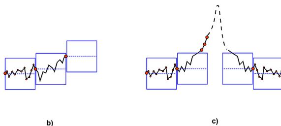
If three successive data points are located above or below the rectangle (simplified!), the peak recognition algorithm will recognize a peak. When the signal difference of one data point to the next one becomes so small that they are within the bandwidth again, the peak end is indicated (c).
