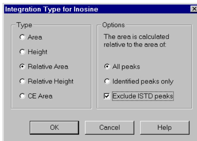
In addition to **Area**, **Height**, and **CE-Area**, you can select the relative area or the relative height as the reference for the evaluation (Integration Type).
