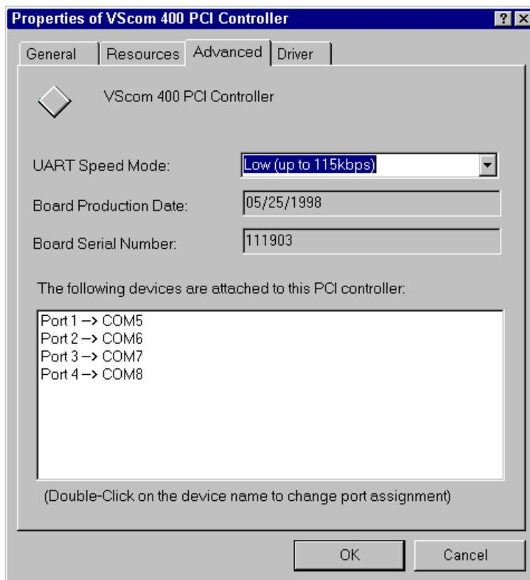
**⚠ Caution:** For operating the PCI board via the Dionex Chromatography Management System, enter **Low (up to 115 kbps)** on this sheet.
