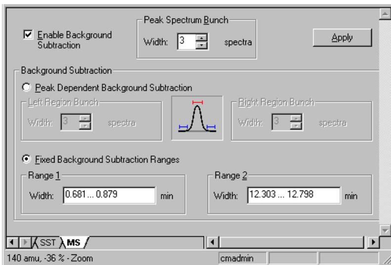
Under **Peak Spectrum Bunch**, indicate the number of single spectra that shall be aggregated to the spectrum at the peak maximum. It is possible to average max. 99 single spectra. For symmetry reasons, odd numbers can be entered only.
