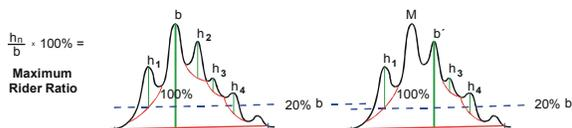
As can be seen in the figure, not the "real" peak height of the peak to be classified is evaluated but the distance between the peak maximum and the skimming tangent.
