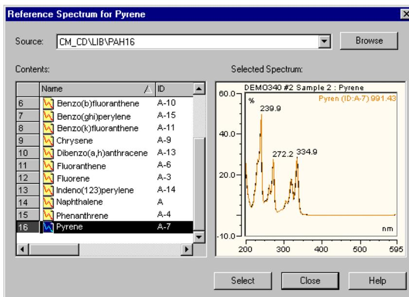
After pressing the **Select** button, the selected reference spectrum is copied to the corresponding line of the peak table.
