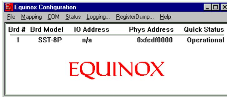
If the board functions correctly, the **Quick Status** will indicate the status **Operational**. If this is not the case, detailed information is available via the **Status** option. NOTE: If the board is not recognized correctly, you may have to use a different PCI slot.
