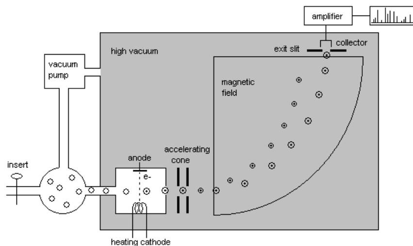
The ions that are created via the electron impact are first accelerated by means of the cones and then separated according to their mass in the magnetic field. Due to the varying intensity of the magnetic field (or the accelerating voltage), ions of different masses are directed through the exit slit into the collector and registered. In this way, mass spectrometers perform a mass scan similar to the wavelength scanning of many photodiode array detectors.
