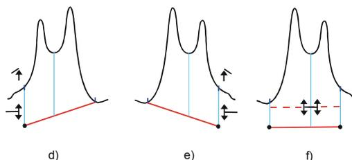
The system automatically makes a distinction between moving a peak delimiter horizontally and a baseline node vertically depending on the direction in which the mouse cursor is drawn.
