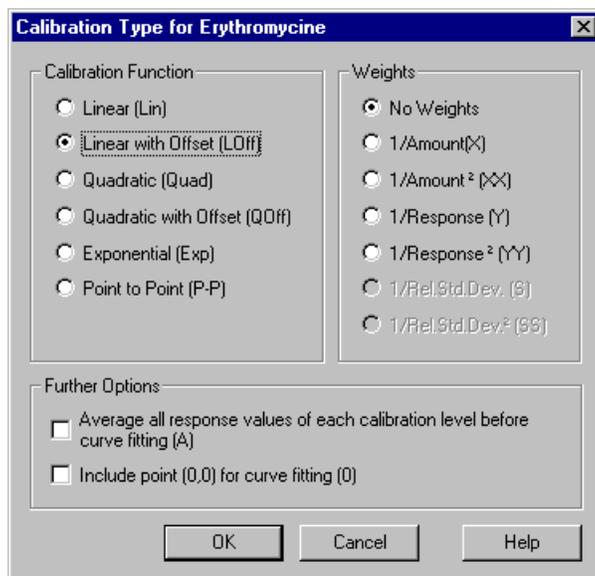
The  $\Rightarrow$  *Calibration Type* determines which  $\triangleright$  *Calibration Function* is used for deriving a valid amount/area assignment for a larger range from the calibration points of the standard samples. For detailed information on linear and non-linear calibration types, see **Calibration Types (Linear)**, or **Calibration Types (Non-linear)** in the **Calibration** section.
