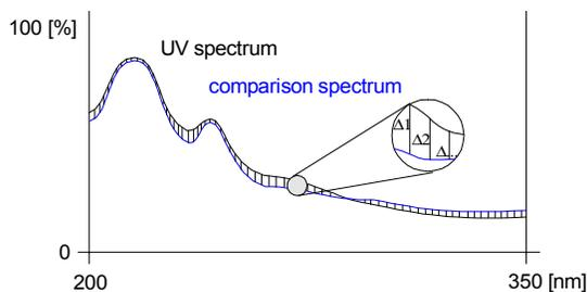
The method provides a value of similarity (match) between completely different (= 0) and identical (= 1000).
