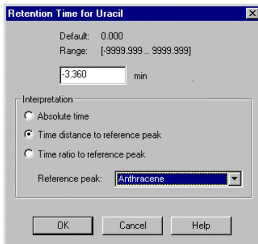
The display of the retention time (relative or absolute time) can be determined individually for each peak on the tab **Interpretation**. Note that relative times can be displayed either as difference or as percentage ratio to the retention time of a reference peak.
