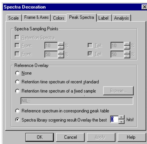
In this example, you will receive a list of three reference spectra. The first spectrum has the highest match value and thus the greatest similarity to the original spectrum.
