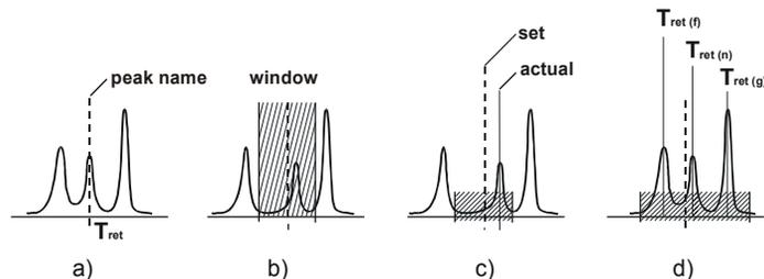
The **Peak Window** can be set for each peak after pressing the F8 key or double-clicking the **Window** column. First, determine the window interpretation. Selecting **Absolute** allows you to enter the window width in minutes. Select **Relative** to define the window width in percent.
