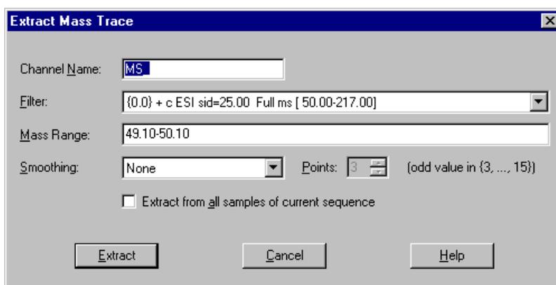
First, enter the name for the new channel. Then, select the desired filter and mass range as well as the **Smoothing** type for the MS chromatograms and the number of data points to be used. Pressing **Extract** makes the new channel available for chromatogram representation.
