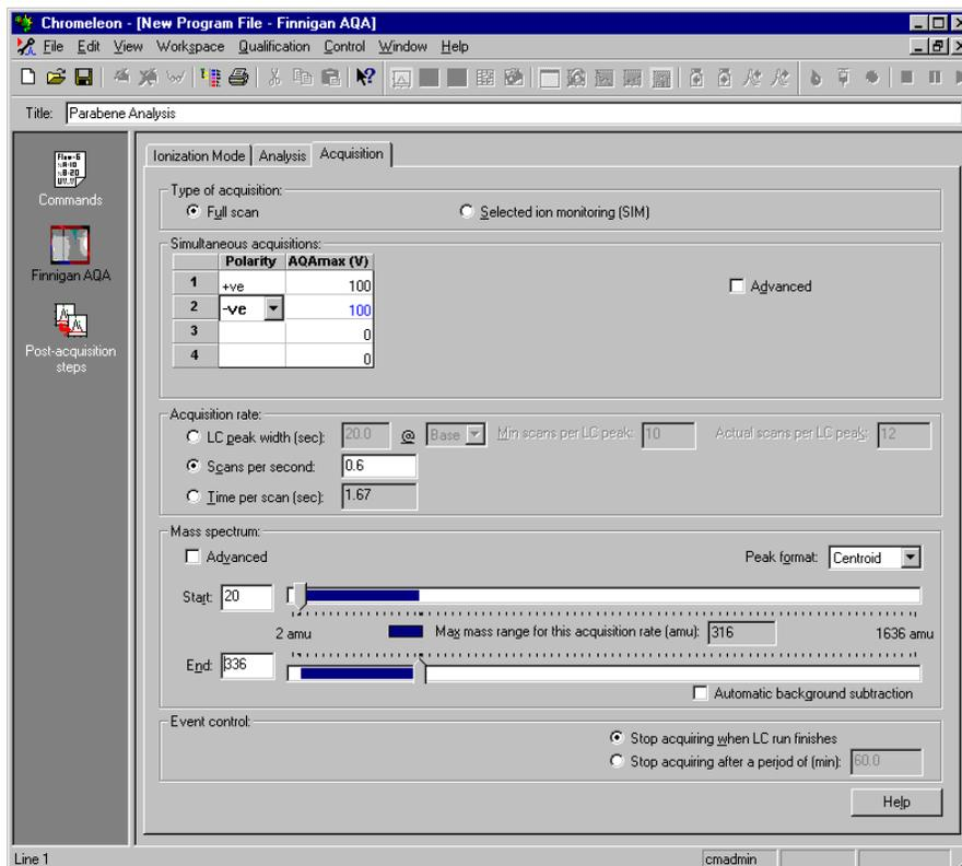
Select the data acquisition mode first: ➤ *Full-Scan* to acquire the entire mass spectrum for each analyte or ➤ *SIM* to obtain MS chromatogram at a defined mass.
