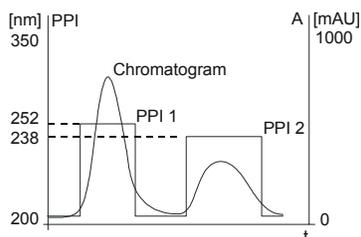
Significant deviations from the rectangle shape indicate peak impurity. However, it is not necessarily correct to deduce from the rectangular shape that the peak is pure.
