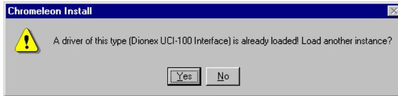
Answer the question whether to load an instance with **Yes** and proceed as described under items 8 and 9 above. Upon completion of the installation the newly installed UCI-100 Interface is shown in the server configuration together with its respective instance number.
