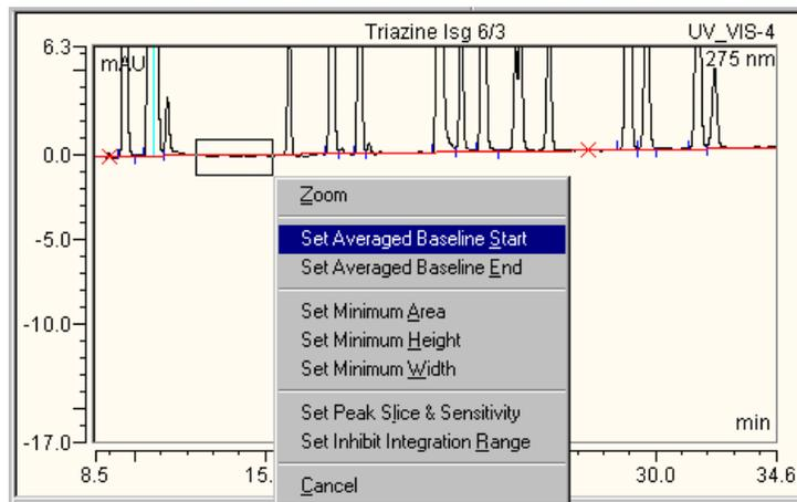
This sets the first baseline point. The x-value is the middle of the selected area while the y-value is the averaged value of the signal values weighted by the data rate. This first value will not be marked, as it is not sufficient for setting the baseline. A second point is required as well.
