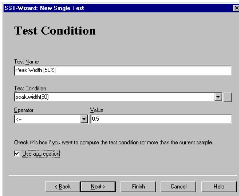
The screenshot shows a dialog box titled "SST-Wizard: New Single Test" with a close button (X) in the top right corner. The main heading is "Test Condition". Below the heading are several input fields and a checkbox:
