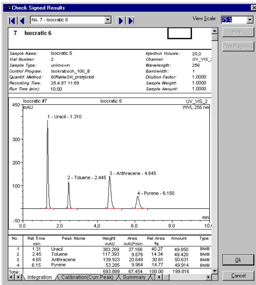
This allows you to check the report to be signed. Use the arrow keys to toggle between the different sequence samples. For each sample, the tabs for the selected report pages are displayed. Pressing OK when you have terminated your checks opens the **Submit Signature** dialog box opens in which the SOR file is signed by entering the User ID and the signature password:
