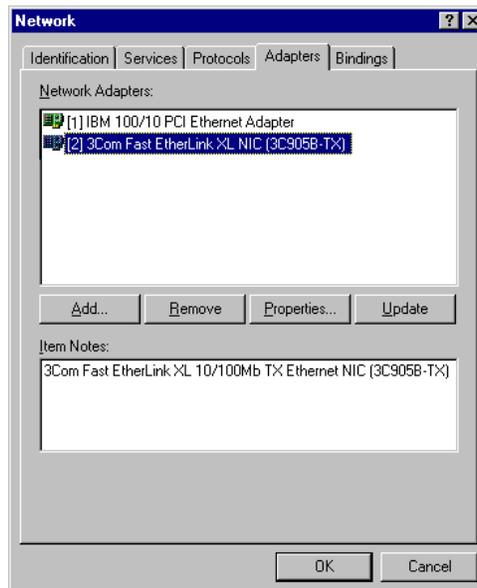
Configuring the network adapter (here [2] 3Com EtherLink XL NIC (3C905B-TX)) is on the **Bindings** tab. First, check via **all protocols** under **Show Bindings for** whether the TCP/IP protocol is installed. Install the TCP/IP protocol, if necessary:
