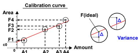
Variance is therefore a criterion for the measuring accuracy in the calibration. With an increasing value, calibration points are increasingly scattered.
