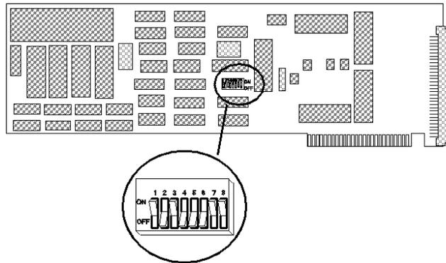
Position the board as indicated in the figure, using the block with the eight switches for setting the I/O-address as a guideline. Proper installation is in three steps:
