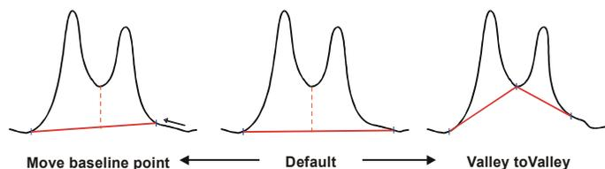
If single peaks are piled on a recognizable "absorption mound," these are integrated individually. To be able to integrate the entire area, the baseline can be fixed. The parameter  $\Rightarrow$ *Lock Baseline* extrapolates the baseline horizontally to the intersection with the signal curve. The **Global Minimum** option searches for the absolute minimum in the direction of the peak end or until the next **Lock Baseline**. Both parameters deactivate the **Valley to Valley** option!
