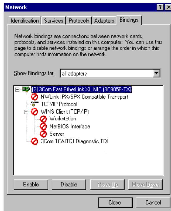
As the TCP/IP protocol is used for the peer-to-peer card, an IP address and a subnet mask are required for the second network adapter. Adjust the properties of the TCP/IP protocol via Start => Settings => Control Panel => Network => Protocols. Select TCP/IP protocol, right-click and select Properties...
