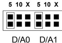
In the above example, the 5V setting was chosen twice, i.e. channel 1 and channel 2 supply voltage in the -5 to +5V range via the bipolar output (pins 17 and 23) and voltage in the 0 to +5V range via the unipolar outputs (pins 18 and 24).
