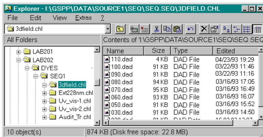
In this example, the channels **3dfield**, **Ext228nm**, **Uv\_vis-1**, and **Uv\_vis-2** were defined. The protocol data directory **Audit\_Tr** was added. If a directory is expanded, the raw data of the corresponding channel is visible.
