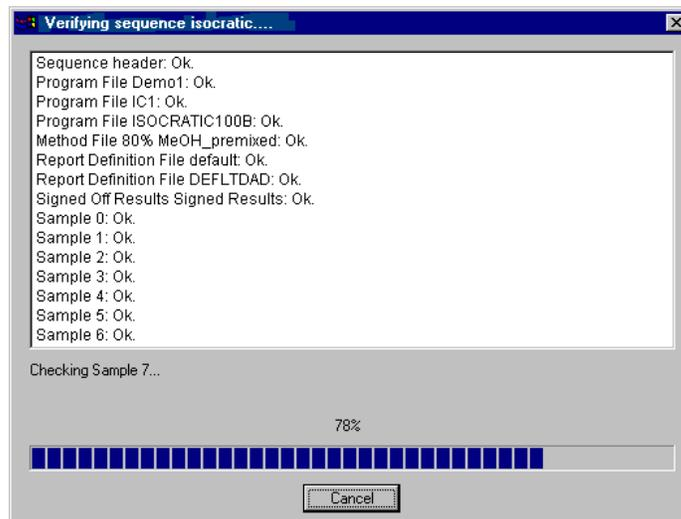
(This process is completed much faster than with **Submit** so that the above dialog box will be visible for a few seconds only, especially with short sequences.) To **approve** a sequence proceed in the same way.
