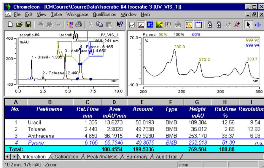
On the top right, the spectrum of the selected peak, e.g., anthracene (provided the analysis was performed with a diode array detector) is displayed; the lower section shows part of the integration report (three lines, the currently selected peak is highlighted by a different background color). As before, the Spectra Plot window can be changed via the **Decorations** command. Choose this
