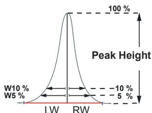
For ideal peaks, Asymmetry is  $A = 1$ . For realistic, tailing peaks, however,  $A$  is between 1.2 and 5. Values higher than 5 often produce imprecise quantitative results.
