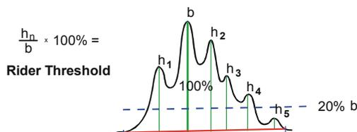
If the height ratio  $h/b$  multiplied by 100 percent produces a value below the defined rider threshold, the corresponding peak is by definition a main peak. Here, this is only the case for the h5 peak.
