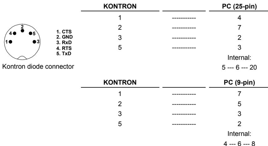
The baud rate set on the unit must correspond to the baud rate specified in the Dionex device driver. Normally, the baud rate is 4800 bit/sec.
