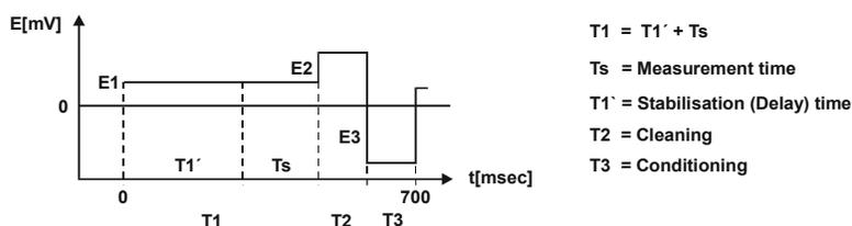
Data is recorded only during the second half of T1. The duration of Ts is either set directly or is determined by defining a delay T1' (stabilizing phase).
