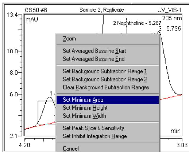
This action enters the selected area as minimum area together with the time of its left edge into the QNT method. Enter the 0.000 as time into the **Detection** tab or move the parameter in the chromatogram with the **Detection Parameter Tool** so that the minimum area is valid for the entire chromatogram.
