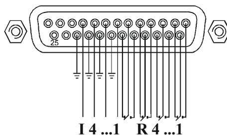
The maximum switching potential of the relays is 100 V with a contact rating of 10 W. Ensure not to exceed a max. current of 0.5 A. To enable a reaction to external events (e.g. inject signal), the relay board offers four remote inputs, which are released when a relay closing contact (e.g. of the autosampler) grounds the corresponding input signal.
