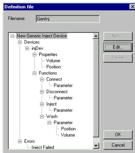
The **New...**, **Edit...**, and **Delete** commands can be selected for the items in the tree structure. **New...** creates an appropriate default entry and opens a dialog box for selecting the settings.
