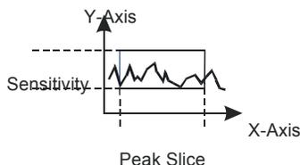
As shown in figure a), this rectangle is placed with its lower left corner on the first data point, and is duplicated by mirroring in the direction of negative y-values. As long as none of the subsequent data points is above or below the mirrored rectangle, the last data point will be used for positioning further rectangles (b). The measured signal is interpreted as noise.
