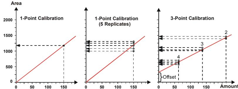
If one calibration sample is analyzed several times, several points can be entered in the amount/area diagram. The points of one concentration are called **replicates**. With an increasing number of available replicates, the impact of imprecision decreases after averaging. In spite of several replicates, only one amount/area ratio is determined. This is referred to as **multi-point calibration on one calibration level** (in the middle of the partial fig.).
