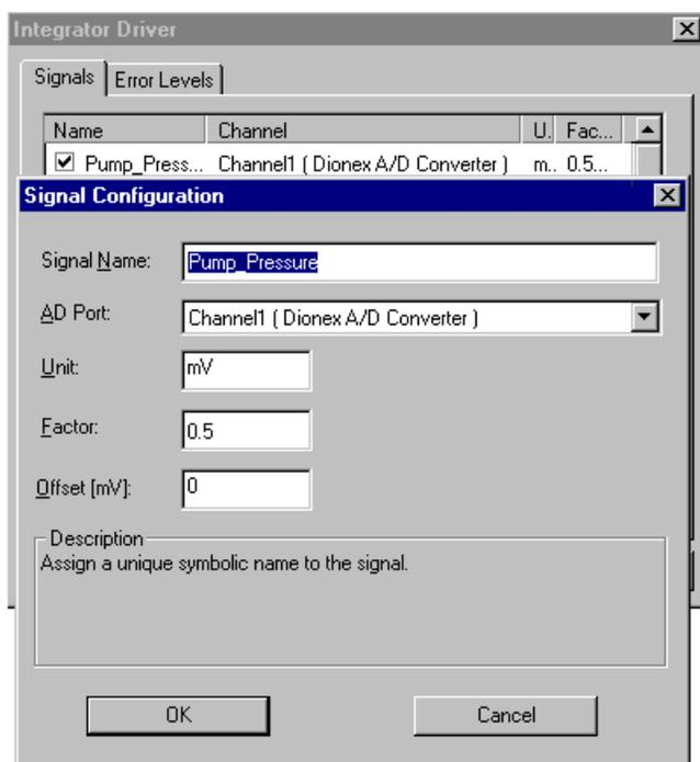
Select the channel to which the pressure output of your pump is connected as **AD Port**. Enter under **Factor** how many bar correspond to an output voltage of 1 mV. For example, enter 0.5 bar/mV for the Dionex P580 pump or 5 bar/mV for the Dionex M480 pump.
