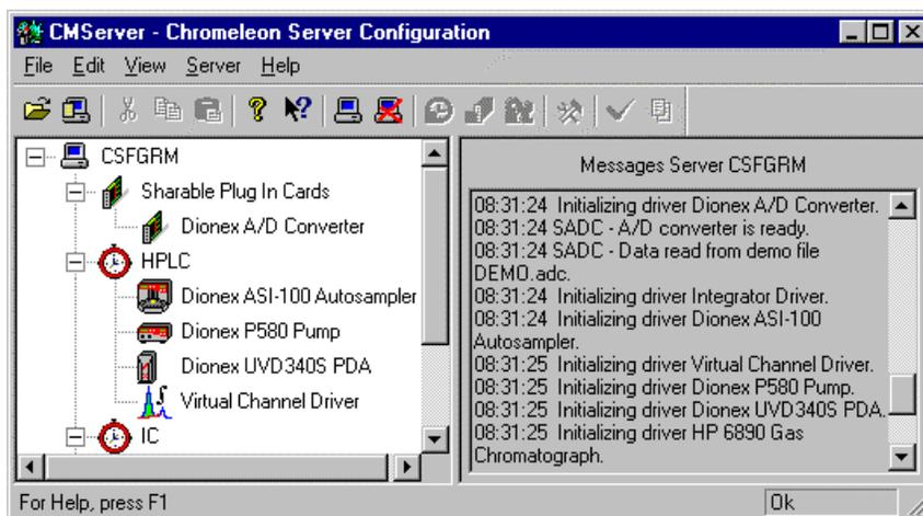
A running server is shown in the shape of a PC icon; an inactive server is crossed out red. A red prohibitive sign (red circle with white line) indicates that a server is active (for example, processing samples).
