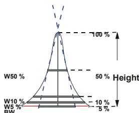
The Dionex Chromatography Management System also determines the peak width at 5, 10, and 50% of the peak height (abbreviations: W5%, W10% and W50%).
