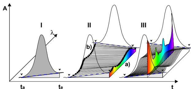
This is performed for all detected wavelengths. The absorbance values at all wavelengths measured at the time  $t_a$  and  $t_e$  result in the baseline spectrum of peak start and peak end (II, a and b). Between these two spectra, the Dionex Chromatography Management System performs an interpolation and thus calculates a separate baseline spectrum for each peak data point. Outside the peak limits, the 3D-field is by definition zero.
