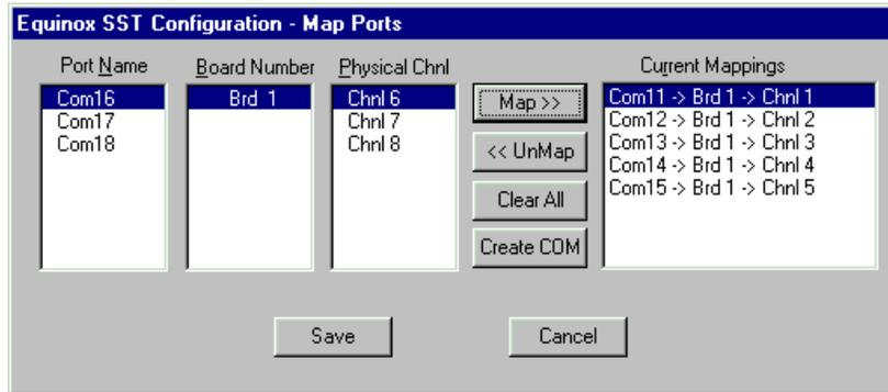
The list box **Port Name** shows all previously installed logical COM ports (e.g. COM11 to COM18). Via **Map**, the logical ports can be assigned physical channels (by pressing the button four or eight times). The result of these mappings is displayed in the list box **Current Mappings**. Save these settings via **Save**. Any error messages can be ignored.
