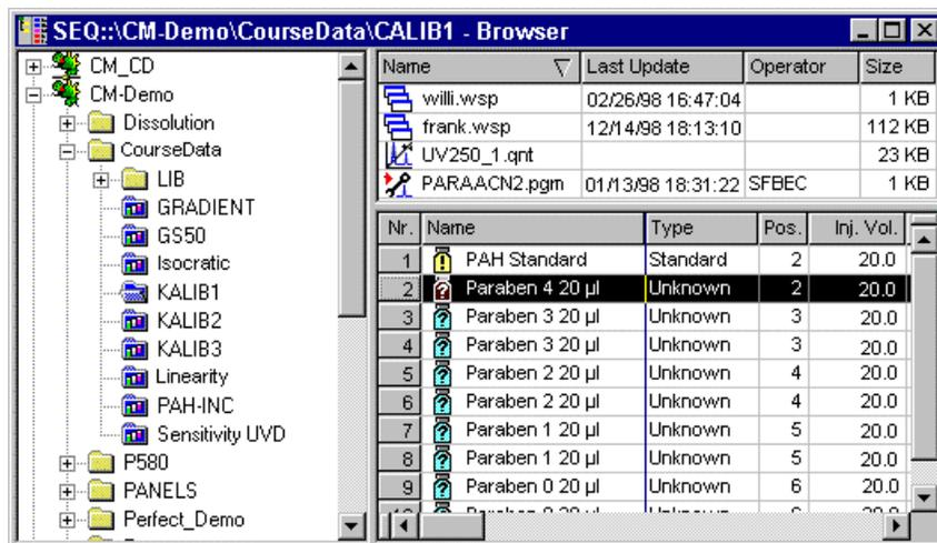
A sample is characterized by various column entries. The entries are managed in a database and are referred to as **Sample Data**. A short explanation of each column is displayed upon pressing the F1 key.
