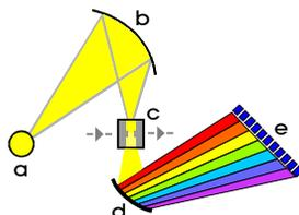
Dionex detectors store this information analog to a UV channel via the signal ➤ *3D-Field*. Apart from the quality of the optics and the grating, the number and size of the photodiodes determine the ➤ *Optical Resolution* of the detector.
