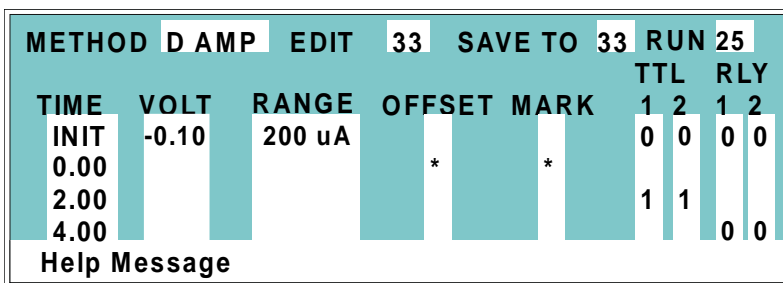
Figure C-14. Method Screen—DC Amperometry
