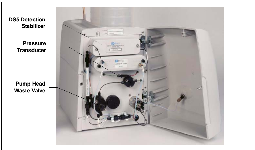
Figure 5-2. ICS-90 Interior Components
