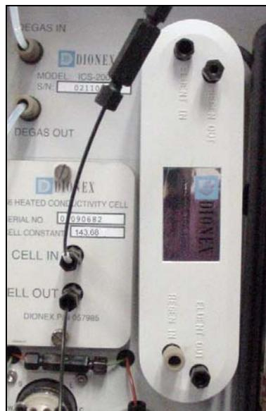
*Figure 21. Suppressor Installed
