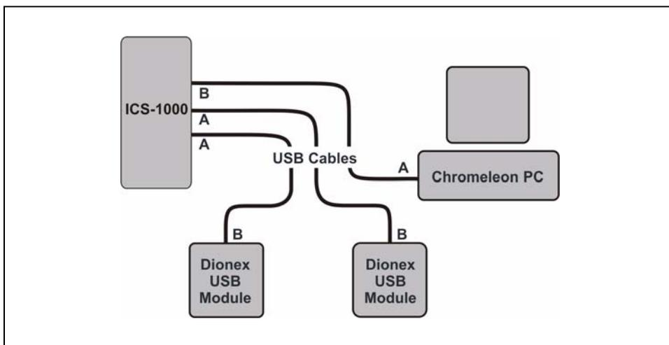
*Figure 8. Example Connections: Two Dionex USB Modules Connected to the ICS-1000*
