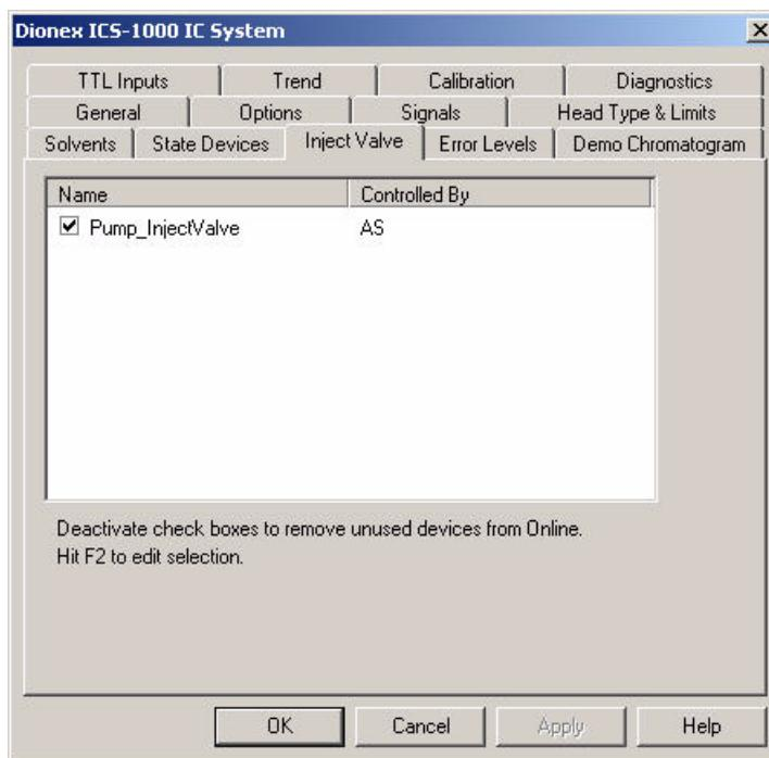
Figure 41. ICS-1000 Inject Valve Server Configuration Properties
