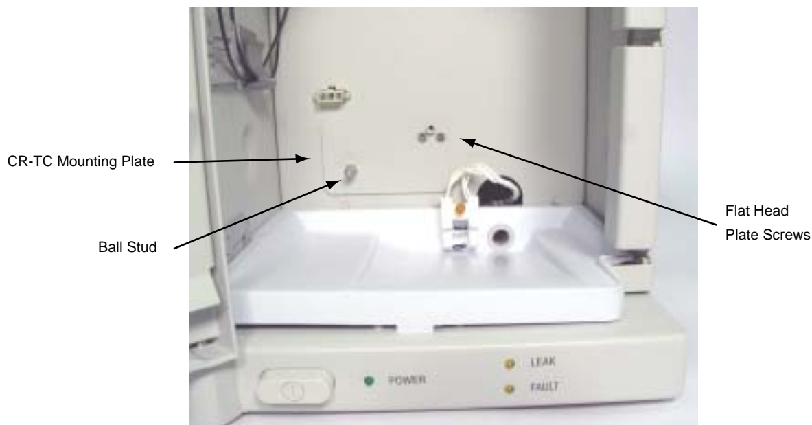
Figure 21 Installed CR-TC Mounting Plate
