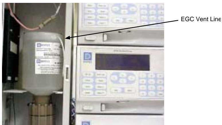
Figure 18 EGC Cartridge Installed in EG40
