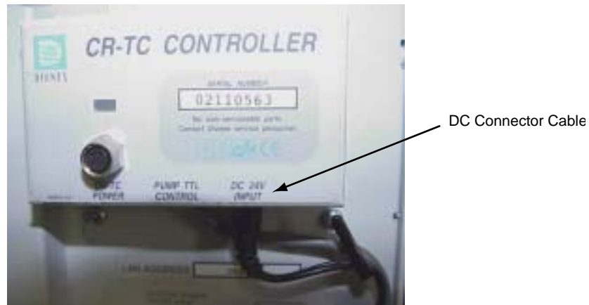
Figure 11 DC Connector Cable Attached to the CR-TC Controller Box
