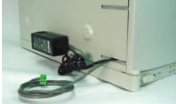
Figure 9 Universal Power Supply Attached to the Exterior of the EG40 with DC 24 V Input Cable and Pump TTL Control Cable
