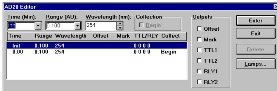
**Range (AU)** sets the full-scale recorder output range to between 0.001 and 2.0 AU. The default is 0.1 AU.
