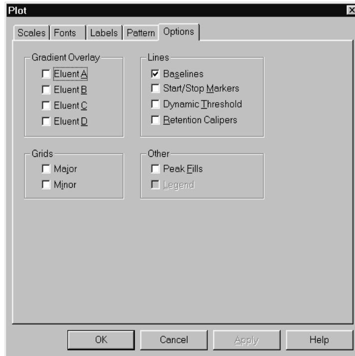
**Gradient Overlay** selects which pump gradient lines to show overlaid on the plot.
