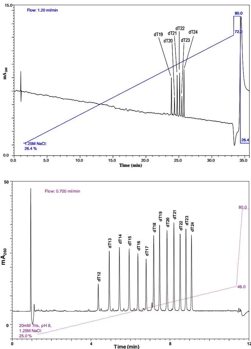
In the example below, the 8 $\mu$ m 4x250mm and 4 $\mu$ m 4.6x150mm columns are compared using a linear gradient of 450-625mM NaCl in 4 column volumes at 1.12ml/min. In this example the 4 $\mu$ m column delivers essentially equivalent resolution for these six oligonucleotides in less than 70% of the time required for the longer 8 $\mu$ m column.
