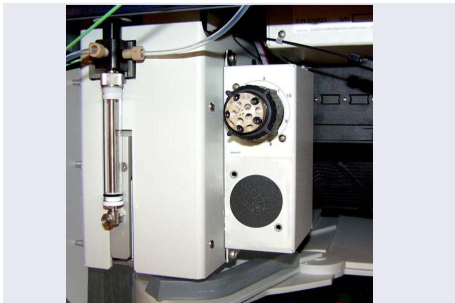
**Figure C-2.** *Optional Valve Installed in the Dionex AS-AP
