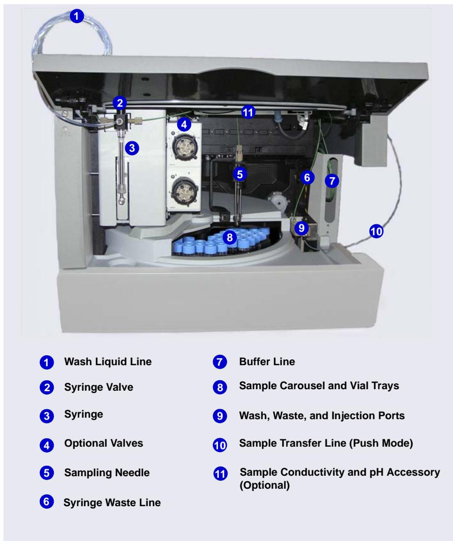
**Figure 2-2.** Dionex AS-AP Front View (Front Panel Lifted)
