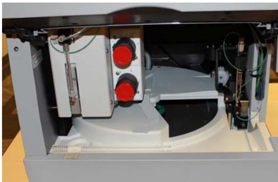
**Figure 3-16.** *Carousel Cover in Correct Position for Installing Foam Insert*
