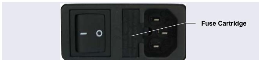
**Figure 5-49.** Dionex AS-AP Fuse Cartridge
