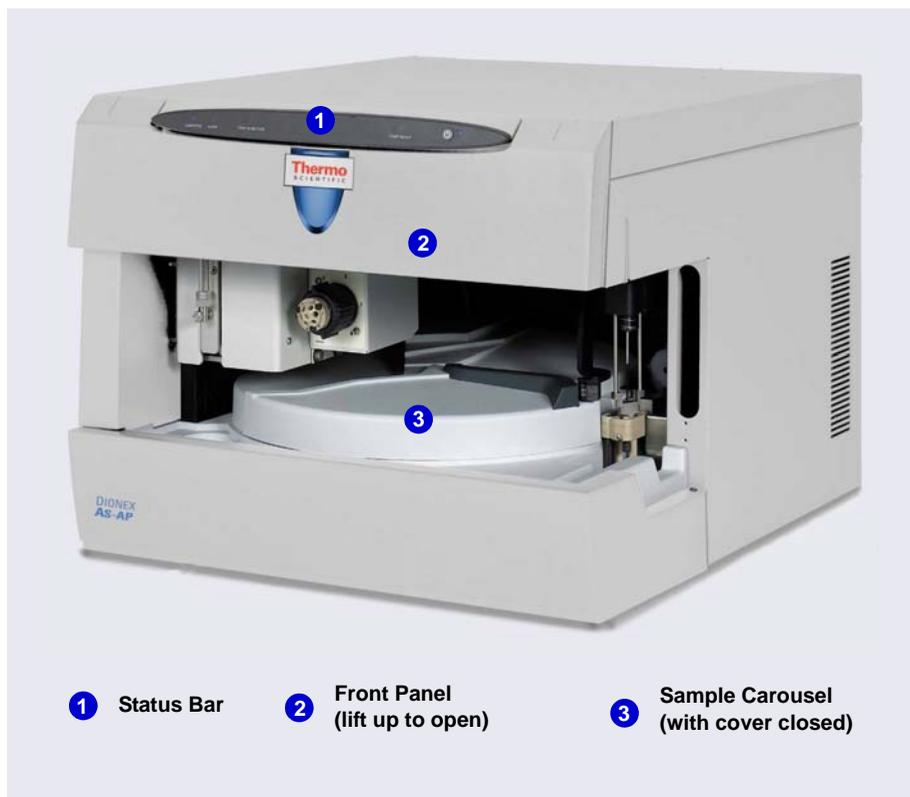
**Figure 2-1.** *Dionex AS-AP Front View (Front Panel Closed)*
