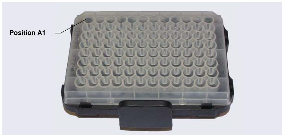
**Figure 3-4.** Well Plate Installed on a Sample Tray
