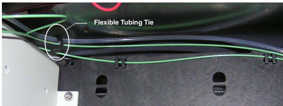
**Figure 5-36.** Flexible Tubing Tie Inside the Dionex AS-AP
