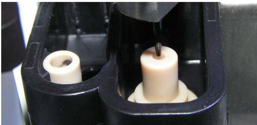
**Figure 5-8.** Needle Centered Above the Injection Port
