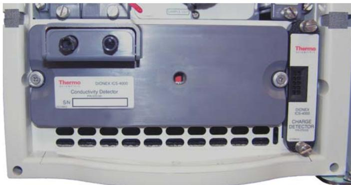
7. Reinstall the Dionex QDC 300 (Capillary) and reconnect all tubing. Close the compartment door.
