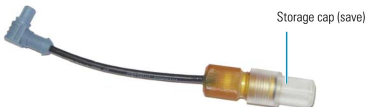
**IMPORTANT** Always store the electrode in the storage cap filled with saturated KCl solution when the cell is not in use. This prevents the pH-Ag/AgCl reference electrode membrane from drying out and damaging the electrode. For storage instructions, see [page 48](#).
