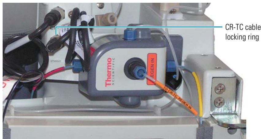
4. Disconnect the liquid lines from the four ports on the CR-TC.
