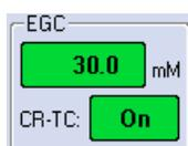
The EGC controls on the Home screen display the eluent concentration currently being generated. If the EGC is not operating, **Off** is displayed and the background of the box is red. The status of the CR-TC (**On** or **Off**) is also displayed. To control the EGC and CR-TC, go to the Electrolytics screen (see Figure v).
