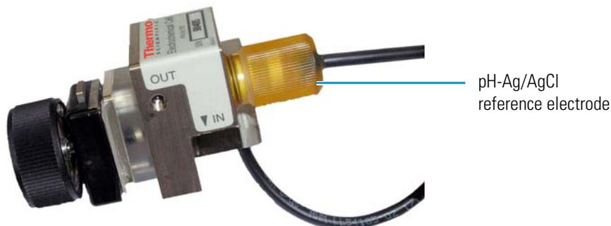
4. Unscrew the storage cap from the new pH-Ag/AgCl reference electrode (see [Figure 99](#)). Save the cap.
