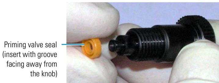
**IMPORTANT** Do not use a sharp tool (such as tweezers) to install the seal. This may scratch the seal and the surface of the priming valve knob. These scratches will prevent a proper seal and cause leakage.
