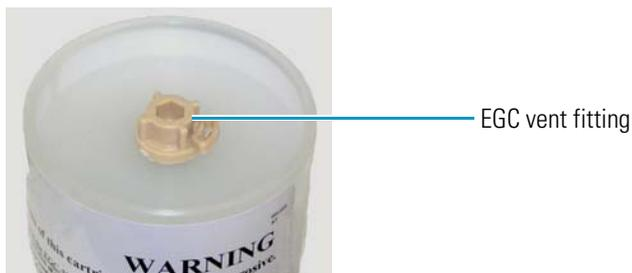
5. Lift the EGC straight up and then slide it forward to remove it from its holder.
