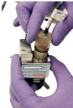
6. Start the pump flow. Wait until liquid is flowing out of the cell inlet line and then reconnect the tubing to the ED cell inlet port. Wait about 1 minute before tightening the connection fully.
