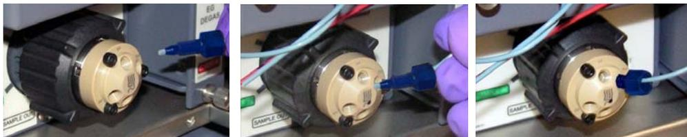
3. While maintaining pressure on the tubing to keep it in place in the port, tighten the fitting bolt fingertight and then tighten the fitting further by following the instructions in [“Ferrule Fitting Guidelines.”](#)
