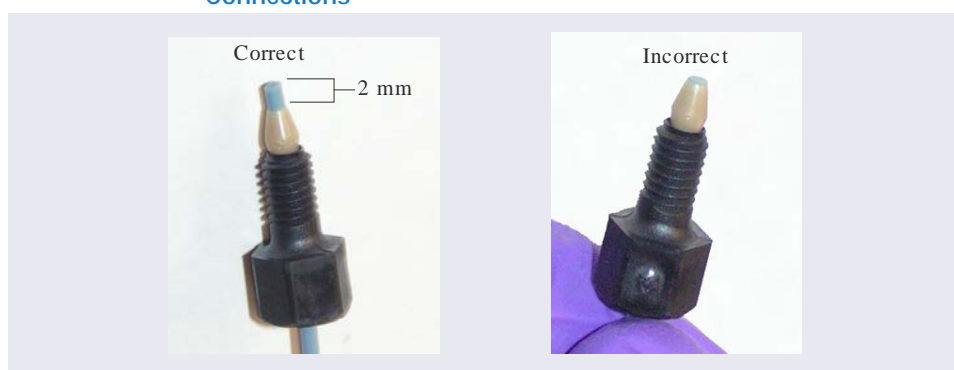
Figure 27. Correct and Incorrect Ferrule and Fitting Bolt Placement for Capillary Tubing Connections
