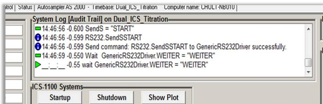
**To troubleshoot:** Check the Audit Trail. If Chromeleon received a truncated response (for example, “WEIT” instead of “WEITER”) increase the wait time from the default value of 200 ms to 500 ms in the device configuration properties of the Generic RS232 driver (see Figure 13).
