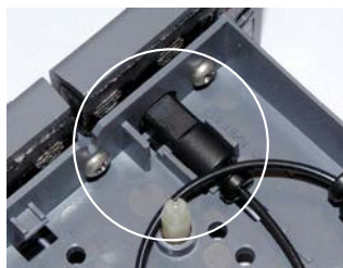
Figure 23 Column Outlet Fitting Installed in Column Cartridge
