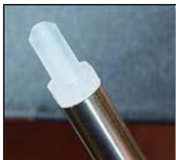
12. Continue threading the free end of the tubing up through the sampling head and out the aperture on the front of the Dionex AS-DV.
