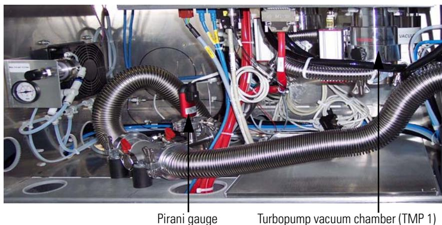
**Figure 1-16.** Vacuum components on the left instrument side
