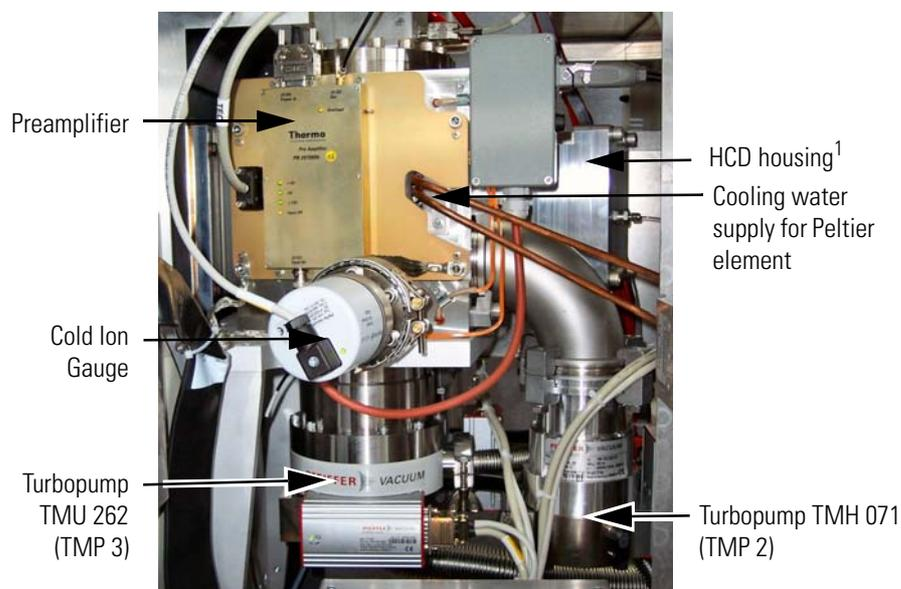
**Figure 1-17.** Vacuum components on the right instrument side
