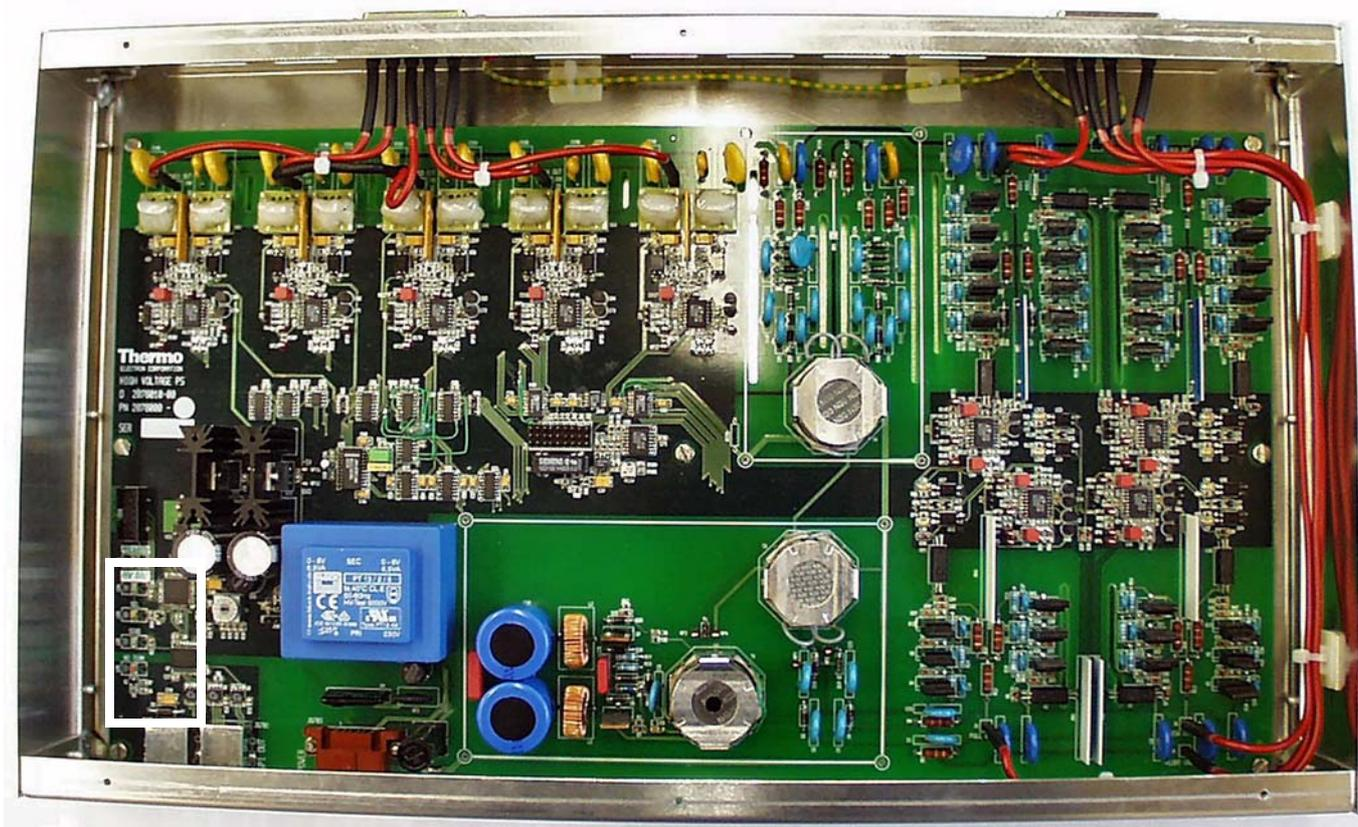
**Figure 1-38.** High Voltage Power Supply board (cover removed)
