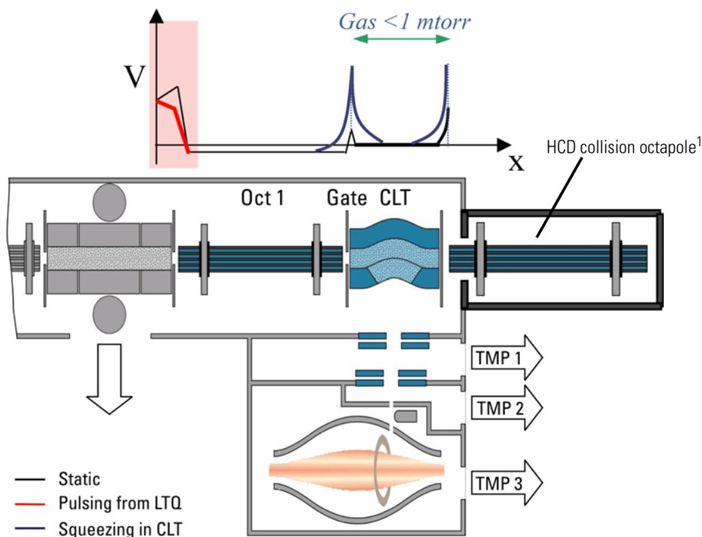
Figure 1-11. Layout of the instrument, also showing the applied voltages
