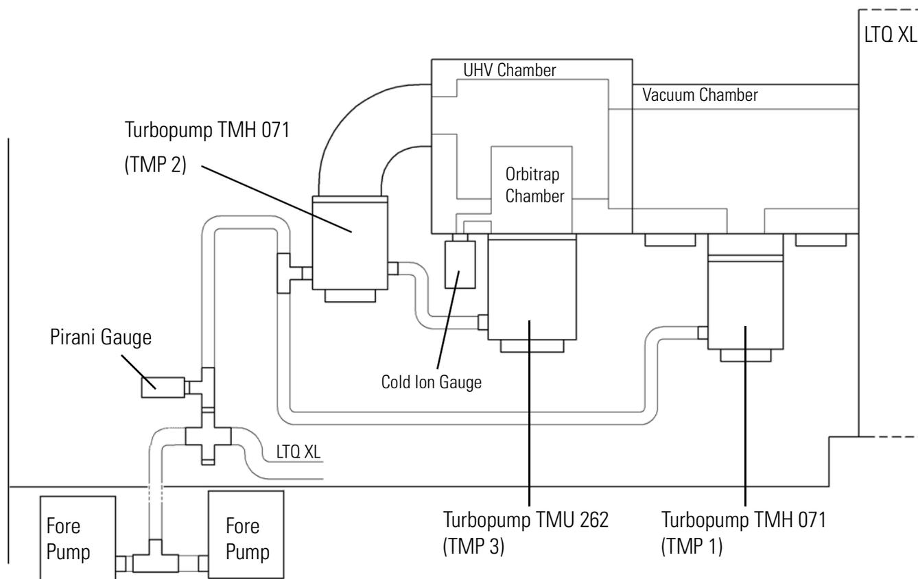
**Figure 1-15.** Schematical view of vacuum system (C-Trap compartment not shown)\*
