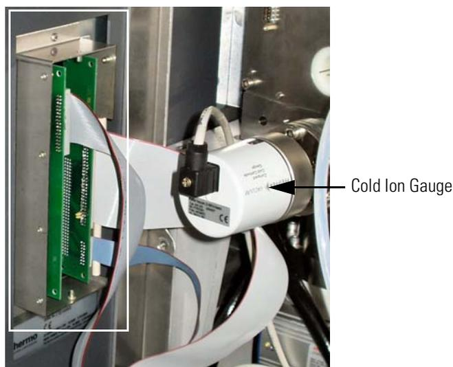
**Figure 1-23.** Electronic connections to linear trap (covers removed)
