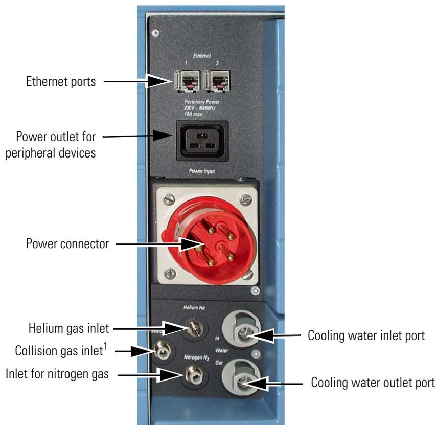
**Figure 1-9.** External connections to the LTQ Orbitrap Discovery
