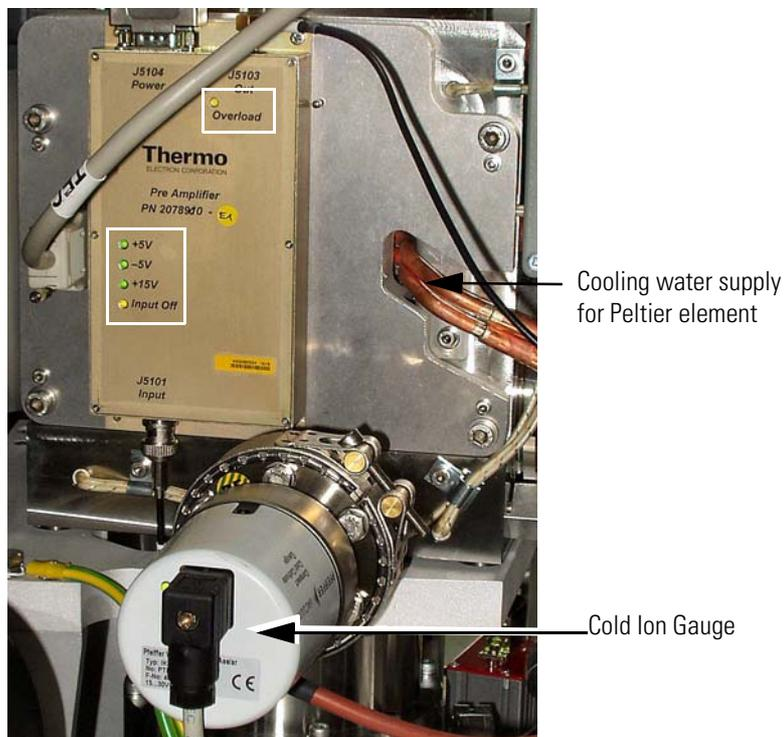
**Figure 1-25.** Preamplifier board
