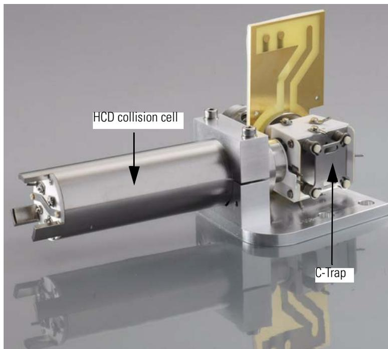
**Figure 1-14.** HCD collision cell and C-Trap
