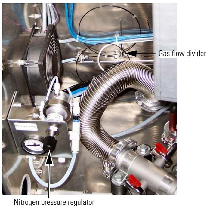
**Figure 1-21.** Nitrogen pressure regulator and gas flow divider
