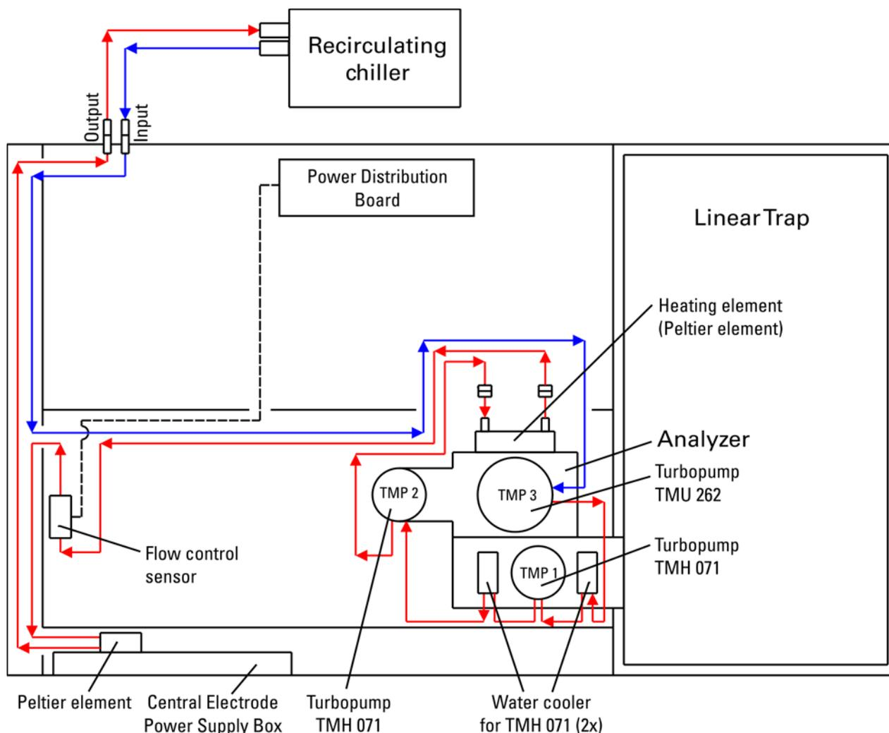
**Figure 1-22.** Schematical view of cooling water circuit\*
