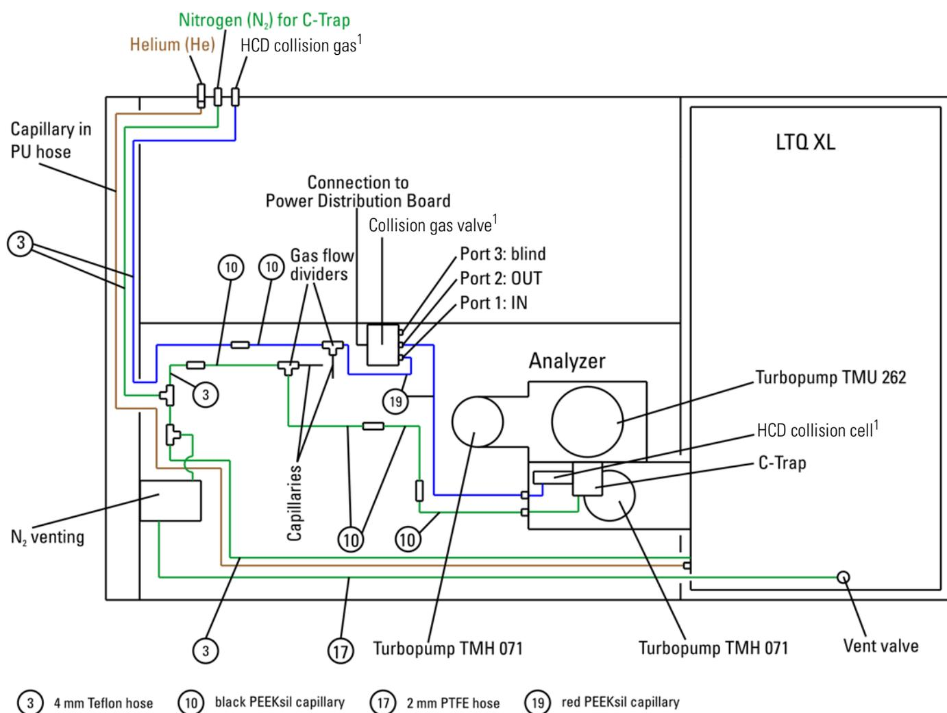
**Figure 1-19.** Schematical view of the gas supply\*
