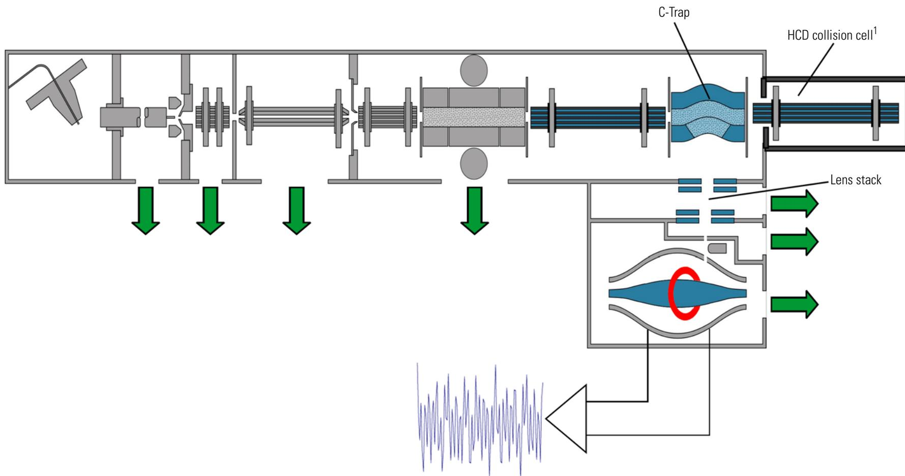
**Figure 1-2.** Schematic view of the LTQ Orbitrap Discovery
