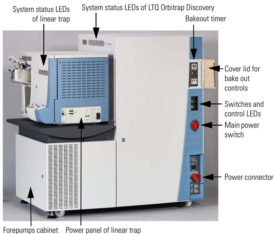
**Figure 1-5.** Right side of the LTQ Orbitrap Discovery
