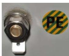
The side panel is connected to the instrument frame by two green/yellow ground wires. See bottom of Figure 1-24. The connectors on the panel are labeled with green-yellow PE (for **P**rotective **E**arth) signs. See photo left. Do not forget to reconnect them before closing the panel!
