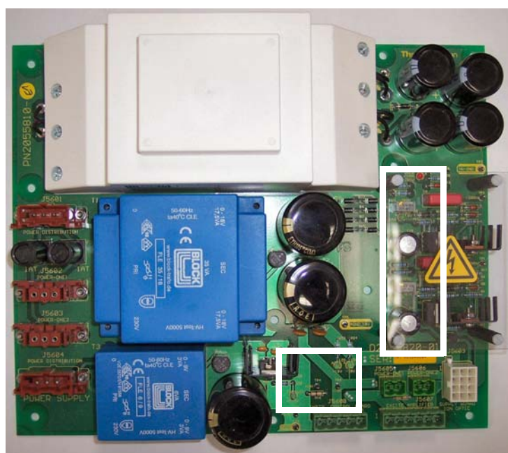
Figure 1-42. Power Supply 1 board
