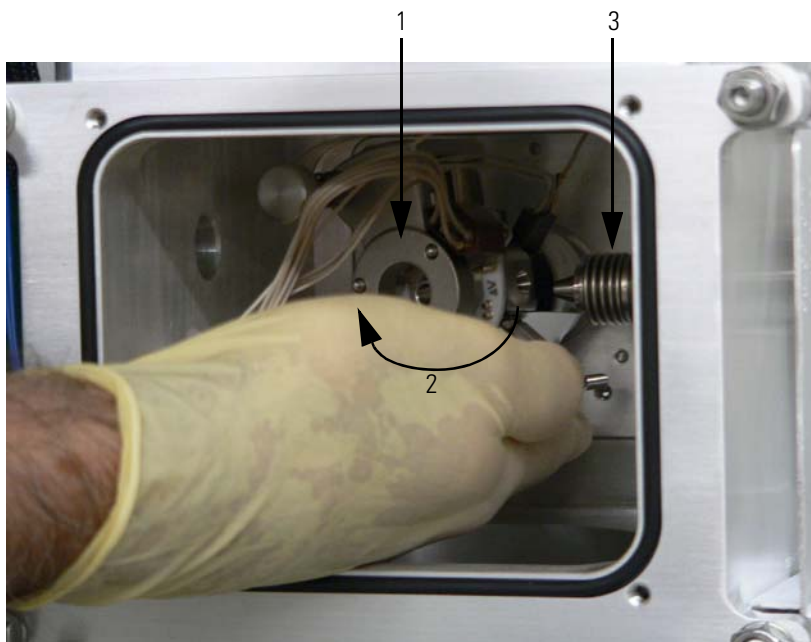
Figure 3-33. Removing the ion source assembly from the vacuum manifold*
