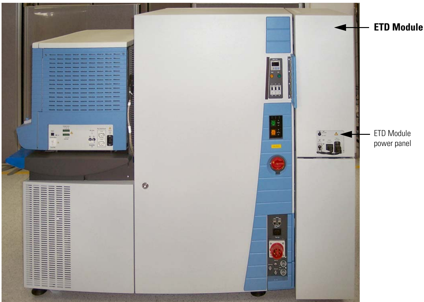
Figure 1-19. Right side of the LTQ Orbitrap Velos ETD
