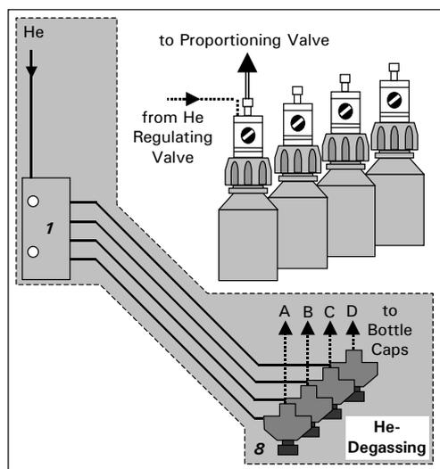
FIGURE 3-2. Solvent Bottle Assembly and He-Degassing Unit
