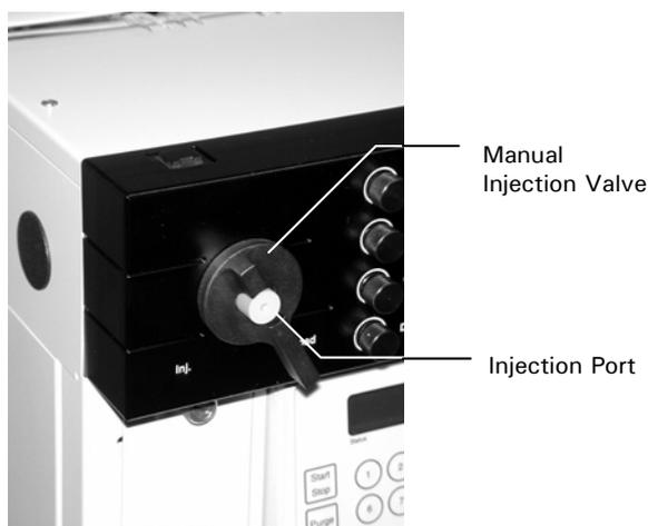
FIGURE A-5. The Manual Injection Valve
