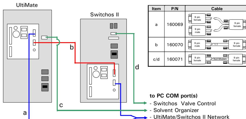
FIGURE A-2. Setting up the RS-232 Connections - UltiMate and Switchos
