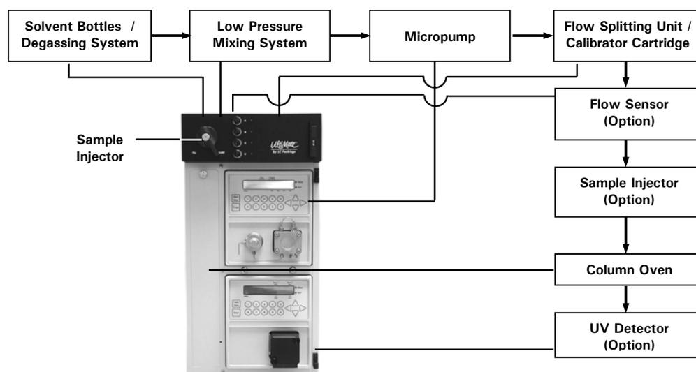
FIGURE 1- 1 Schematic Design - UltiMate System
