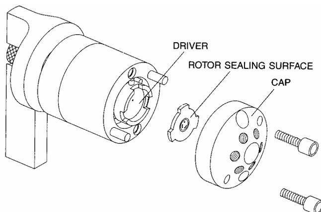
FIGURE D-1 Exploded View of the Valco Model C1 Valve
