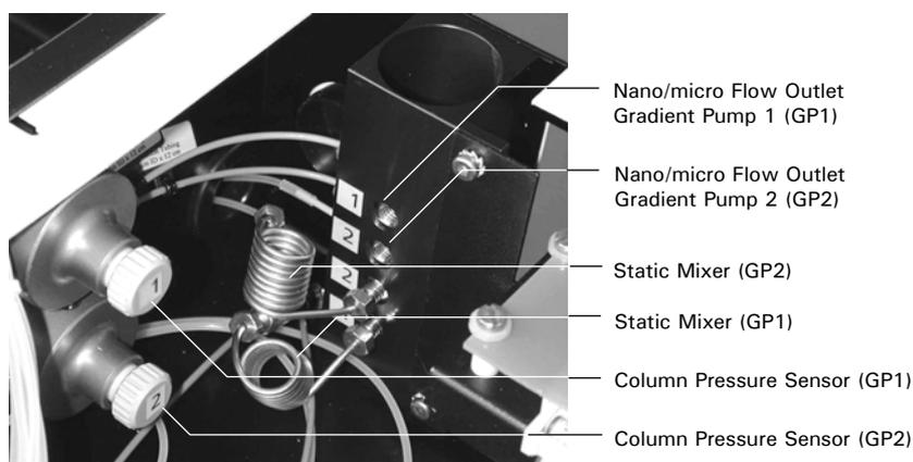
FIGURE B-7 The Nano/micro Flow Outlets of the two Gradient Pumps
