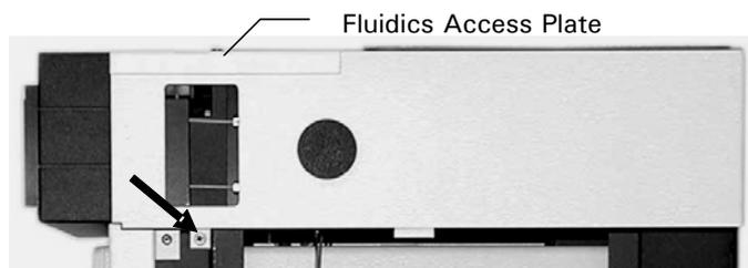
FIGURE 3-23. Removing the Top Cover (Side Panels removed)
