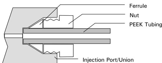
FIGURE C-3. PEEK tubing with Nut and Ferrule
