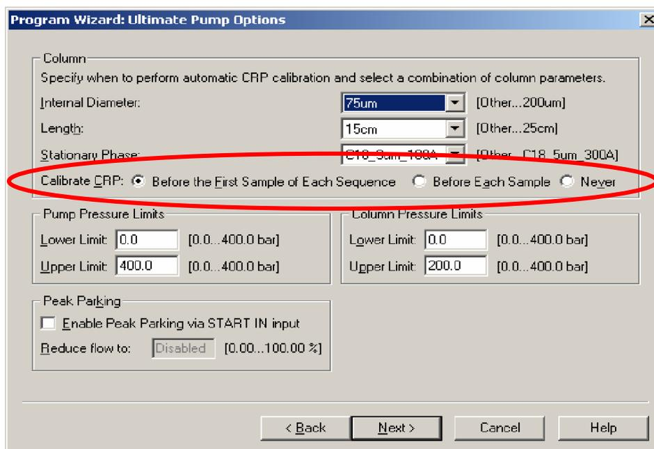
FIGURE A-18. Flow Sensor Setting in the UltiMate Pump Options Box.
