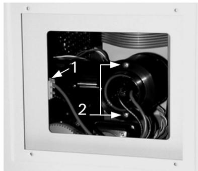
FIGURE 3-17. Accessing the D2 Lamp
