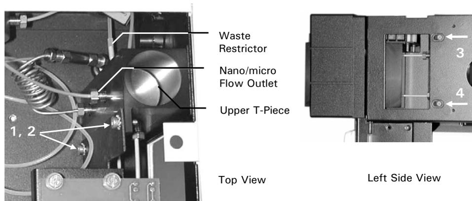
FIGURE 3-25 Removing the T-Piece Assembly
