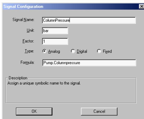
FIGURE 2-26 Virtual Channel Setup for Column Pressure Readout
