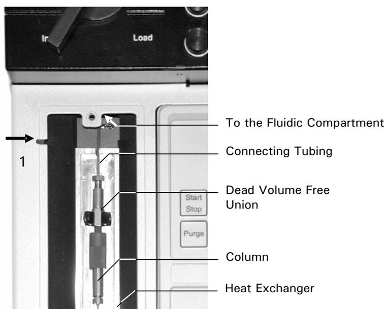
FIGURE C-1. Installing of a 180 µm – 800 µm Column in the UltiMate Oven
