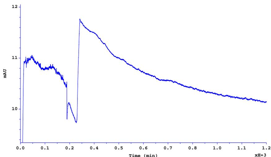
FIGURE 5-15. 24h Drift and Noise Test - Results
