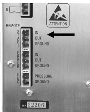
FIGURE A-8. START IN Port on the Micropump
