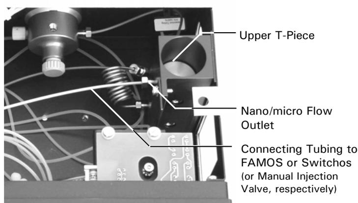
FIGURE 2-6 The Nano/Micro Flow outlet of Solvent Organizer
