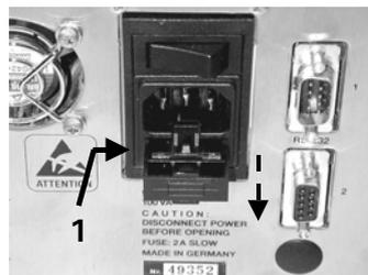
FIGURE 5-20. The Fuse Compartment
