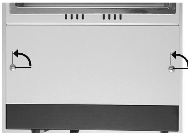
FIGURE 3-18. Removal of Fluidics Access Plate
