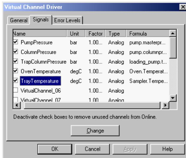
FIGURE 2-27 Example for a typical Virtual Channel Setup
