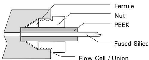
**FIGURE C-5. Using a PEEK Sleeve**
