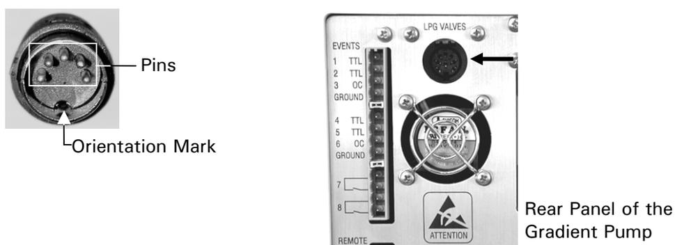
FIGURE B-6 Connector Plug to Solvent Organizer Module
