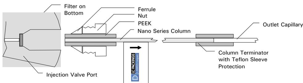
FIGURE C-6. Installation Inlet Filter/Nano Column
