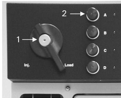
FIGURE 3-24. Manual Injection Valve
