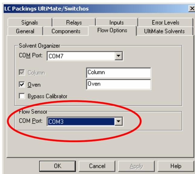
FIGURE A-17. CHROMELEON Server Configuration for the Flow Sensor
