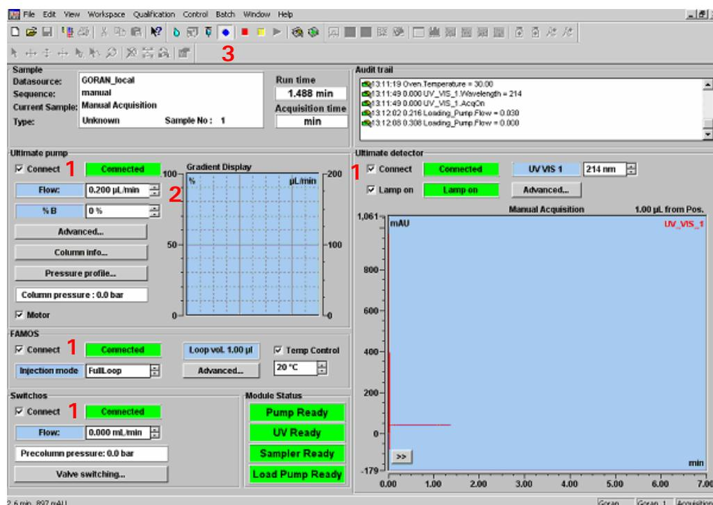
FIGURE 2-28 The Control Panel for UltiMate, FAMOS and Switchos
