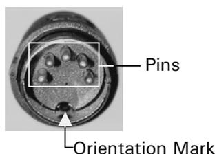
FIGURE 4-6. Connector Plug to Solvent Organizer Module
