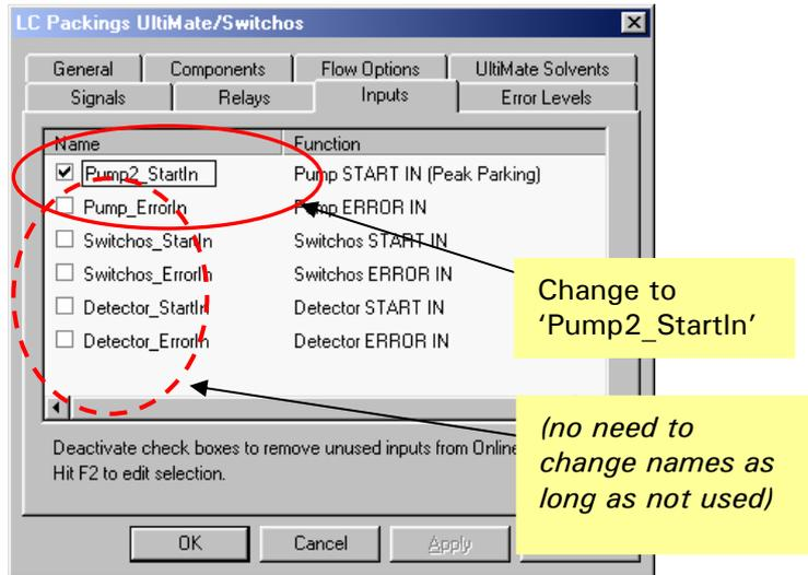
FIGURE B-14 Configuration of the UltiMate/Switchos components
