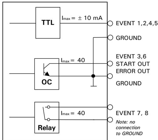
FIGURE 4-5. Output Circuits
