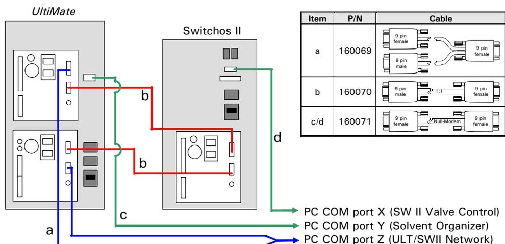
FIGURE 2-8 Setting up the RS-232 Connections - UltiMate and Switchos
