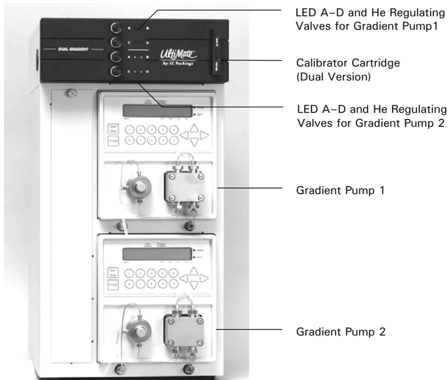
FIGURE B-1 Front View UltiMate Dual Gradient System
