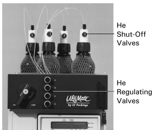
FIGURE 2-40 Solvent Organizer with He Shut-Off Valves and He Regulating Valves
