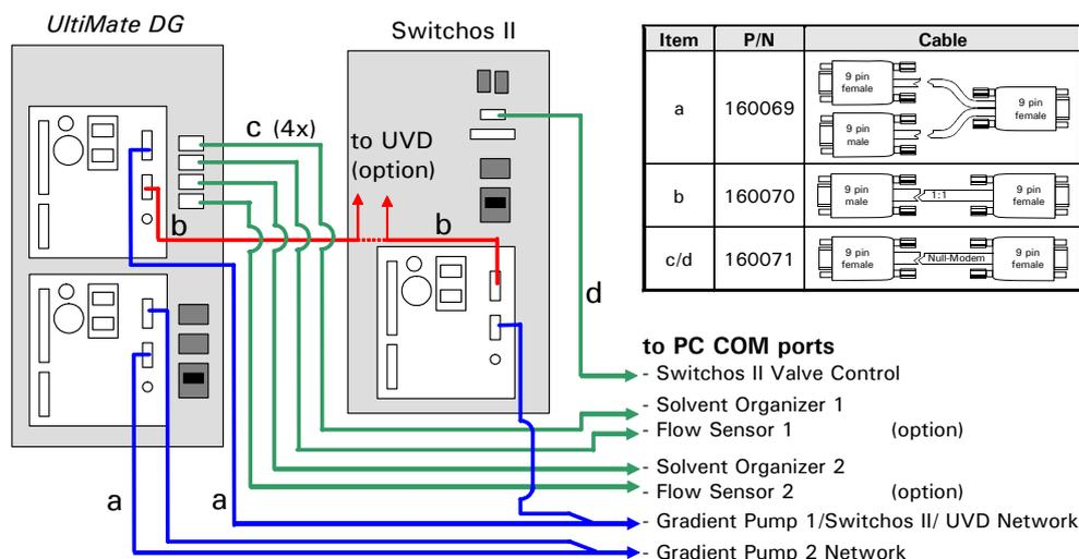
FIGURE B-5 PC Connections of the UltiMate Dual Gradient System (without Flow Sensors)
