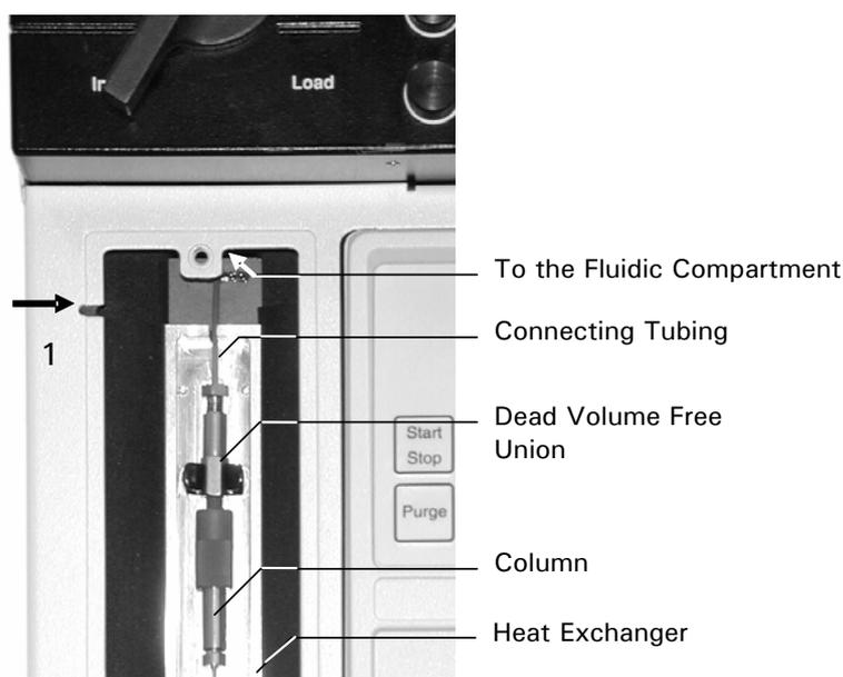
FIGURE 2-43 Installing of a 180 µm – 800 µm Column in the UltiMate Oven
