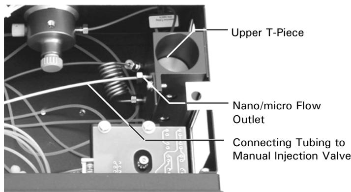
FIGURE A-9. The Nano/Micro Flow Outlet of the Solvent Organizer
