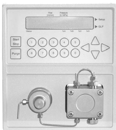
FIGURE 4-1. The UltiMate Micropump
