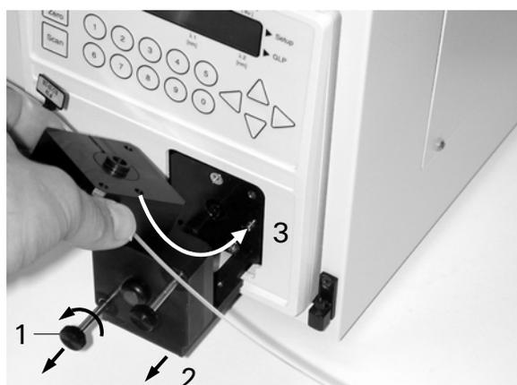
FIGURE 5-4. Cell Region of UV Detector
