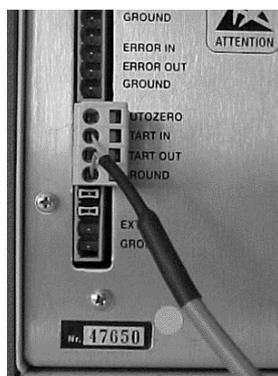
FIGURE A-6. START IN Port on the UV-Detector
