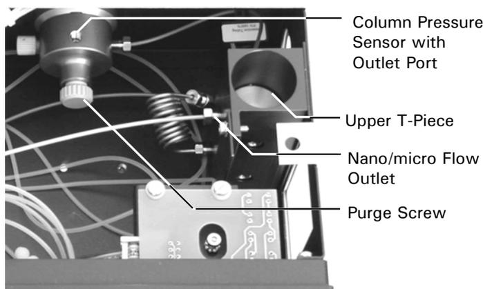
FIGURE 2-42 Purge Valve – Column Pressure Sensor
