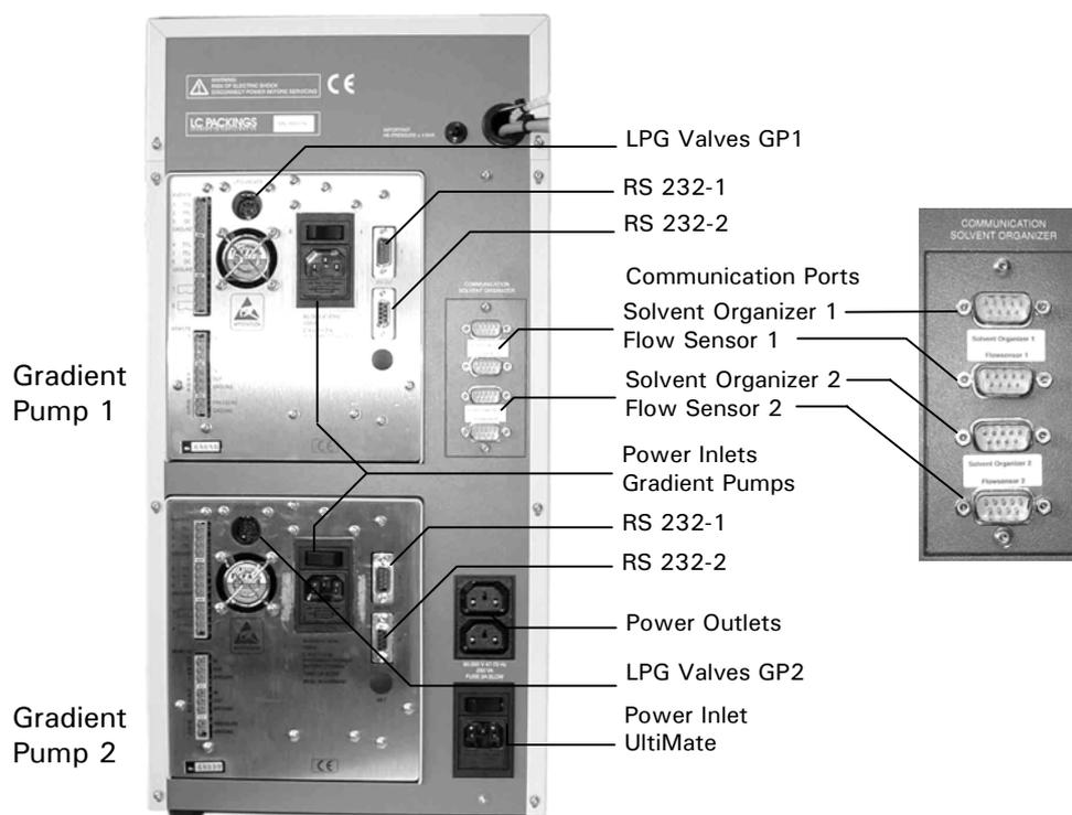
FIGURE B-4 Rear View of the UltiMate Dual Gradient System
