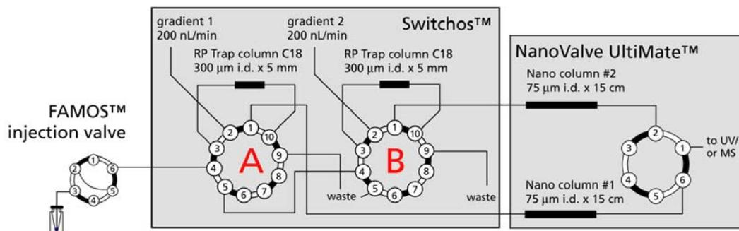
FIGURE B-9 Fluidic Connections for the Parallel Nano-LC Application
