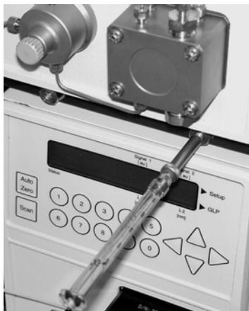
FIGURE 3-30. Placing the Syringe on the Solvent Inlet Line
