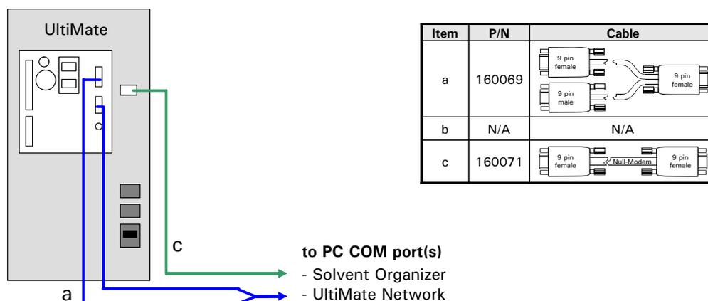
FIGURE A-1. Setting up the RS-232 Connections- UltiMate Micropump
