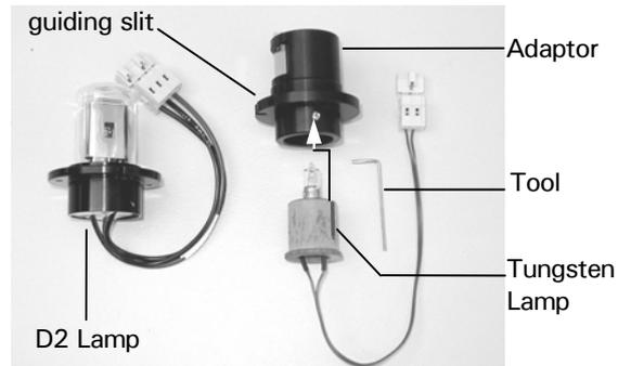
FIGURE 5-19. D2 Lamp/Tungsten Lamp Assembly
