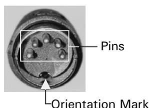
FIGURE 2-3 Connector Plug to Solvent Organizer Module
