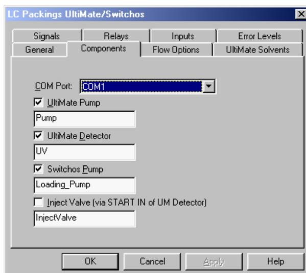
FIGURE 2-22 The UltiMate Configuration Box – Components Tab
