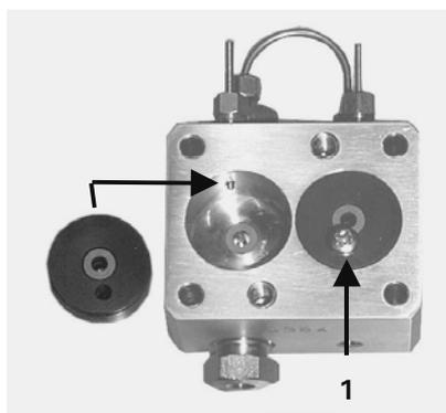
FIGURE 4-17. The Low Pressure Seal Holder
