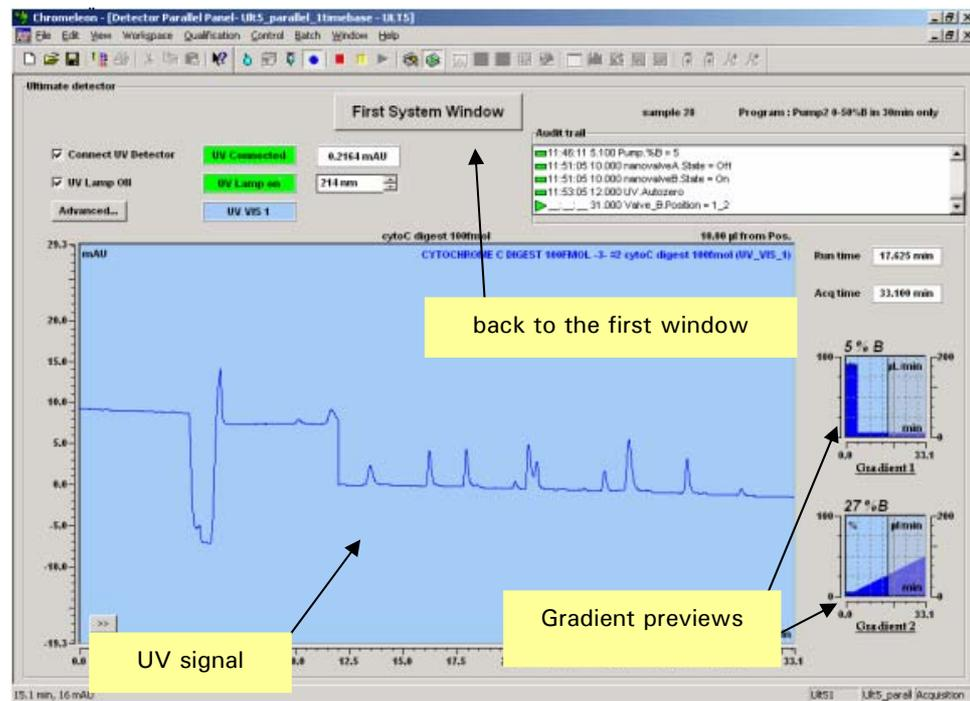
FIGURE B-19 Control Panel for the UV Detector
