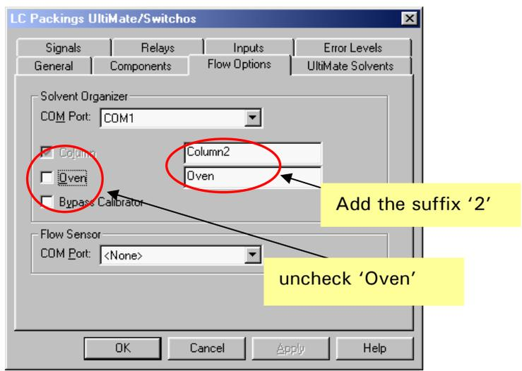
FIGURE B-13 Configuration of the Flow Options Tab
