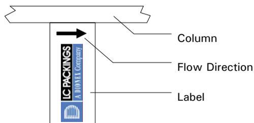
FIGURE C-2. Column Label Indicating Flow Direction
