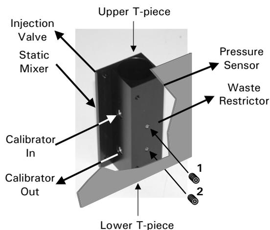
FIGURE 3-26. T-Piece Assembly
