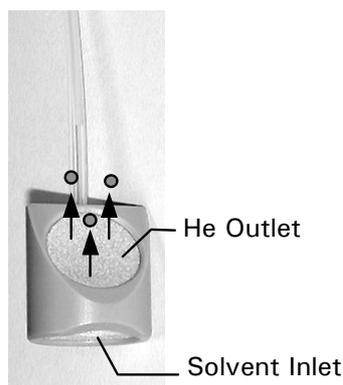
FIGURE 3-4. Sparging/Filter Unit
