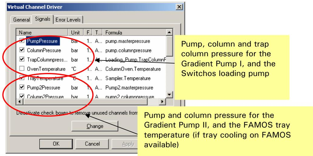
FIGURE B-15 Signals Tab for Virtual Channel Drivers
