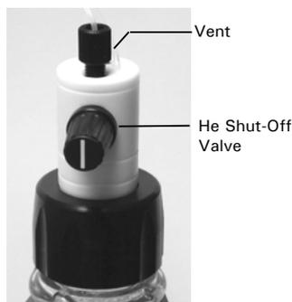
FIGURE 3-29. The He Shut-Off Valve (Opened Position)
