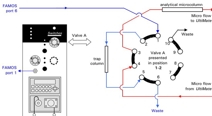
FIGURE 2-9 Typical Pre-Concentration Setup
