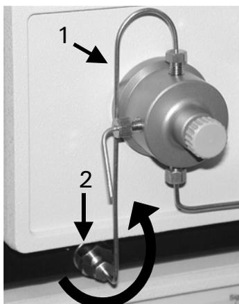
FIGURE 3-14. Tubing - High Pressure Inline Filter
