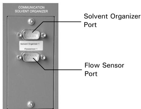
FIGURE A-15. Communication Ports on the Rear Panel
