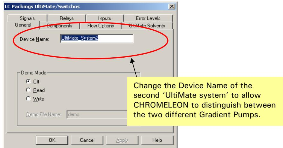
FIGURE B-11 Configuration of the 'LC Packings UltiMate/Switchos#2' Device
