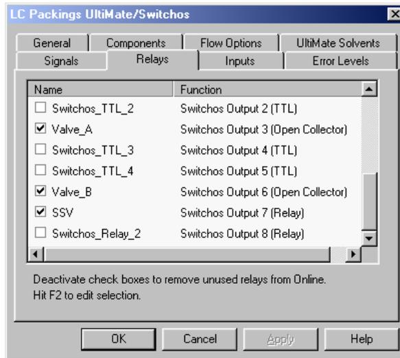
FIGURE 2-23 The UltiMate Configuration Box – Relays Tab
