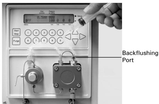
FIGURE 2-39 Filling the Backflushing System of Pump Head
