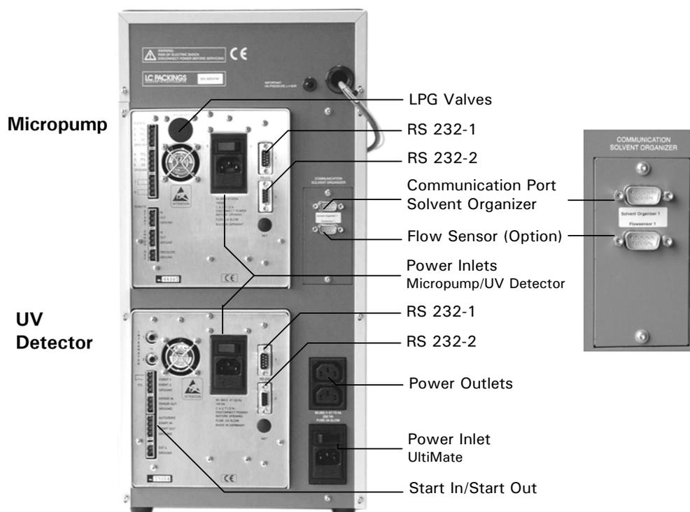
FIGURE 2-1 Rear View of UltiMate with Communication Ports/Power Connections
