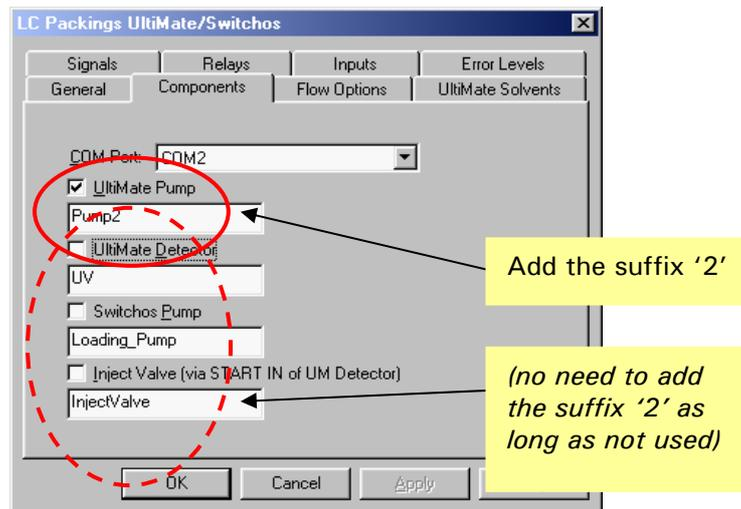
FIGURE B-12 Configuration of the UltiMate/Switchos Components
