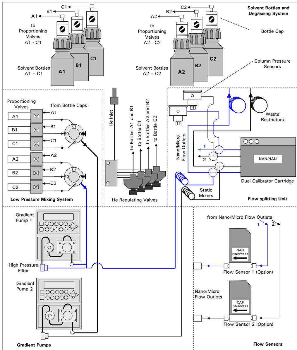
FIGURE B-2 Flow Diagram of the UltiMate Dual Gradient System
