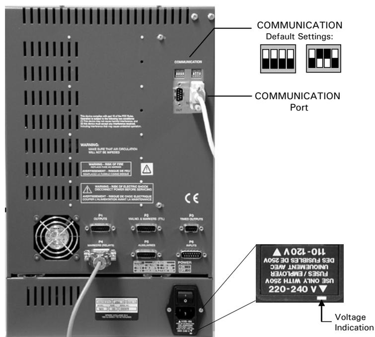
FIGURE 2-7 Rear Panel – FAMOS Autosampler
