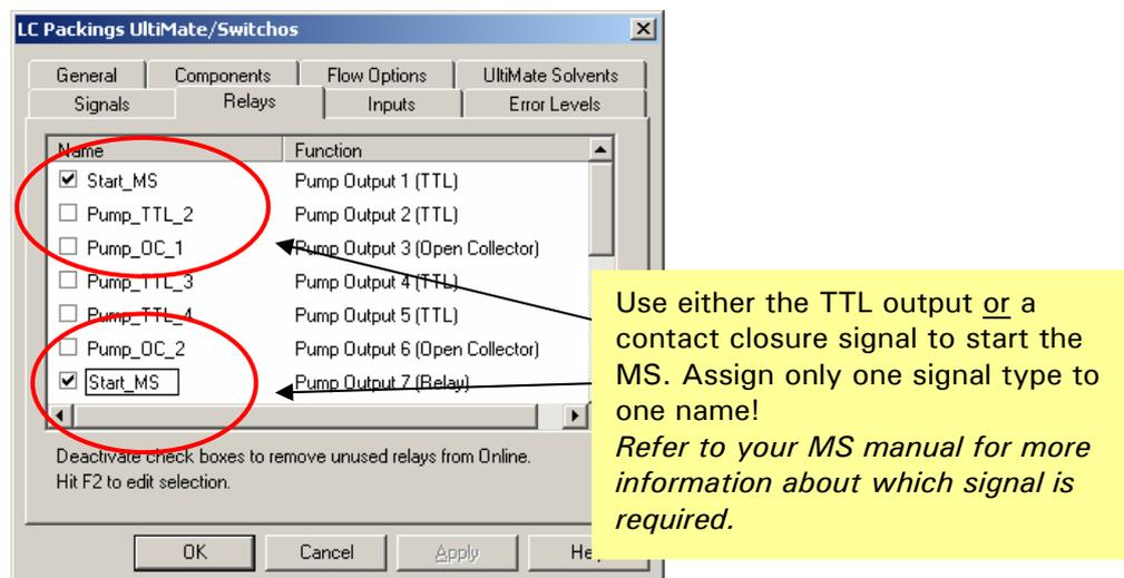
FIGURE B-16 Relay tab with configured Pump Outputs
