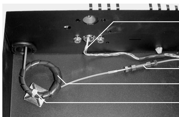
FIGURE 3-27. Waste Restrictor and Union (Solvent Tray removed)
