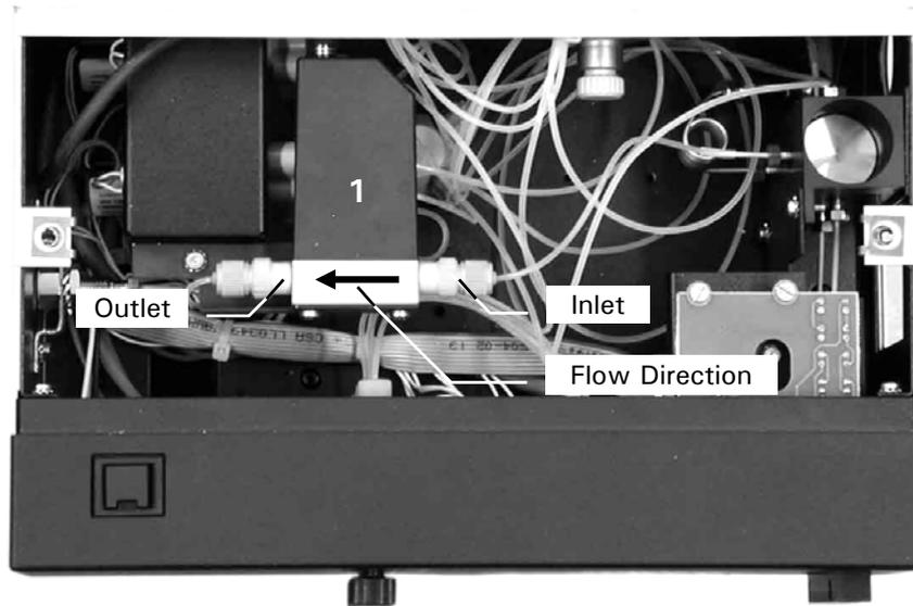
FIGURE A-14. The Fluidic Compartment with the Nano Flow Sensor
