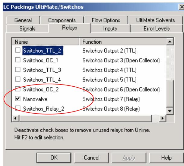
FIGURE B-17 Relay Tab with configured Switchos Outputs
