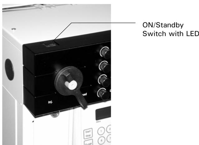
FIGURE 2-38 The ON/Standby Switch
