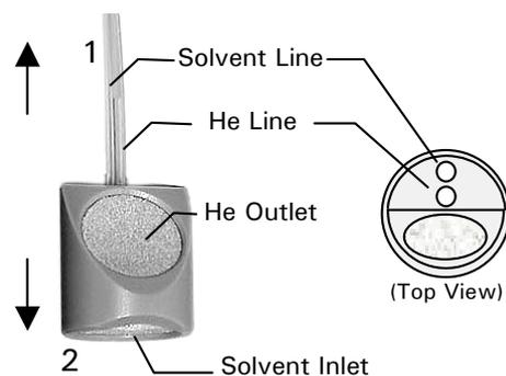
FIGURE 3-13. Sparging/Filter Frit
