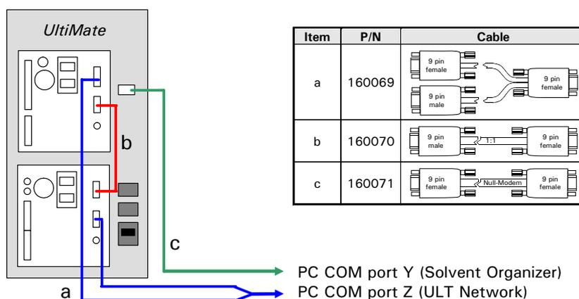
FIGURE 2-2 Setting up the RS-232 Connections – UltiMate
