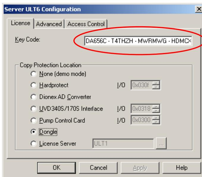
FIGURE 2-15 Server Configuration – Entering the Key Code (using a Dongle)
