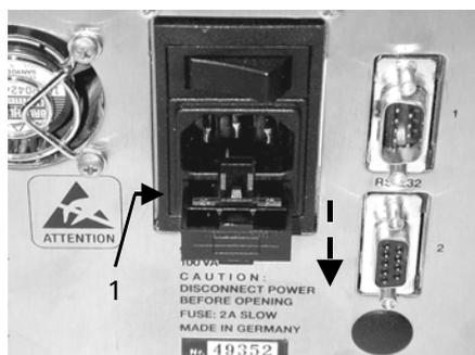
FIGURE 4-21. The Fuse Compartment
