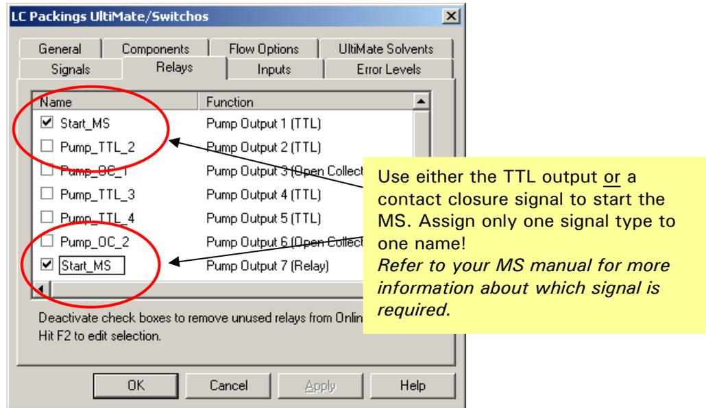
FIGURE B-21 Relay Tab with configured Pump Outputs
