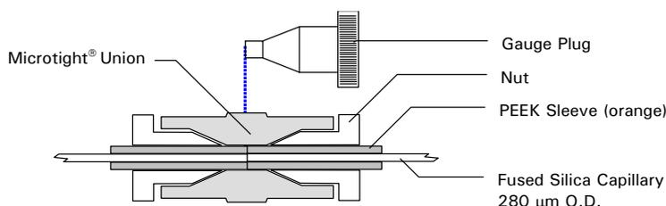
FIGURE C-7. High Pressure Connection using a Microtight union.
