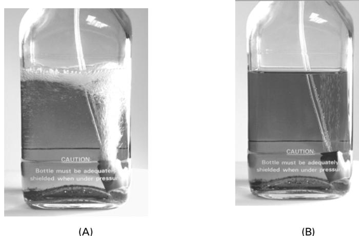
FIGURE 3-7. (A) Rapid Sparging (B) Sparging – Maintenance Mode (Shield removed to provide clarity)
