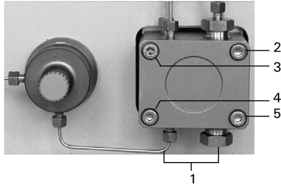
FIGURE 4-14. Disassembly of the Pump Head
