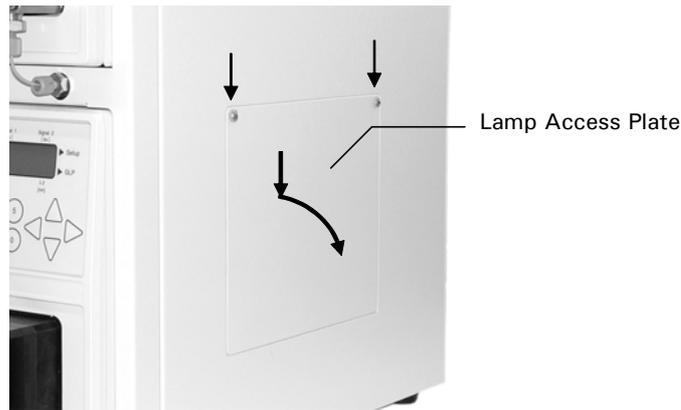
FIGURE 3-16. Removing the Lamp Access Plate
