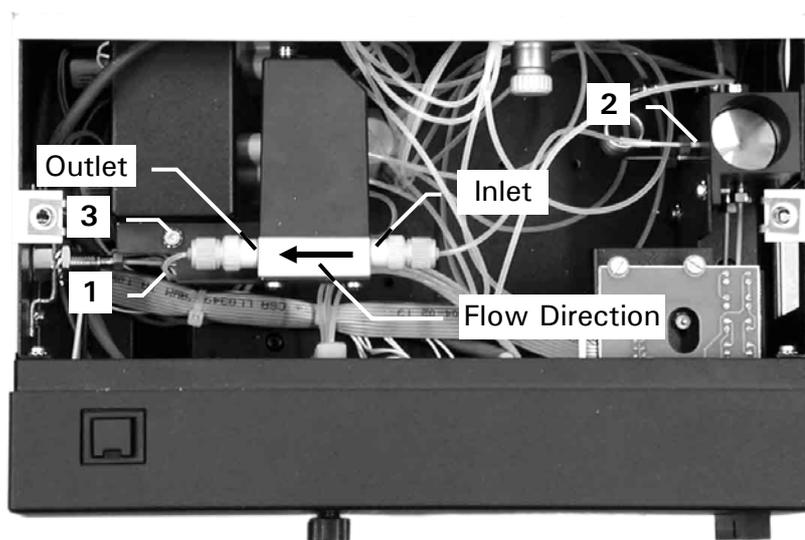
FIGURE A-19. Connecting Tubing of the Flow Sensor
