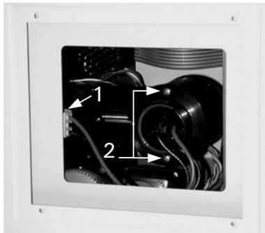
FIGURE 5-18. Replacing D<sub>2</sub> Lamp
