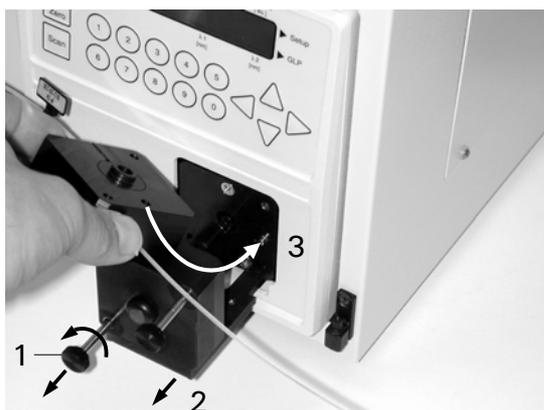
FIGURE 2-5 Installing the Flow Cell
