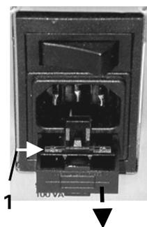
FIGURE 3-28 Fuse Compartment
