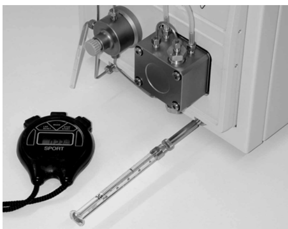
FIGURE 4-12 Placing the Syringe on the Solvent Inlet Line
