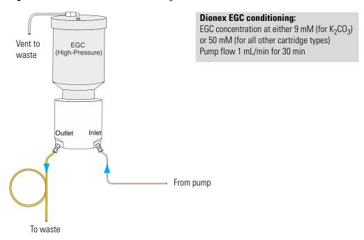
7. Remove the vent fitting or fitting plug and connect the vent line removed from the old cartridge to the vent opening. Save the vent fitting.
