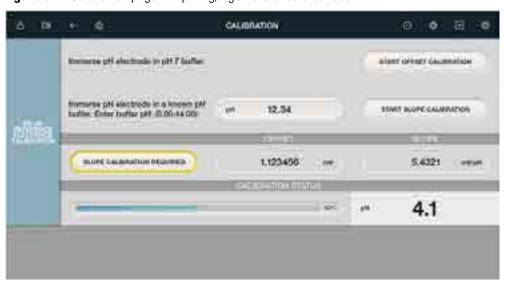
Figure 64. Calibration page: ED pH-Ag/AgCl reference electrode
