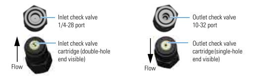
**Note** For correct pump operation, the check valve cartridges must be installed in their respective housings in the correct orientation. Liquid enters through the check valve in the large single hole and exits through the small double holes.
