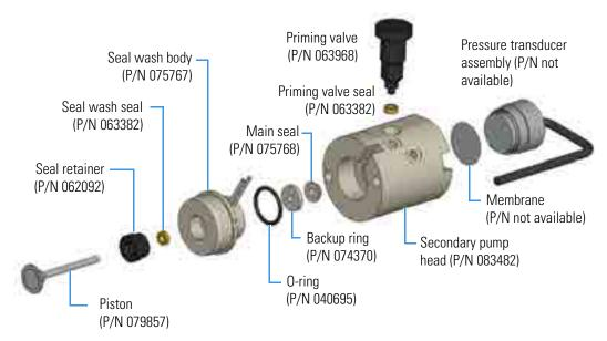
Figure 85. Secondary pump head assembly
