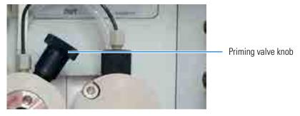
6. Pull the old seal off the end of the priming valve knob.
