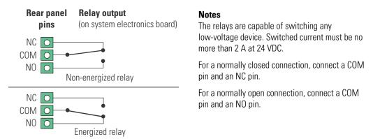
Choose NC or NO based on what you want the state of the connected device to be when the Dionex Integrion power is turned off. A normally open relay is open when the relay is switched off and closed when the relay is turned on. A normally closed relay is closed when the relay is off and is open when the relay is on.
