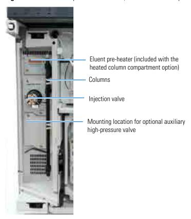
The column compartment is an insulated environmental chamber that can house a guard column, a separator column, an injection valve, and an optional auxiliary high-pressure valve. The compartment protects the housed components from fluctuations in ambient temperature.
