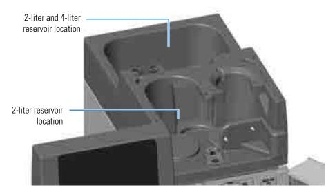
The following reservoirs are available for use with the Dionex Integrion HPIC System:
