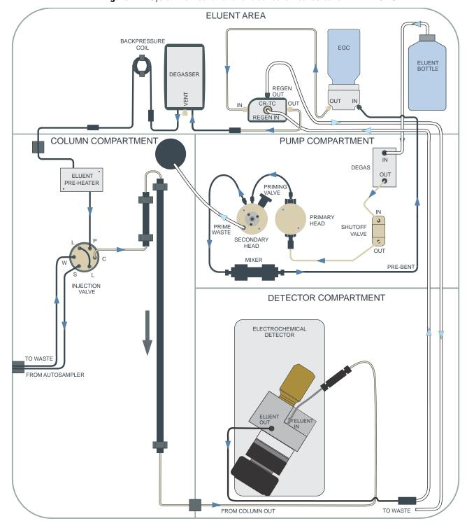
Figure 22. System flow schematic for electrochemical detection with RFIC-EG
