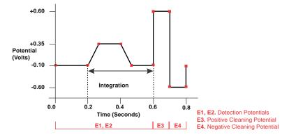
With the example waveform shown in Figure 33, the current is integrated both while the potential is swept across the metal oxide formation wave and also during the reverse sweep across the oxide reduction wave. This technique minimizes baseline shift and the peak dips that can occur when an eluting analyte's effect on oxide suppression is greater than the detector response from the analyte.
