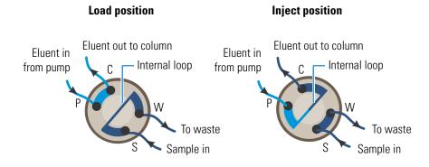
Figure 13. Injection valve flow schematics (6-port valve)
