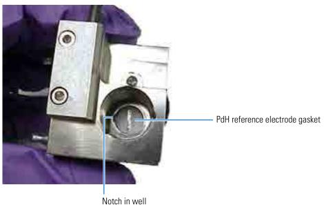
5. Using tweezers, grasp the new PdH reference electrode gasket (P/N 072214) on its edge (see Figure 104). To avoid deforming the gasket cutout, do not place the tweezer tips on the cutout.
