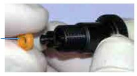
**IMPORTANT** Do not use a sharp tool (such as tweezers) to install the seal. This may scratch the seal and the surface of the priming valve knob. These scratches will prevent a proper seal and cause leakage.
