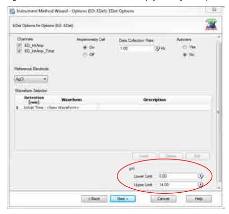
**Note** To disable the alarm, set the upper limit to 14 and the lower limit to 0.
