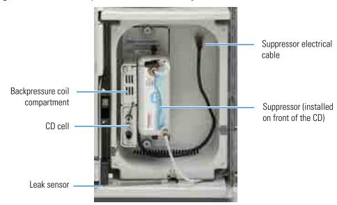
The CD consists of a heated conductivity cell and the electronics required for collecting the conductivity data and sending it to the computer and the analog output.
