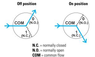
**Note:** When the valve is off (not energized), port 0 is open (N.O.) and port 1 is closed (N.C.). Conversely, when the valve is on, port 1 is open and port 0 is closed.
