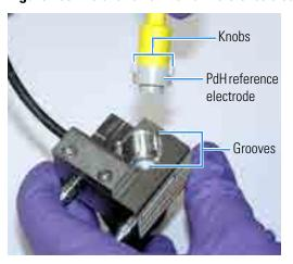
Figure 105. Installation of the PdH reference electrode
