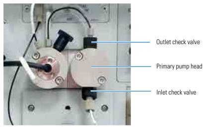
6. Loosen both check valve assemblies, using a 1/2-inch wrench, and remove them from the pump head.
