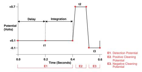
The potentials, labeled E1, E2, and E3, are applied for durations t1, t2, and t3, respectively. At t1, the E1 potential is applied. After a delay, the signal is measured by integrating the current for a fixed time. Current integrated for a fixed time is charge and the units are coulombs. At t2 and t3, positive and negative cleaning pulses are added to the waveform. This waveform period repeats until the end of data acquisition or until another waveform is specified.
