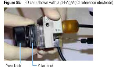
**Note** Handle the cell gasket and the inside surfaces of the cell carefully to prevent scratches, which may subsequently cause leaks.
