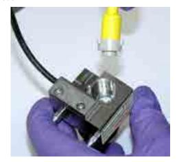
$4. \ \ Using tweezers, remove the PdH \ reference electrode gasket from the well (see Figure 103).$
