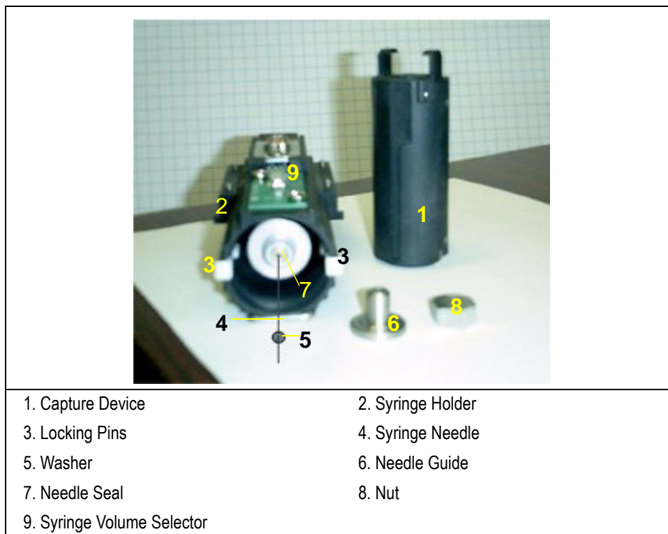
Figure 7-11. Injection Device Assembly
