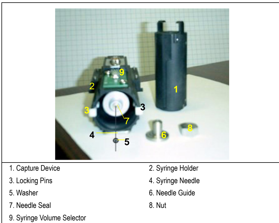
Figure 2-13. HS Injection Device Components
