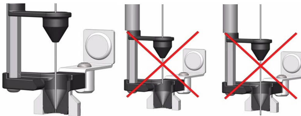
Figure 57. Correct and Incorrect Position of the SPME Needle Tip
