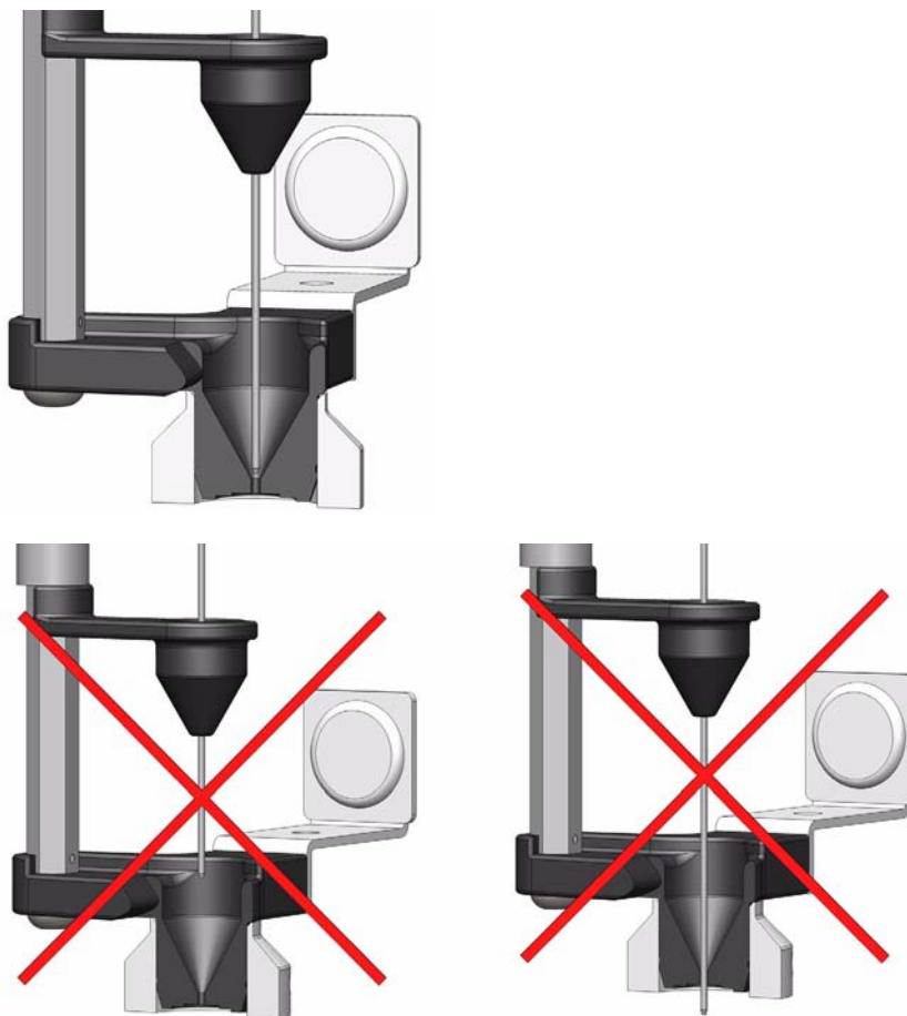
Figure 50. Correct and Incorrect Position of the Syringe Needle Tip
