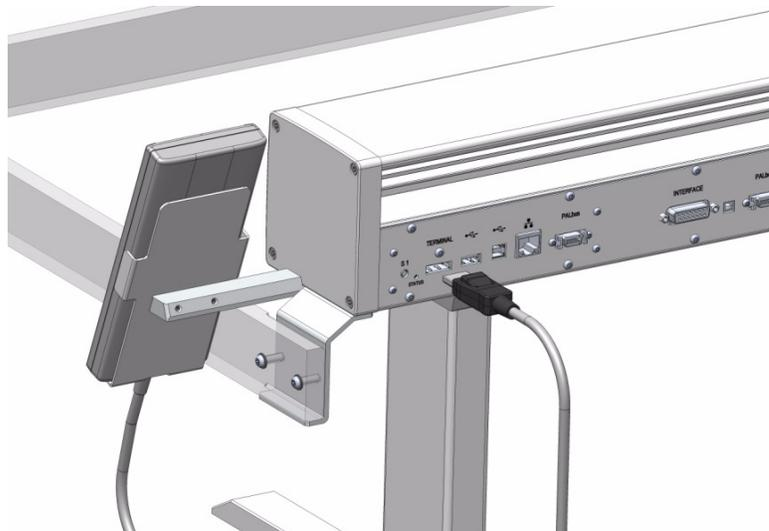
5. Place the Handheld Controller onto its mounting bracket. See [Figure 12](#).
