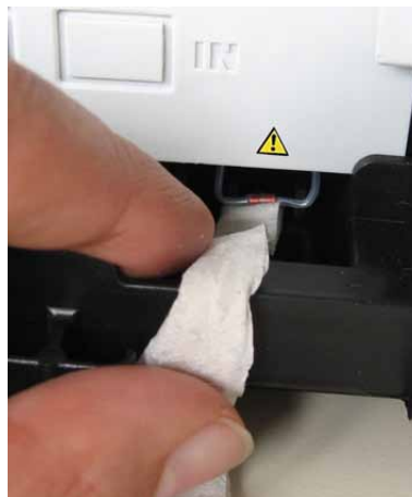
Fig. 13: Drying the leak sensor
