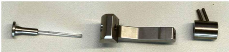
Fig. 59: Holding hook disassembled
