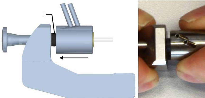
*Fig. 60: Installing the secondary piston seal (1)*
