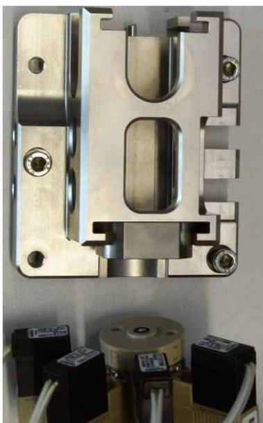
*Fig. 63: Installing the proportioning valve (here with pump head body)*
