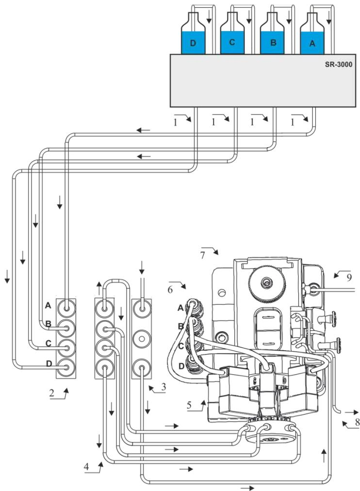
Fig. 5: Flow path through the LPG-3400XRS pump
