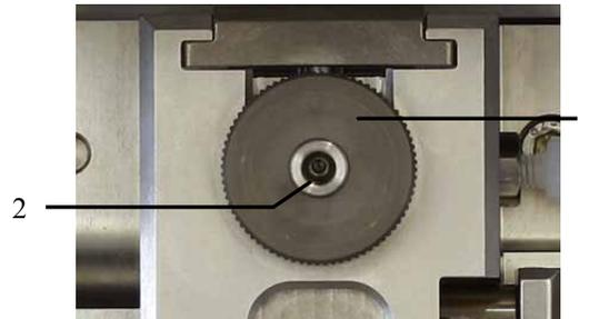
Fig. 10: Purge unit in the pump head
