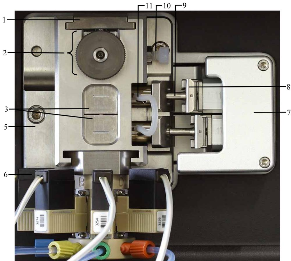
Fig. 39: Pump head with proportioning valve
