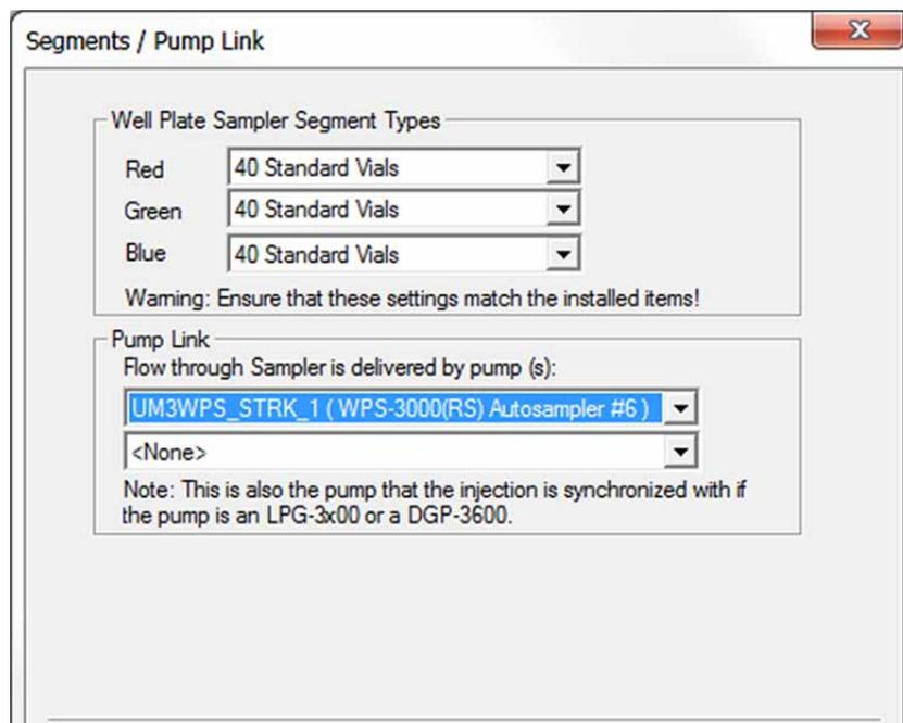
Fig. 35: Segments/Pump Link settings
