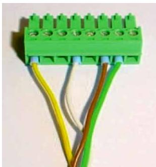
Fig. 19: 8-pin terminal connector on synchronization cable
