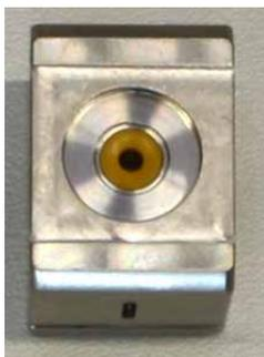
*Fig. 57: Piston seal installed in the displacement chamber*
