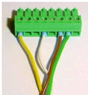
*Fig. 17: 8-pin I/O terminal connector
