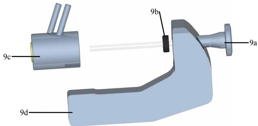
Fig. 42: Holding hook with piston and guide bushing
