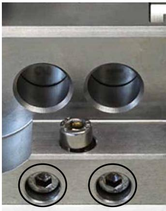
Fig. 46: Clamping screws for holding hooks
