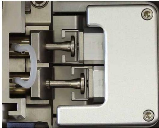
Fig. 44: Pistons without piston retaining springs
