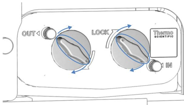
Figure 14: Closing the rotating locks
