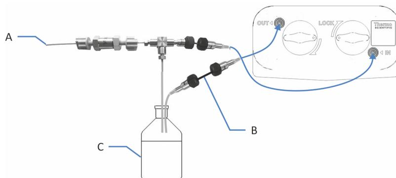
Figure 42: Setup for forward flushing (here: without overpressure relief valve)
