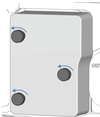
Figure 33: Screws on the lamp house cover
