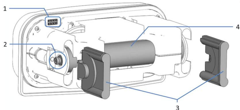
Figure 12: Rear side of the flow cell
