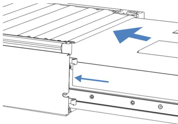
*Figure 47: Inserting the slide-in module*
