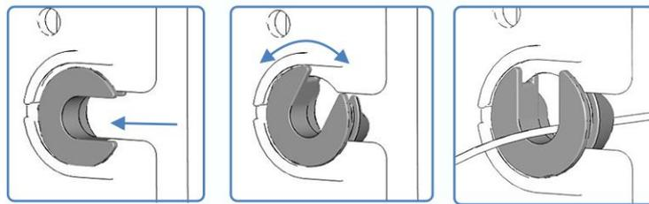
Figure 20: Using the rotating plug
