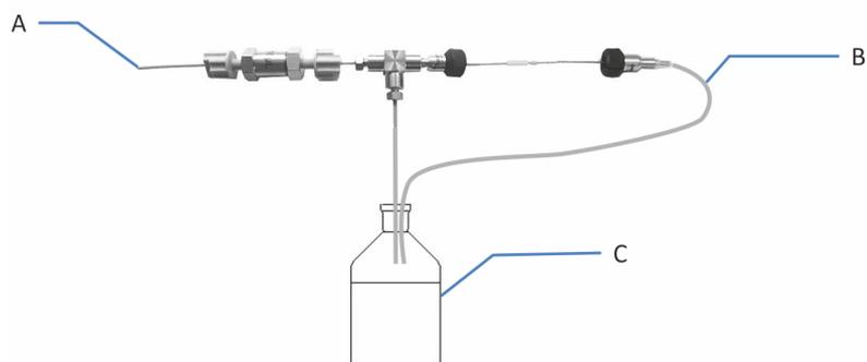
Figure 40: Setup for flushing the T piece
