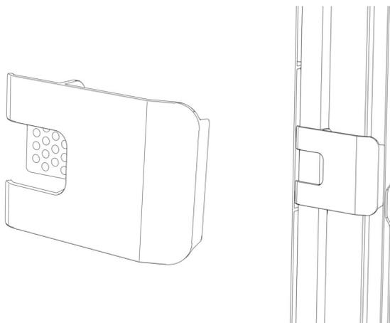
Figure 16: Tubing bracket (left), tubing bracket installed (right)
