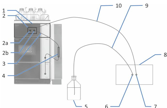
Figure 29: Calculating the pressure at the inlet port of the flow cell in your used system configuration
