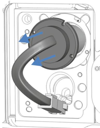
Figure 34: Pulling out the UV lamp
