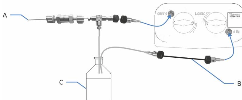
Figure 41: Setup for back-flushing (here: without overpressure relief valve)
