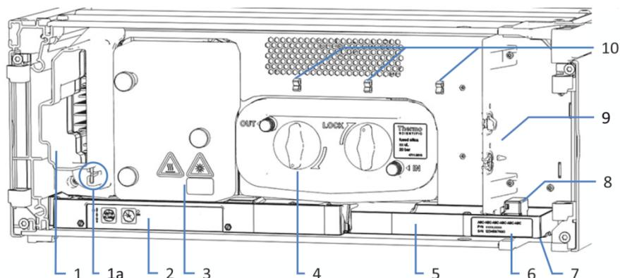
Figure 2: Interior view (here with flow cell installed)
