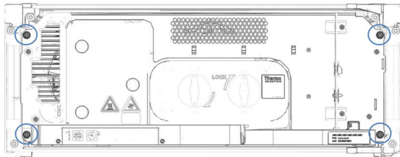
Figure 45: Captive screws on the slide-in module (doors not shown)
