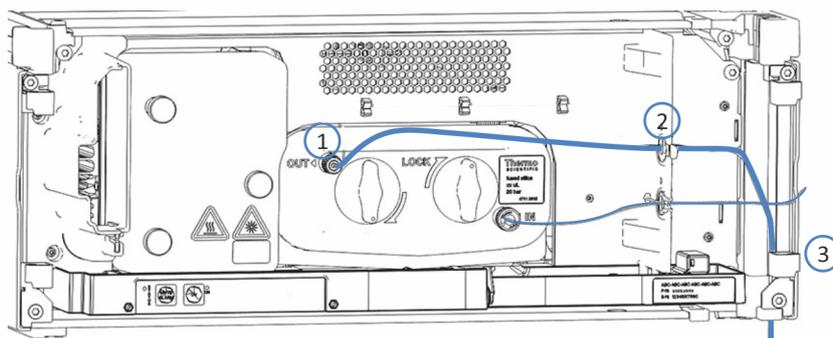
Figure 24: Connecting the detector waste line
