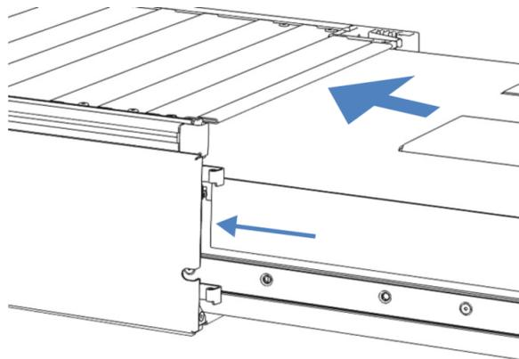
Figure 47: Inserting the slide-in module
