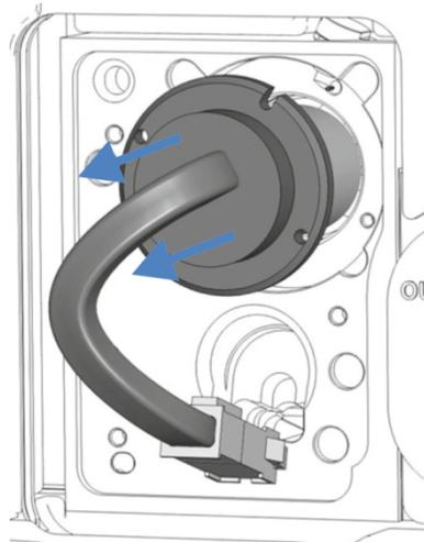
Figure 34: Pulling out the UV lamp
