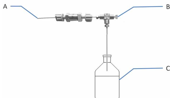
Figure 39: Setup for determining the pump flow
