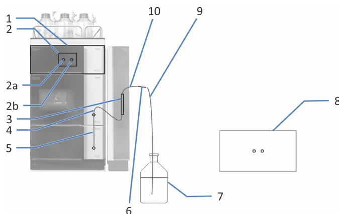
Figure 26: Measuring the Vanquish system backpressure (without flow cell and additional module)
