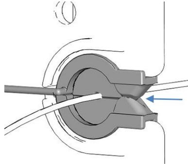
Figure 19: Capillary installed in the plug with slit
