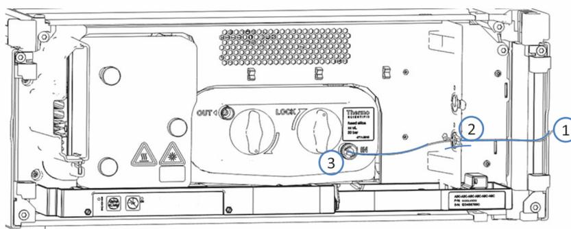
Figure 23: Connecting the inlet capillary from the column compartment (example)
