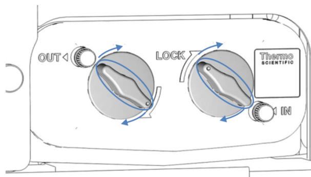
Figure 14: Closing the rotating locks
