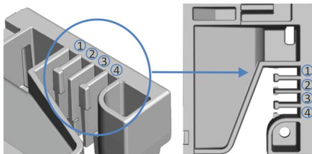
Figure 15: Tubing chase with tubing guides (left: view from inside, right: view from top)
