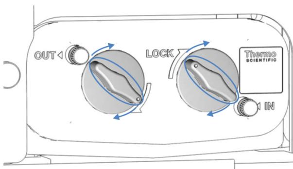
Figure 37: Closing the rotating locks
