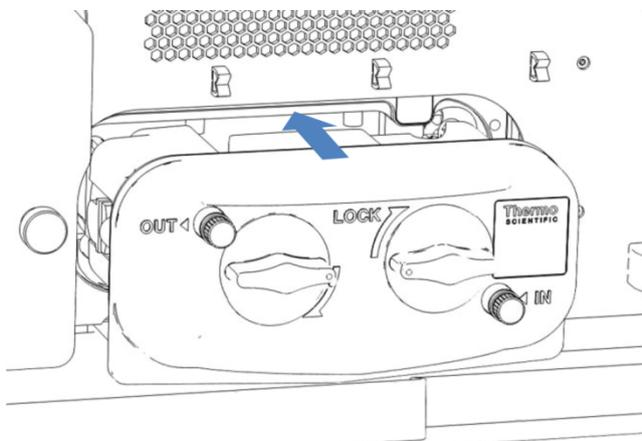
Figure 36: Inserting the flow cell with opened rotating locks
