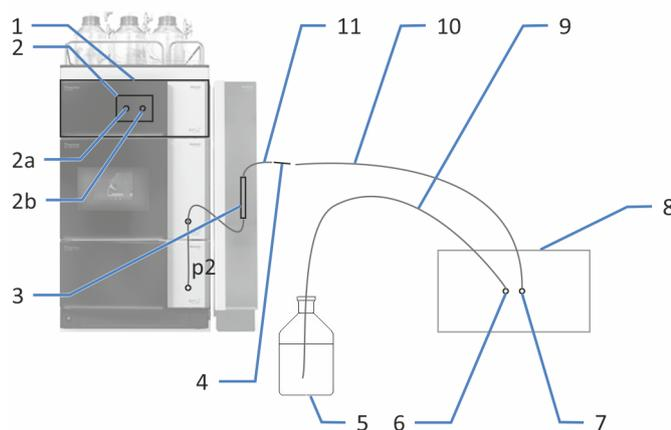
Figure 27: Determining the backpressure of a second detector (example)
