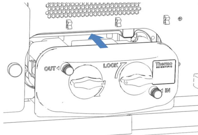
Figure 13: Inserting the flow cell with opened rotating locks
