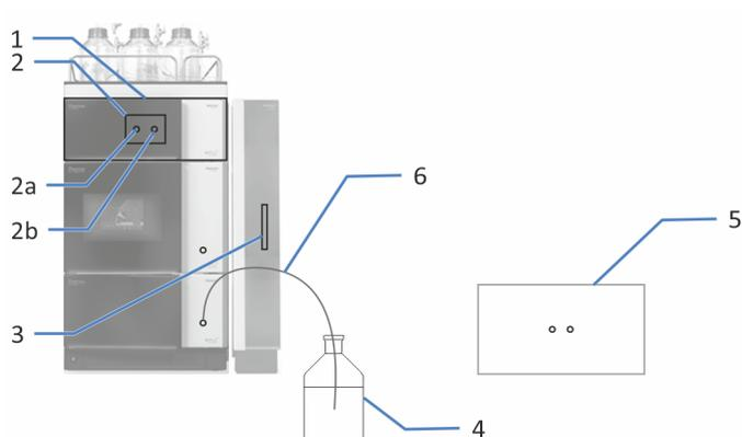
Figure 25: Measuring the backpressure of the waste line
