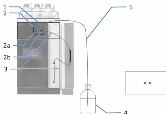
Figure 28: Measuring the backpressure of the flow cell, column, detector inlet capillary and waste line
