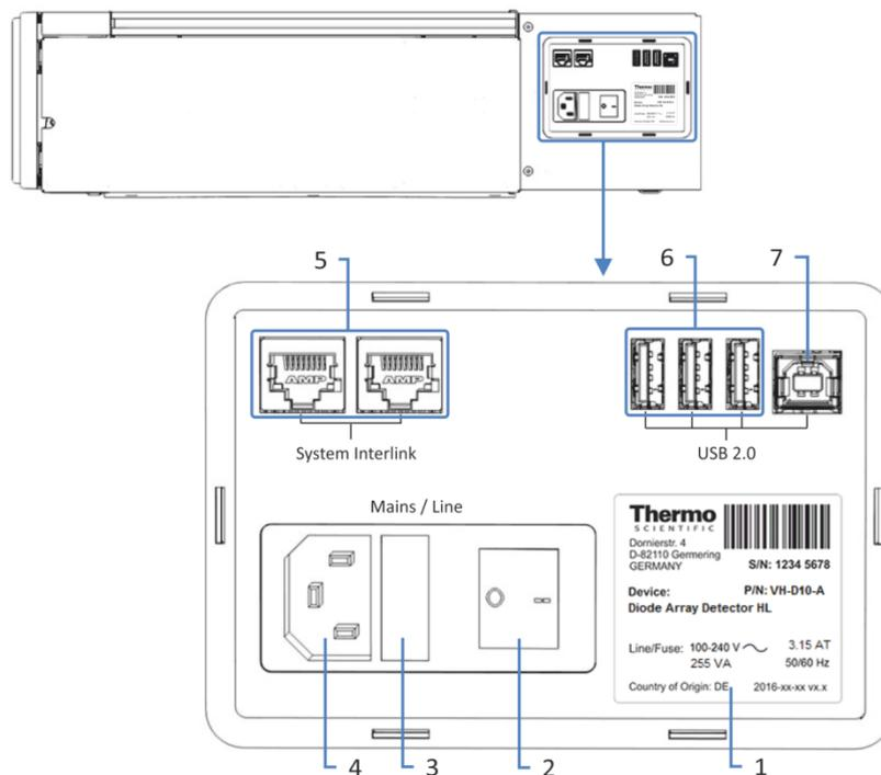
Figure 9: Electrical connectors on the right side of the device
