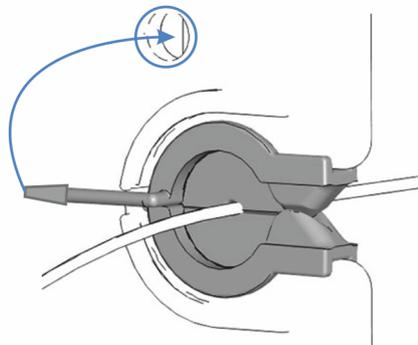
Figure 18: Securing the partition panel plug with slit
