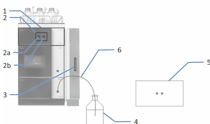
Figure 25: Measuring the backpressure of the waste line
