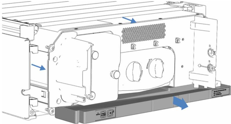
Figure 46: Pulling out the slide-in module (doors not shown)
