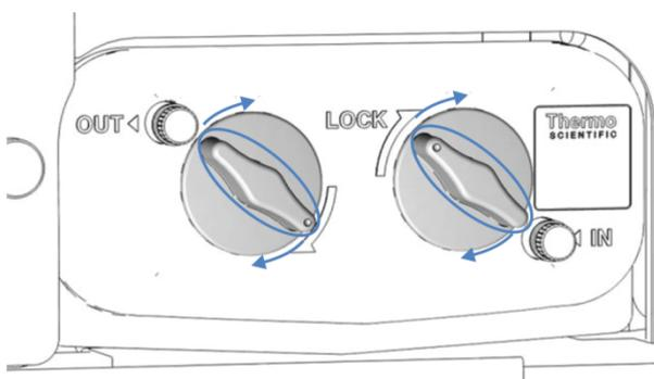
Figure 37: Closing the rotating locks
