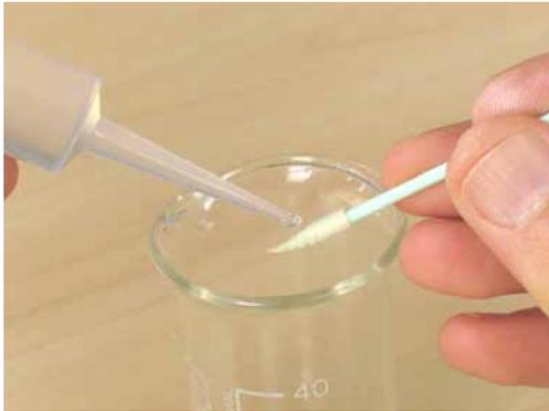
Fig. 23: Wet the swab with clean isopropyl alcohol
