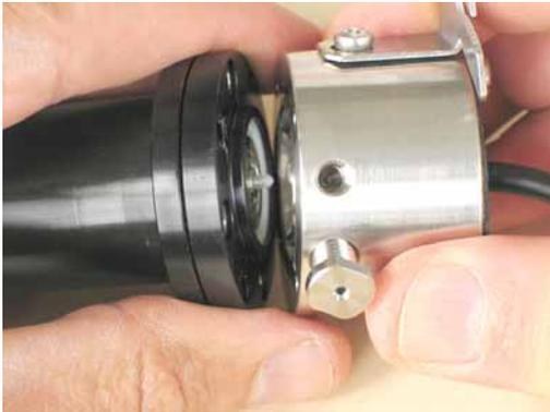
Fig. 34: Reassemble drive and fluidic block
