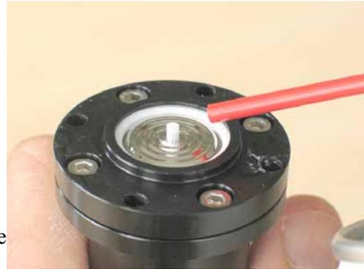
Fig. 30: Blow the liquid off the membrane
