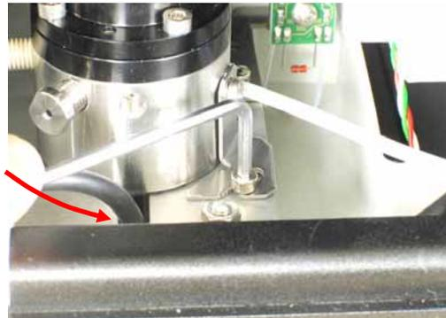
Fig. 14: Loosen the fixing screw
