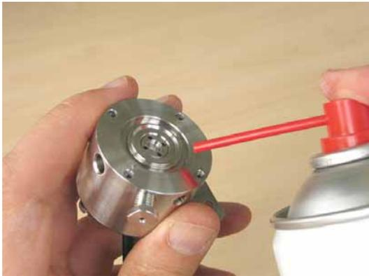
Fig. 27: Blow the liquid off the valve seat vicinity
