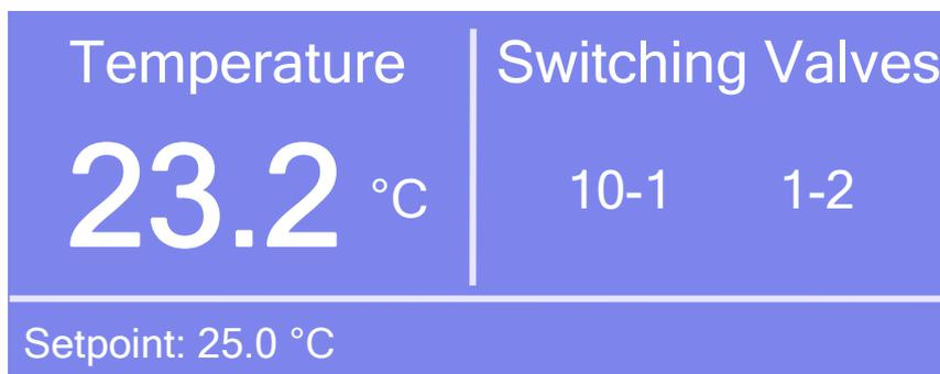
Fig. 28: Front panel display (here: for an FLM with two 2-position/10-port switching valves)
