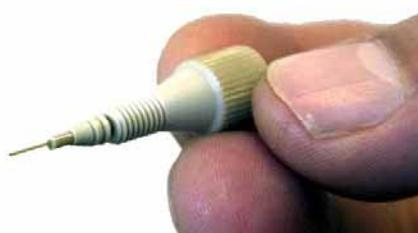
*Fig. 7: Inserting the column*
