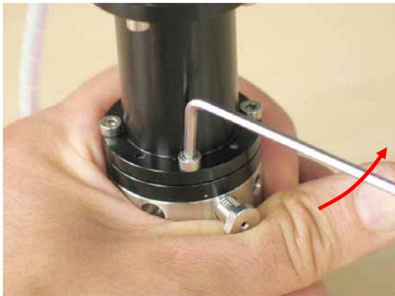
Fig. 20: Remove the screws on the FCV fluidic block
