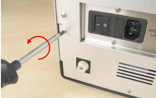
Fig. 7: Loosen the screw for the right side panel
