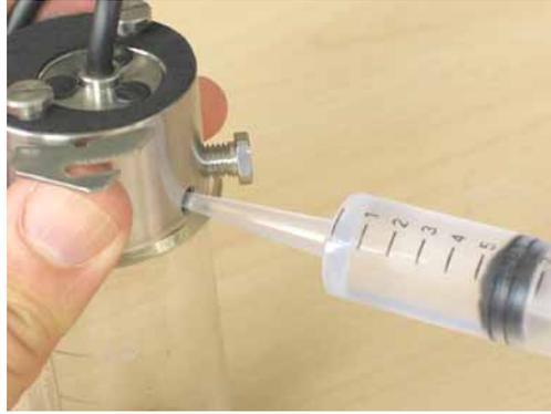
Fig. 22: Remove solvent from the fluidic block
