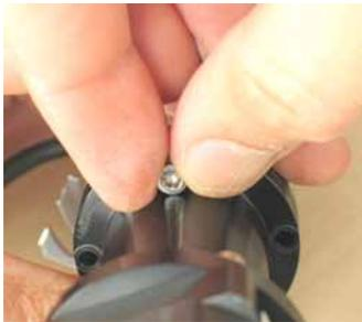
Fig. 36: Replace the screws
