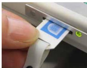
Fig. 38: Inserting a memory chip card in a memory card slot
