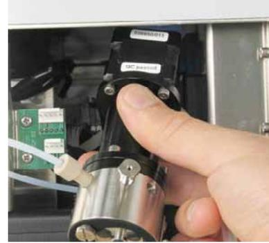
Fig. 17: Remove the FCV
