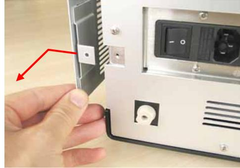
Fig. 8: Remove the side panel
