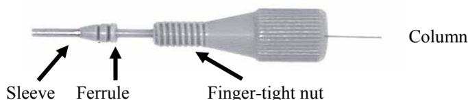
*Fig. 3: Fitting connection*
