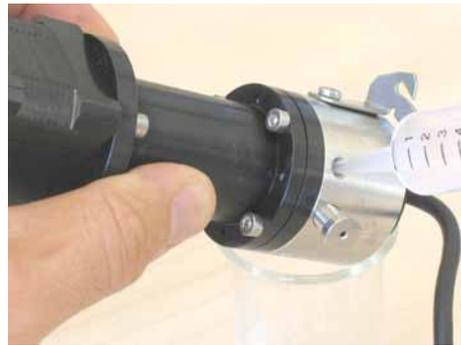
Fig. 19: Remove the solvent
