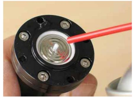
Fig. 33: Blow liquid off
